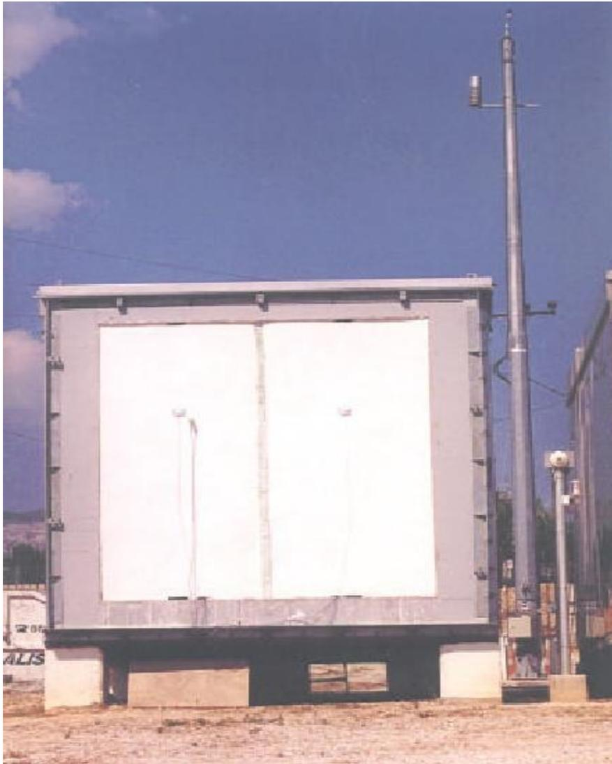
**Figure 21<sup>[VI]</sup> – Positioning of the wall component in the test cell – view of the meteorological mast**
