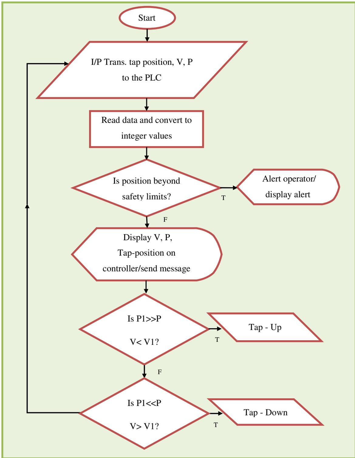
Figure 19: Voltage control algorithm
