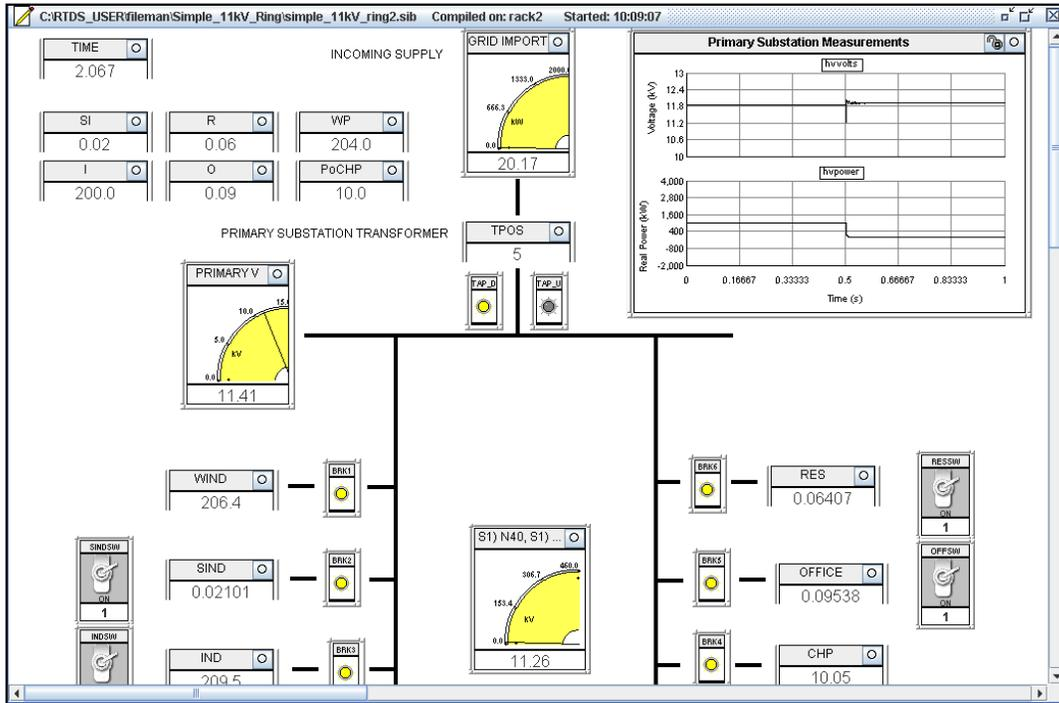
**Figure 29: Tap - down operation snapshot**
