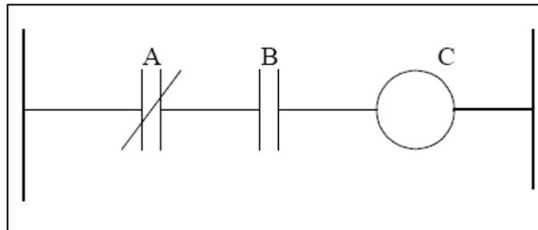
**Figure 14: Simple relay controller**
