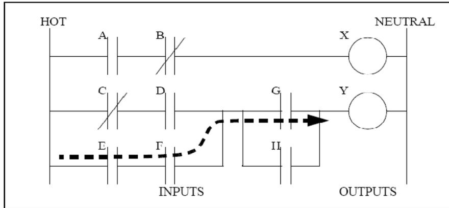
**Figure 15: Simple ladder logic diagram**
