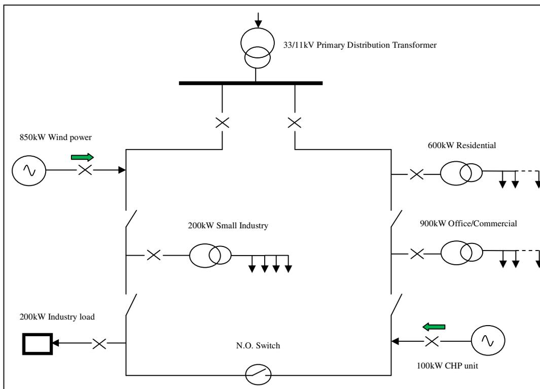
Figure 5: Example ring type distribution network
