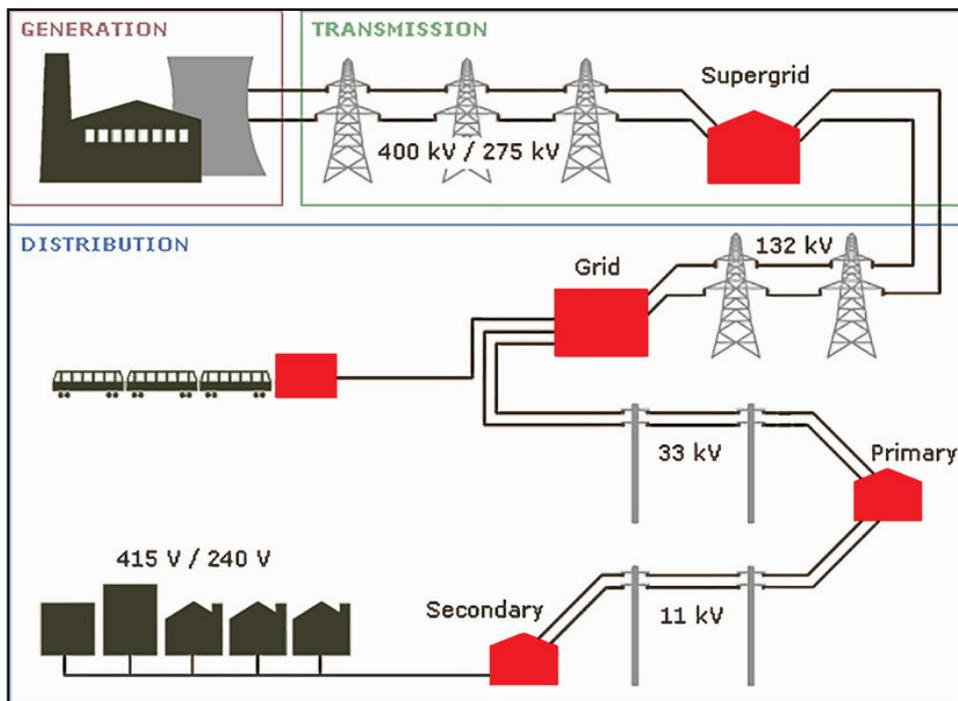
Figure 1: UK Electricity System Configuration [2]
