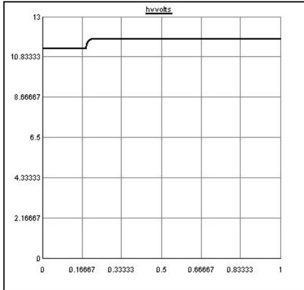
**Figure 27: Tap - up operation resulting in voltage rise**
