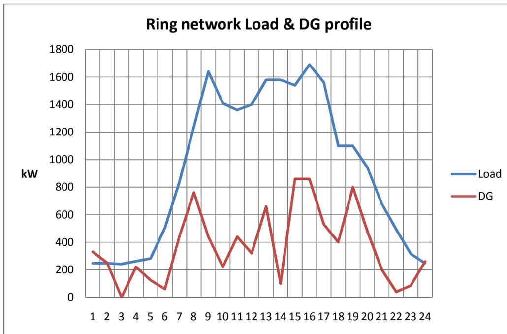
Figure 12: Total Load and DG profile for a typical day
