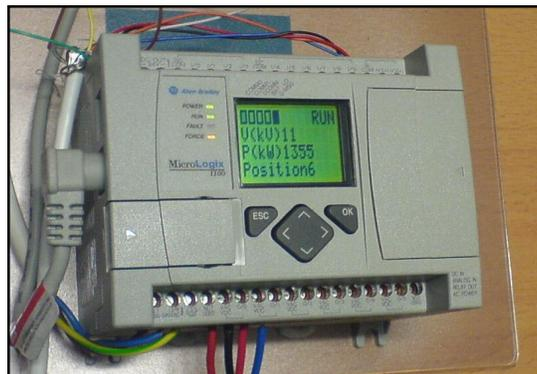
**Figure 30: LCD Display on the PLC**
