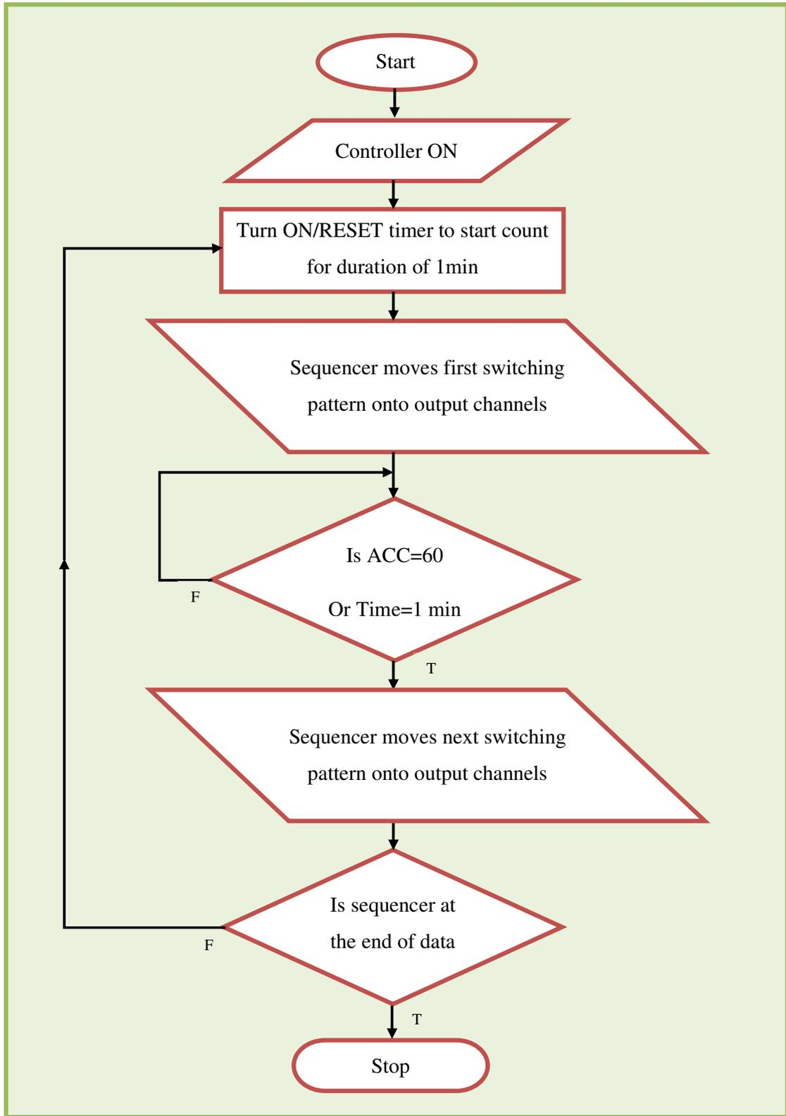
Figure 18: Load switching algorithm
