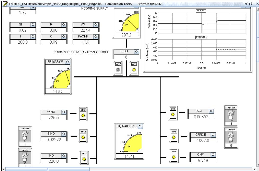
**Figure 28: Tap - up operation snapshot**
