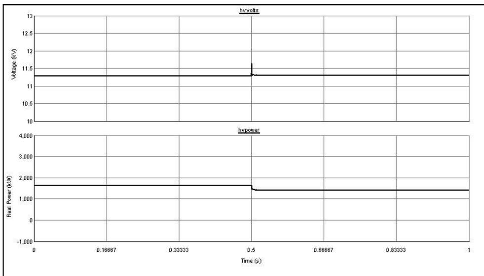
**Figure 25: Small industry load switched off**
