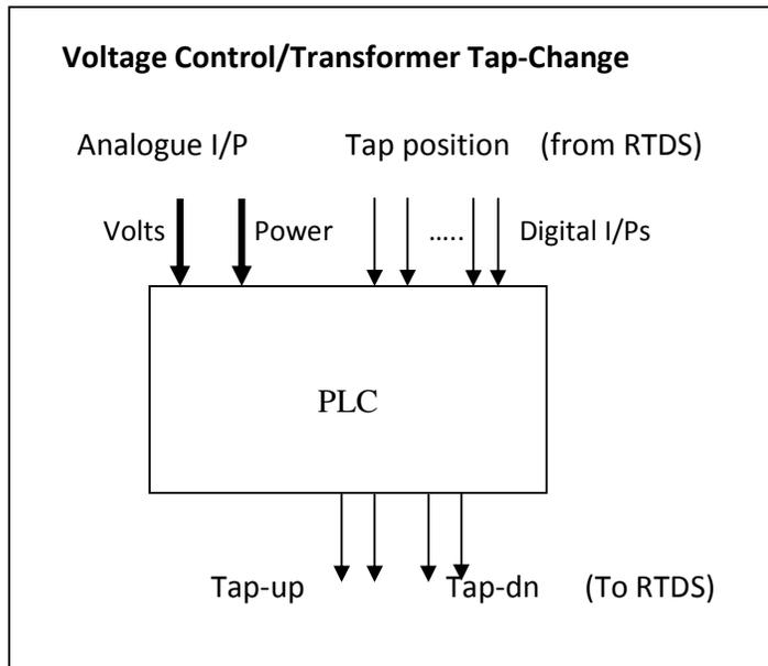
**Figure 20: Schematics for controller wiring**
