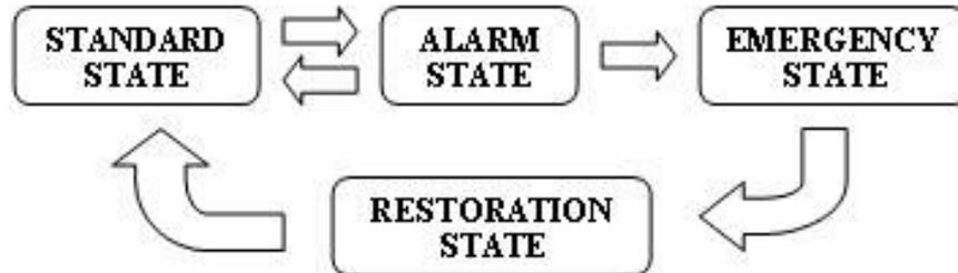
Figure 21. Power system operation states
