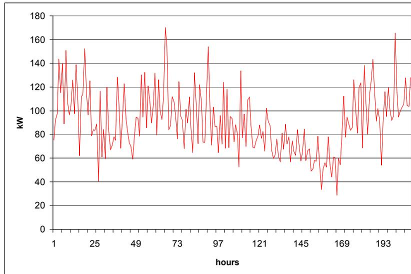
**Figure 56: Assumed curve of electricity consumption of the plan in full capacity**
