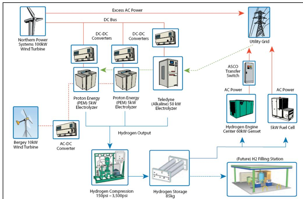
**Figure 19: Configuration of Xcel-NREL Wind2H2 Project [28]**
