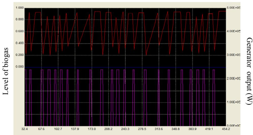
**Figure 44: Engine operation and biogas storage level**
