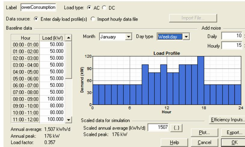
**Figure 42: Load profile generator in Homer**
