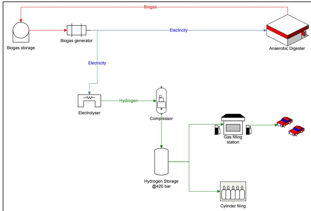
**Figure 37: Schematic diagram of the H2 SEED Project**
