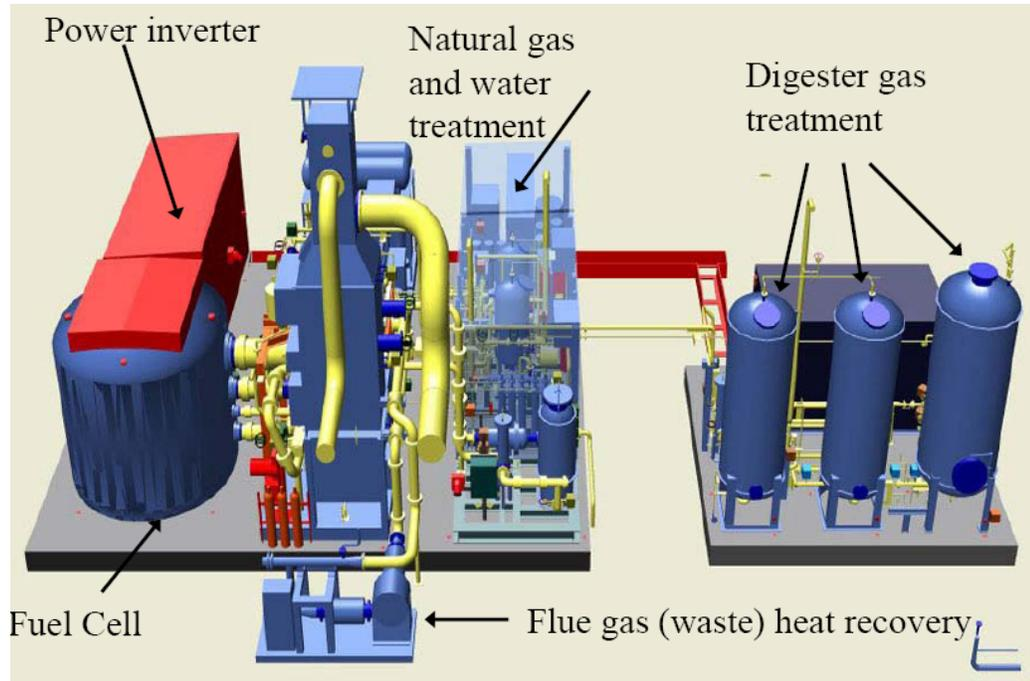
Figure 29: 3D model of 1MW biogas-powered fuel cell installation [37]
