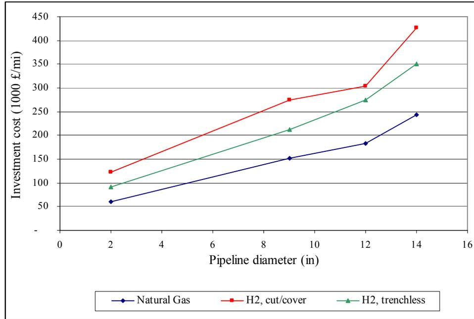
**Figure 12: Comparison between cost of hydrogen and natural gas pipelines [19]**
