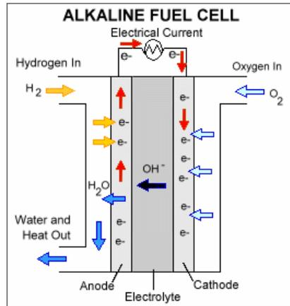
**Figure 6:** Schematic diagram of an alkaline fuel cell [3]
