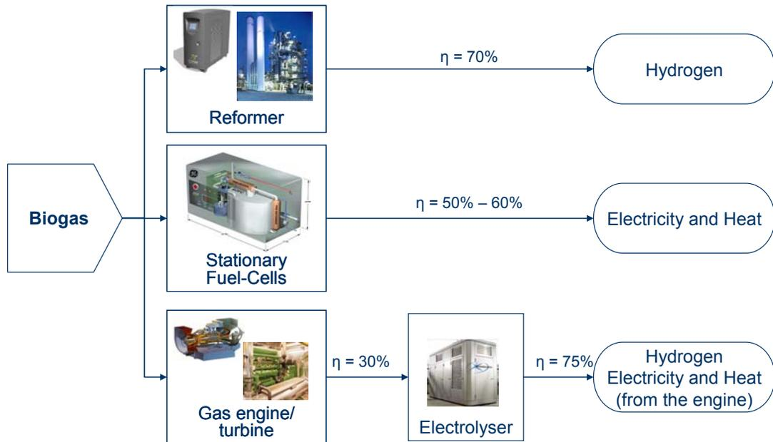
**Figure 28: Technological pathways with biogas and hydrogen technologies**
