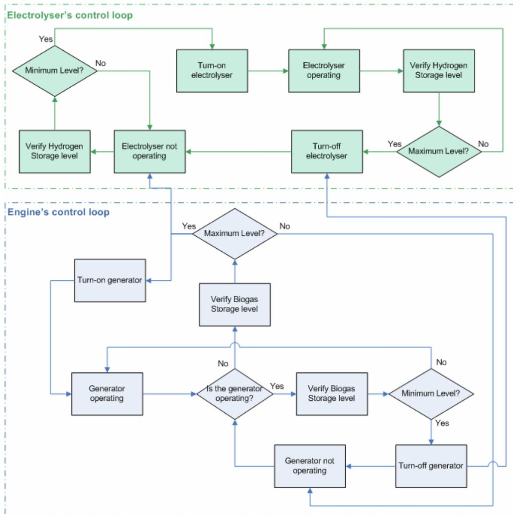
Figure 38: Logic diagram for the H2 SEED project
