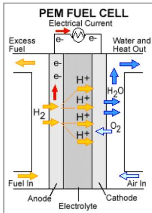
**Figure 4: Schematic diagram of a PEM Fuel Cell [3]**
