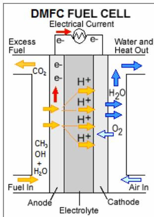
**Figure 5: Schematic diagram of a DMFC**
