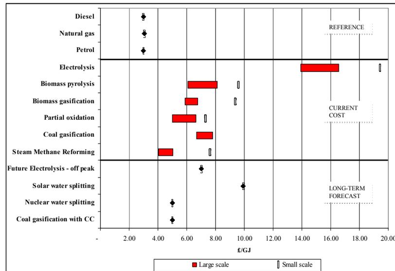
**Figure 10: Cost of hydrogen from different technologies, compared to traditional fossil fuels. Values in pounds (£) per GJ of annual capacity [13-14-5-15-16]**
