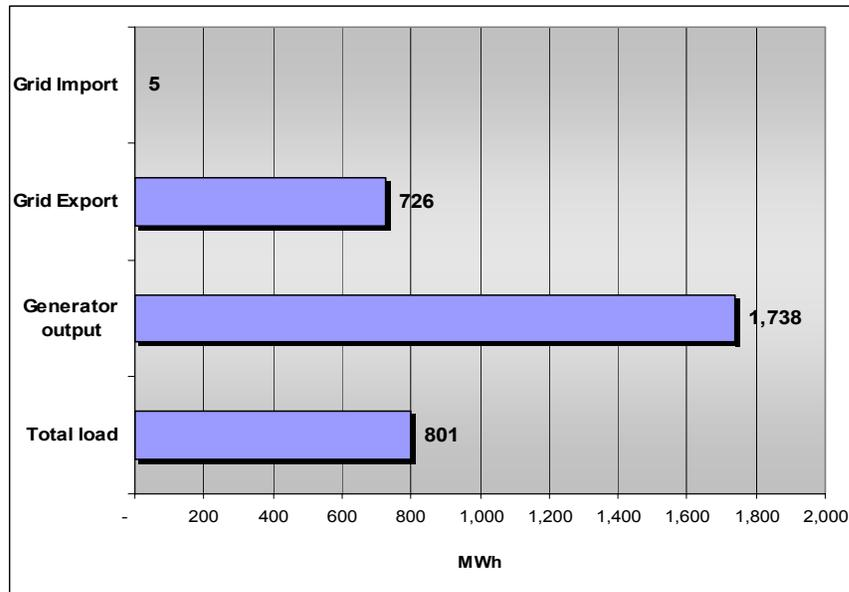
**Figure 58: Results for plant operating in full capacity**
