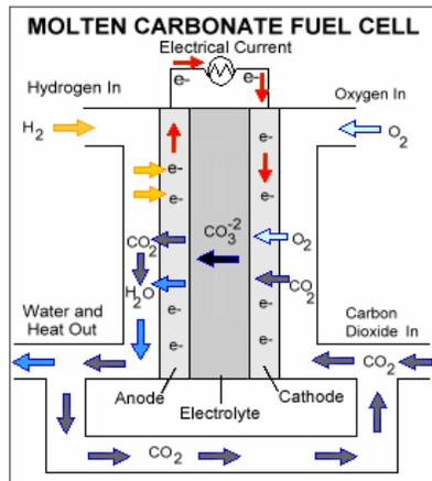
**Figure 8: Schematic diagram of a molten carbonate fuel cell [3]**
