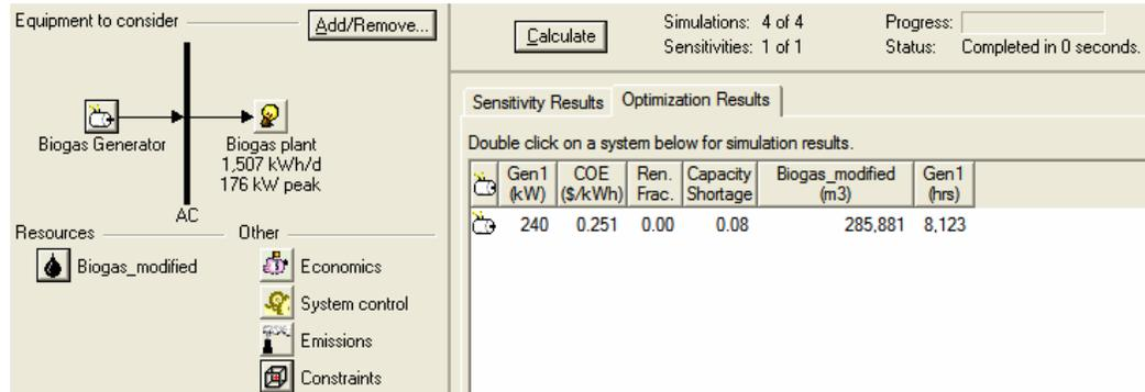
**Figure 39: Simplified energy balance in Homer**
