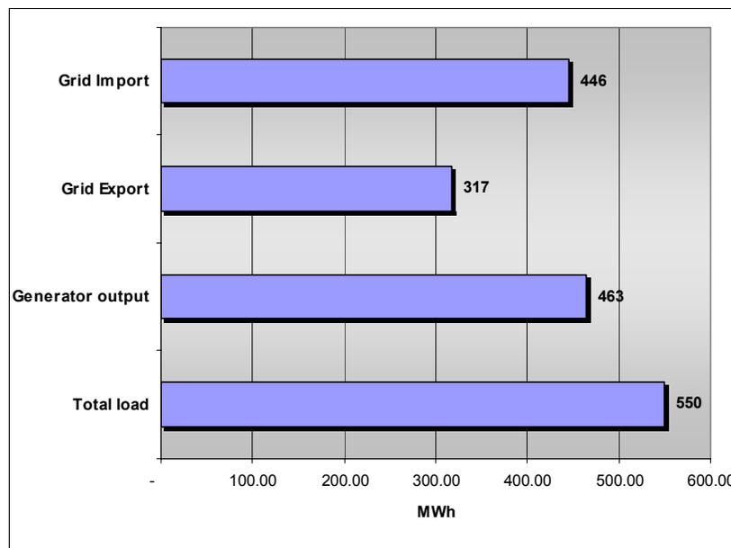
**Figure 49: Results for modified reference case, with electrolyser operating in idling power**
