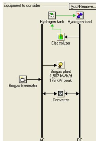
**Figure 41: Components considered in Homer model**
