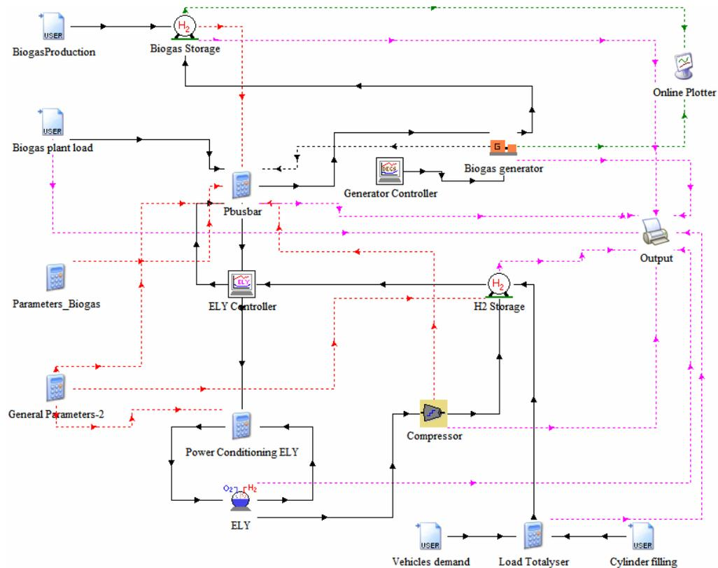
**Figure 43: TRNSYS model of the H2 SEED project**
