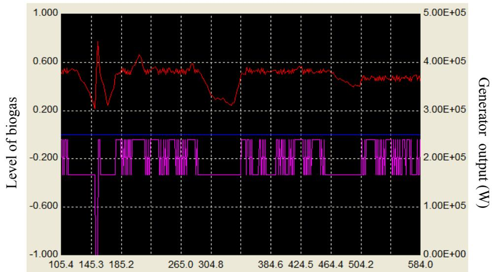
**Figure 57: Biogas level and generator behaviour for plant operating in full capacity**
