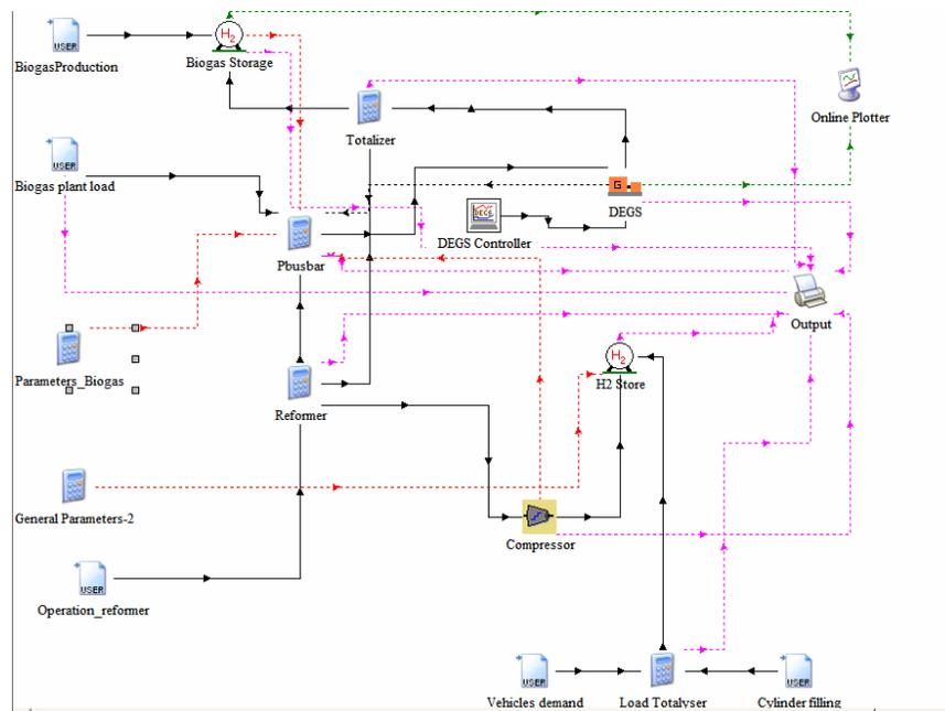
**Figure 62: TRNSYS model for the H2SEED project using an alternative configuration with a reformer**
