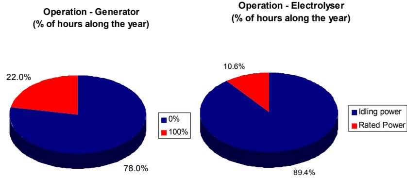
**Figure 50: Number of hours of generator and electrolyser operation in the modified reference case**
