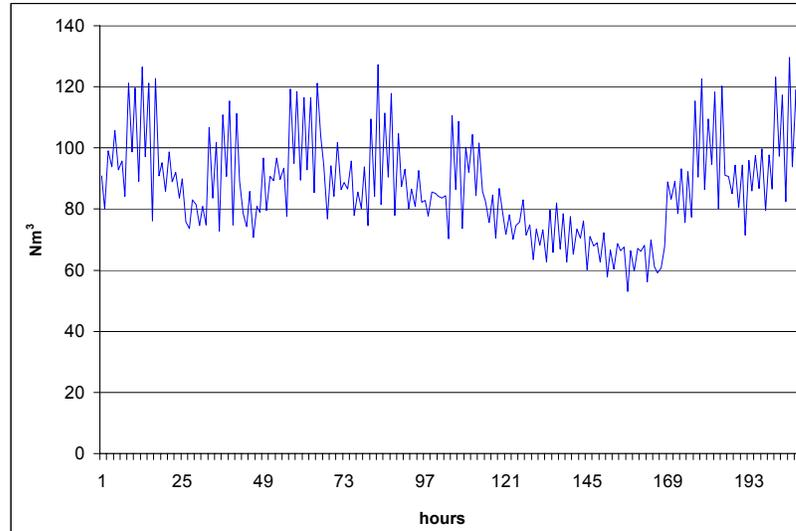
**Figure 55: Assumed curve of biogas production in full capacity**
