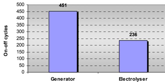
**Figure 52: Number of on-off cycles of generator and electrolyser in the modified reference case**
