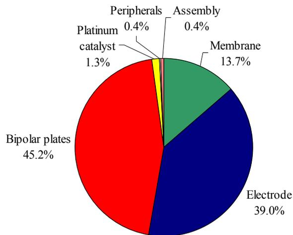
**Figure 13: Cost breakdown of current cost estimate of manually produced PEM fuel cells [5]**
