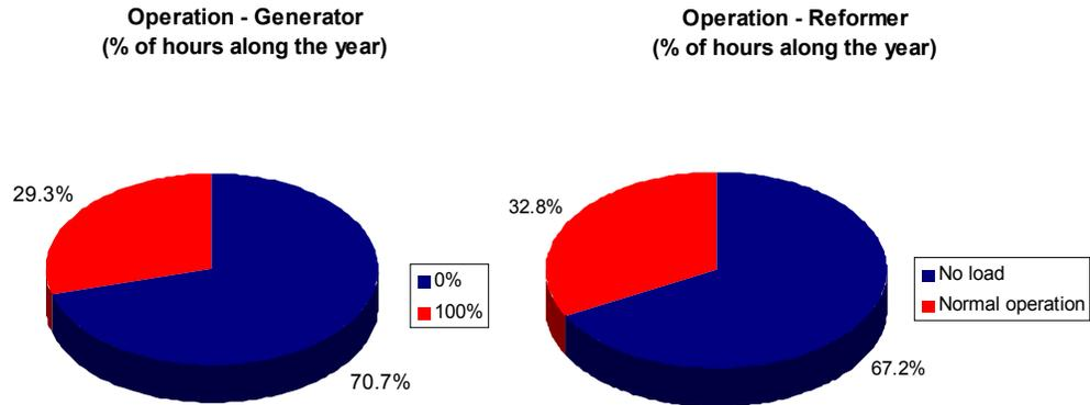
Figure 65: Performance of generator and reformer
