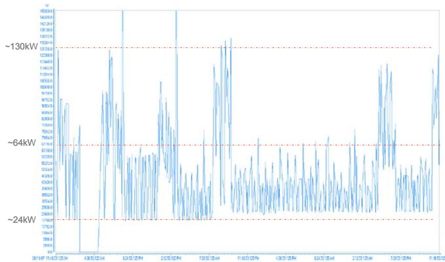
Figure 34: Weekly electricity consumption profile
