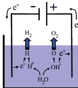
Figure 1: Schematic representation of an eletrolyser
