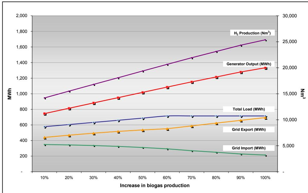
**Figure 54: Results for the constant increase in biogas production**
