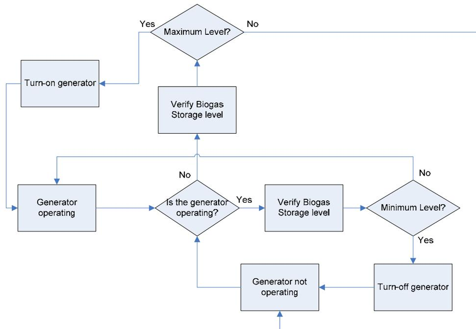
**Figure 36: Logic diagram for biogas engine operation**
