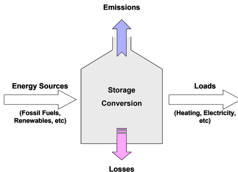
Figure 32: The “big boiler” energy system model [39]
