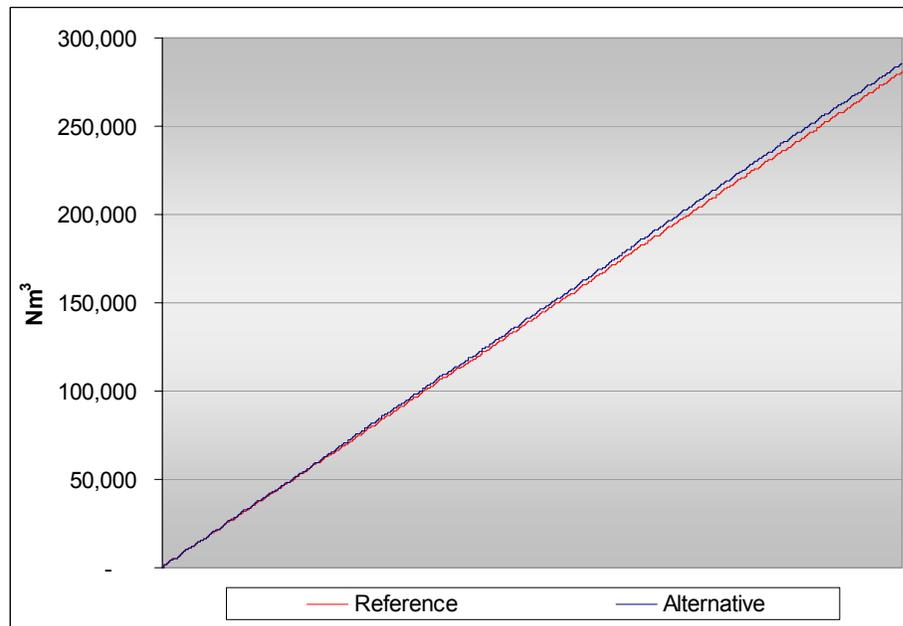
**Figure 71: Biogas consumption for reference and alternative cases**
