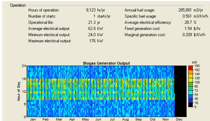
**Figure 40: Detailed results for a simplified energy balance in Homer**
