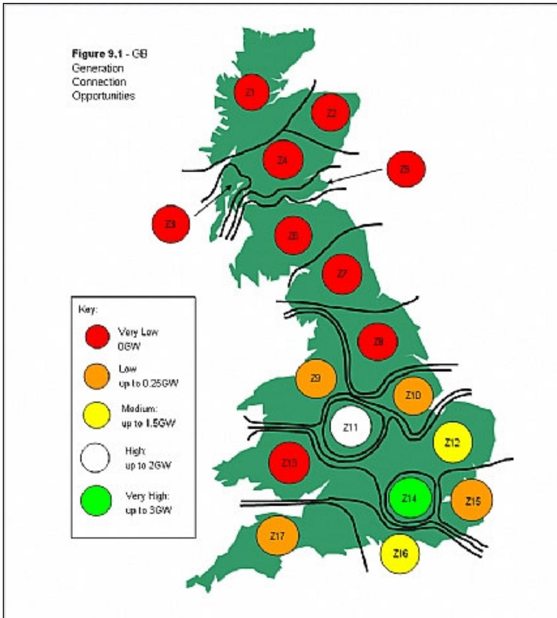
Figure 25: Capacity of the Transmission Network for Further Generation (National Grid, 2007)
