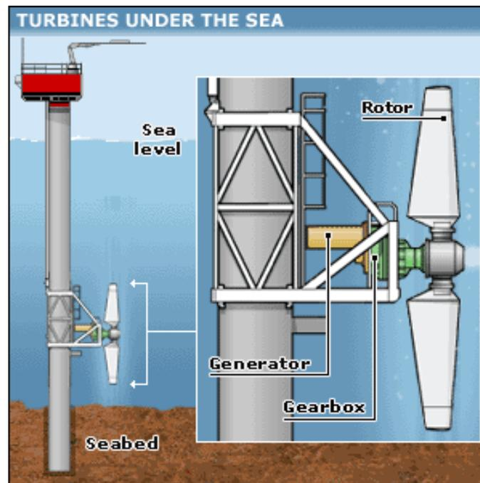
Figure 6: Seaflo Schematic Diagram (MCT, 2004)
