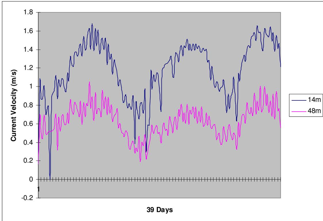
Graph 9: Variation of Tidal Current Velocity with Depth 3 (50m Seabed Depth)
