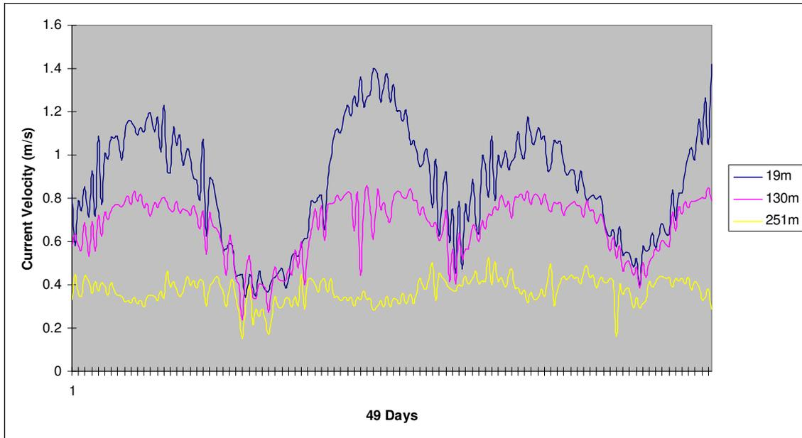
Graph 7: Variation of Tidal Current Velocity with Depth 1 (260m Seabed Depth)
