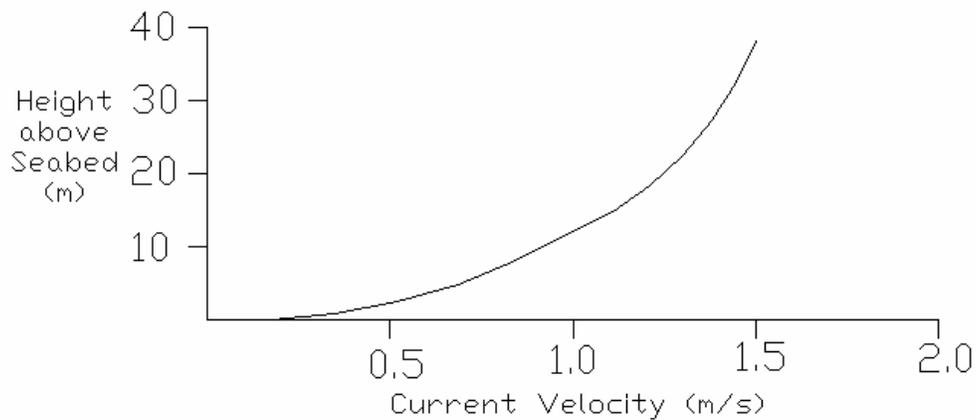
Graph 10: Variation of Tidal Current Velocity with Depth 4 (50m Seabed Depth)
