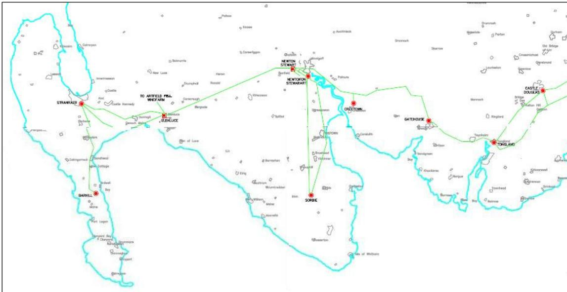
Figure 21: Local 33kV Distribution Grid & Substations (Scottish Power, 2006)
