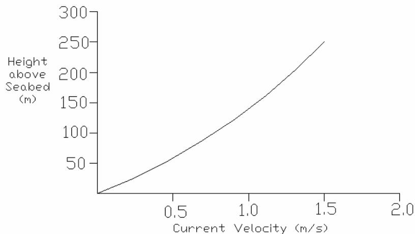
Graph 8: Variation of Current Velocity with Depth 2 (260m Seabed Depth)
