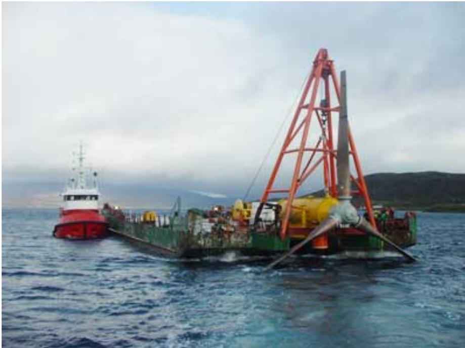
*Figure 4: Hammerfest Strøm AS tidal turbine being deployed (Hammerfest Strøm AS, 2007)*
