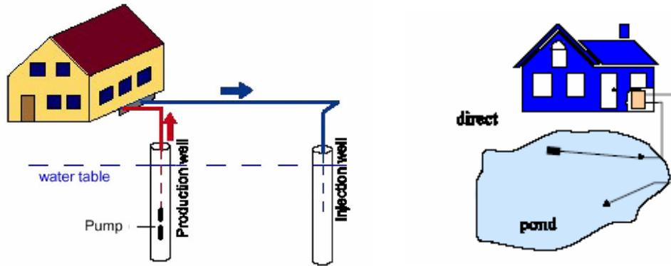
Fig 20 a & b. Open Loop System Using Wells [6] and a Pond [27]
