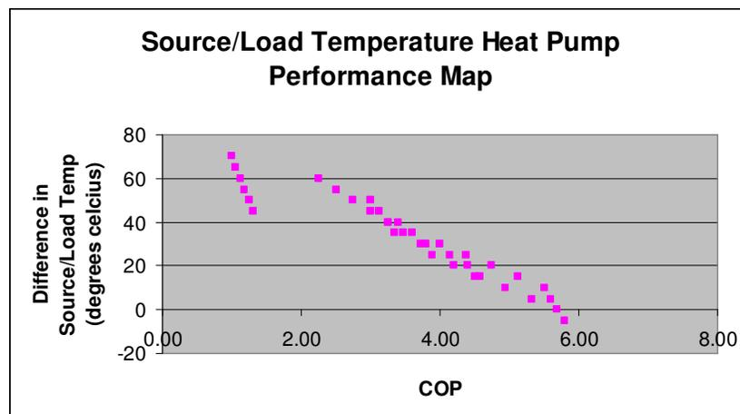
**Fig 66. Graphical Representation of Viessmann Vitocal 350 Performance Map [adapted from 82]**
