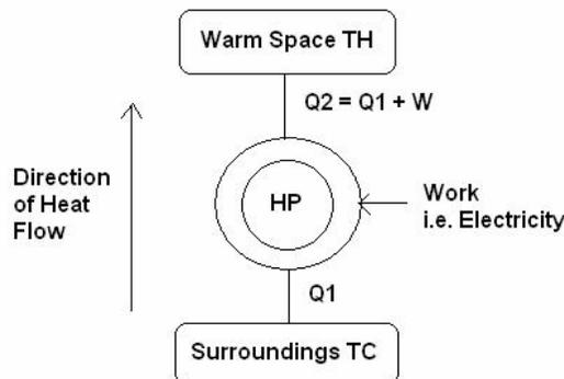
**Fig 1. Basic Premise of a Heat Pump (reproduced from [1])**
