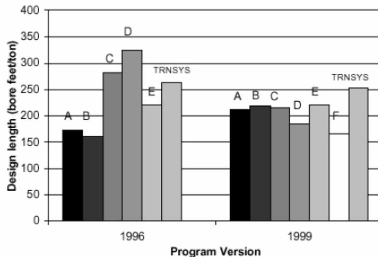
**Fig 54. One Year Comparison of Design Lengths for a Cooling Based Residential Heat Pump System (max entering temperature of 35°C) [70]**
