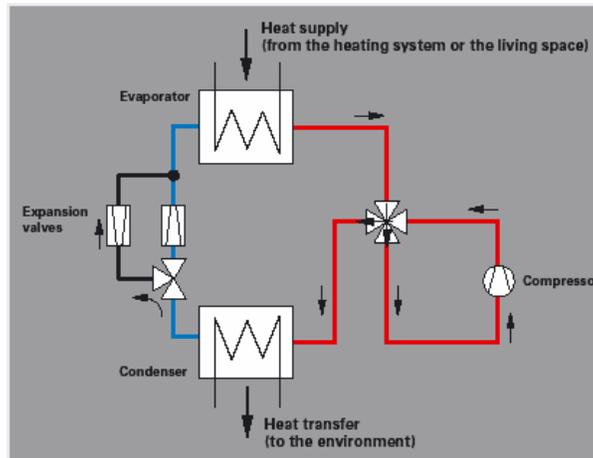
**Fig 12. Function Diagram of a Reversible Heat Pump in Cooling Mode [5].**
