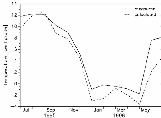
Fig 51. Measured and EED Calculated Brine Temperatures for UEG Plant, Wetzlar [71]
