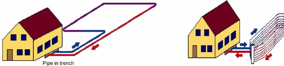
**Fig 22. Trench Collector Systems [6]**
