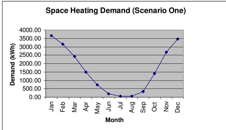
Fig 57. Heating Energy Use Profile of Detached House
