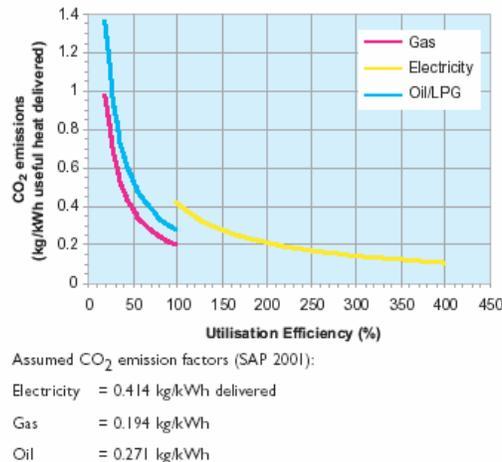
Fig 14. Carbon Dioxide Emissions for Different Fuel Use Efficiencies [11]
