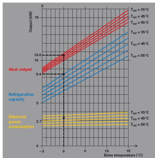
**Fig 5. Heat Pump Output Diagram for Different Source and Sink Temperatures [5] (this shows the relationship between heating/cooling/electrical input and temperature)**
