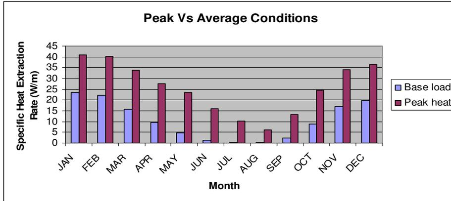
Fig 59. Peak Vs Base Specific Heat Extraction (EED Simulation Data)
