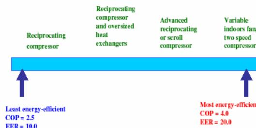
**Fig 8. Efficiency for Different Types of Compressor (for an open earth-energy system with source temperature of 10°C) [6]**
