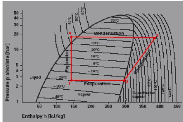
Fig 3. Vapour Compression Cycle on a Pressure/Enthalpy Diagram [5].
