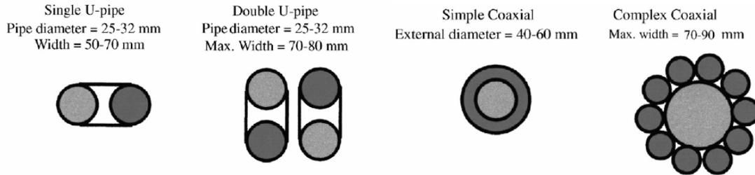
Fig 23a. Vertical Heat Exchanger Pipe Configurations [37]
