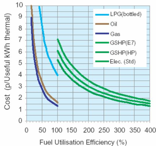
Figure 6: Domestic fuel costs\* versus fuel utilisation efficiency
