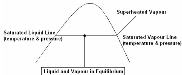
**Fig 4. Liquid/Vapour and Mixed Zones**
