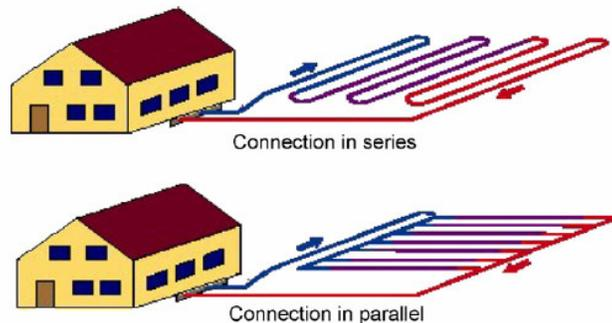
Fig 21. Series and Parallel Ground Loop Configurations [6]
