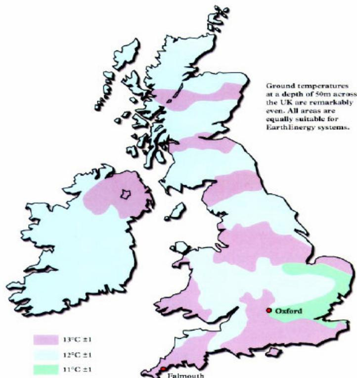
Fig 37. Ground Temperatures in the UK at a Depth of 50m [33]
