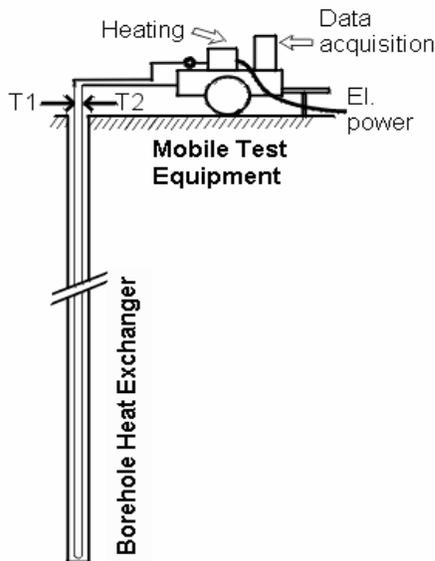
**Fig 47. Schematic of a Thermal Response Test [70]**
