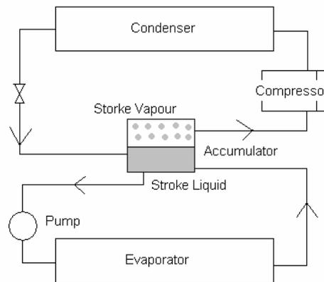
**Fig 9. Heat Pump Cycle with Accumulator (reproduced from [1])**
