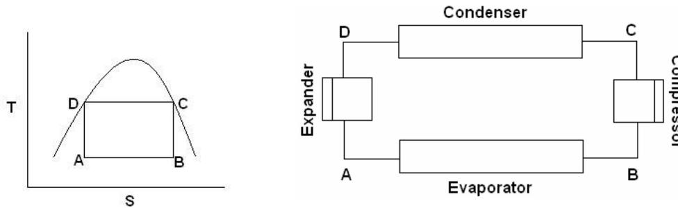
Fig 2a. & 2b. Carnot Cycle Explained (reproduced from [1])
