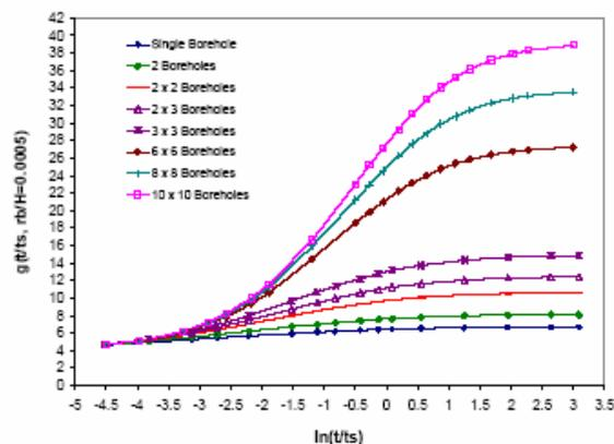
**Fig 49. G-functions for various Multiple Borehole Configurations compared to a Temperature Response Curve for a Single Borehole [77]**
