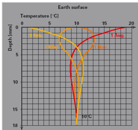
Fig 16. Example of a Typical Ground Temperature Profile [5]
