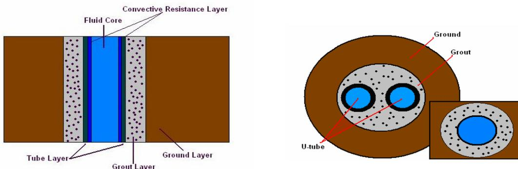
**Fig 48a. Heat Transfer Model Implications & Fig 48b. ‘Birds Eye View’ of Borehole (reproduced from [77]), to simplify further the u-tube can be modelled as a single cylinder with twice the area (see inset)**
