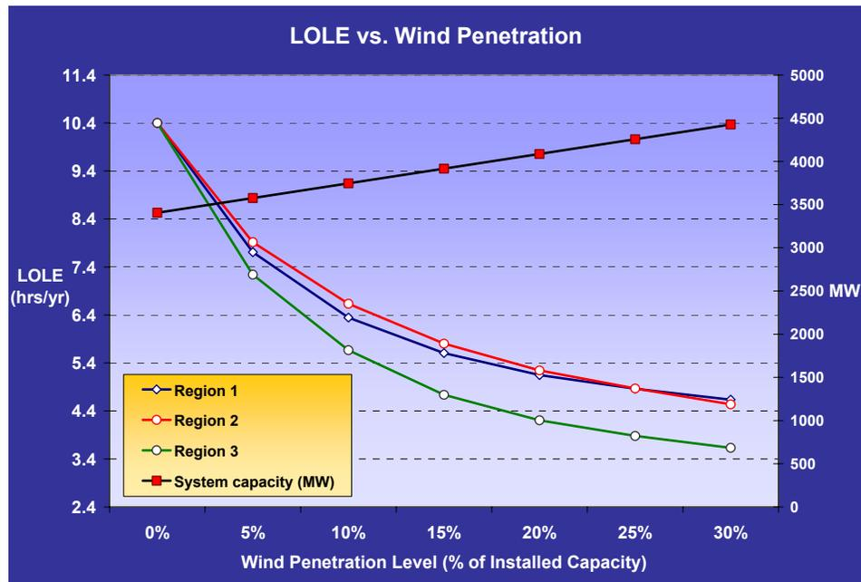
Figure 6-1: The effect of wind penetration on system reliability
