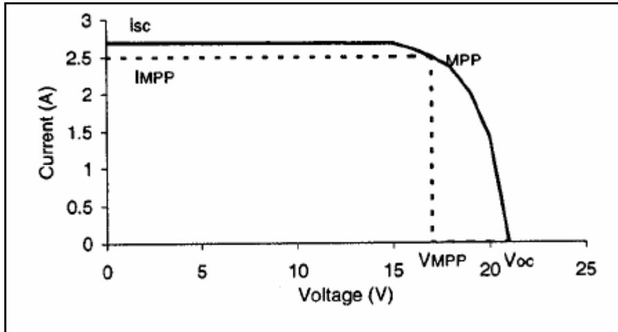
Figure 2-11: PV Cell Current-Voltage characteristics curve
