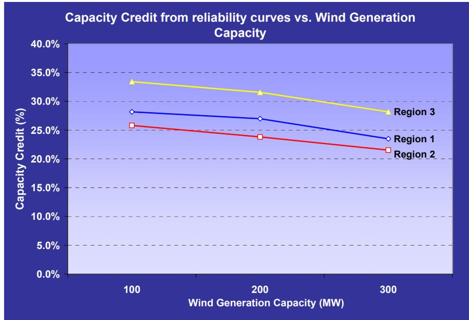
Figure 5-4: Capacity credit with different wind generation capacity
