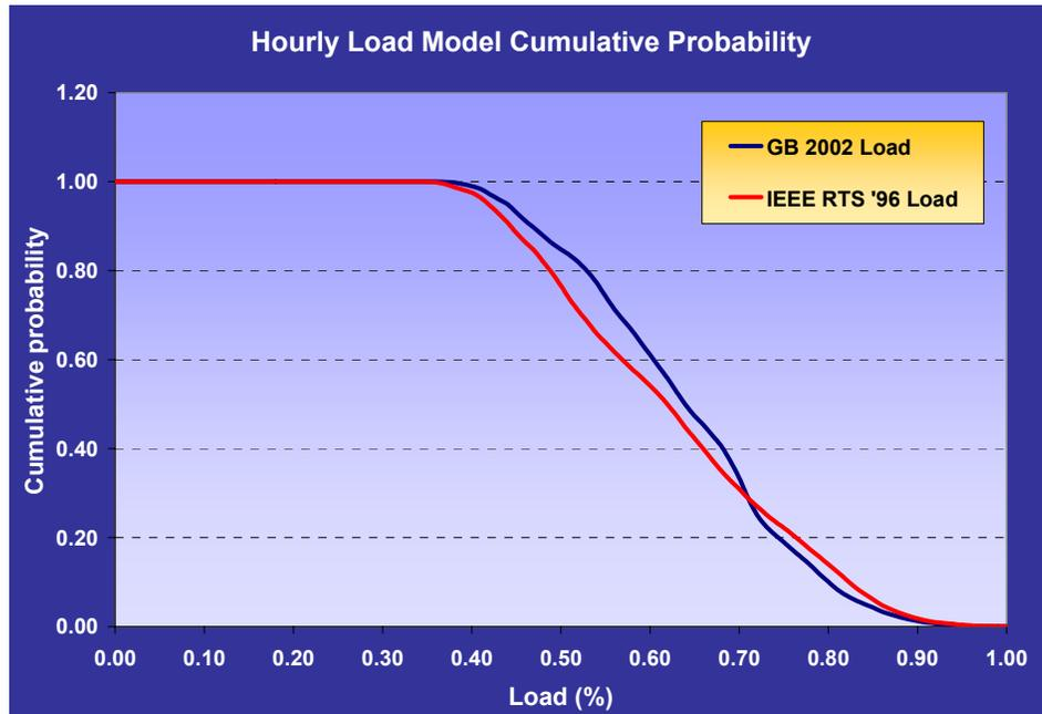
**Figure 6-9: Hourly load cumulative probability curve comparison**
