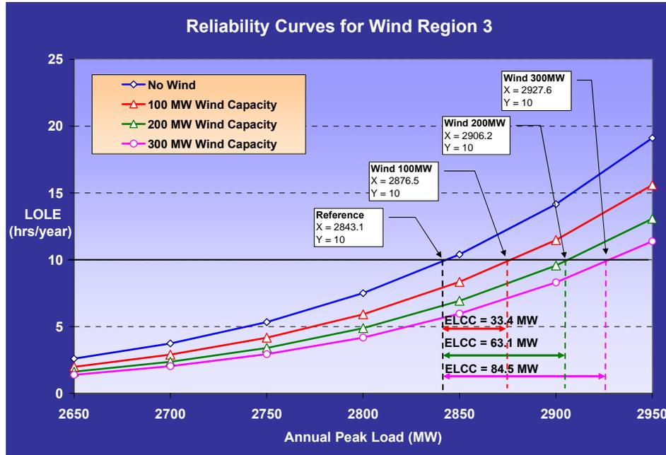
Figure 5-3: Wind Region 3 capacity credit evaluation using reliability curves
