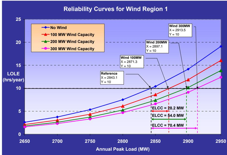
**Figure 5-1: Region 1 capacity credit evaluation using reliability curves**
