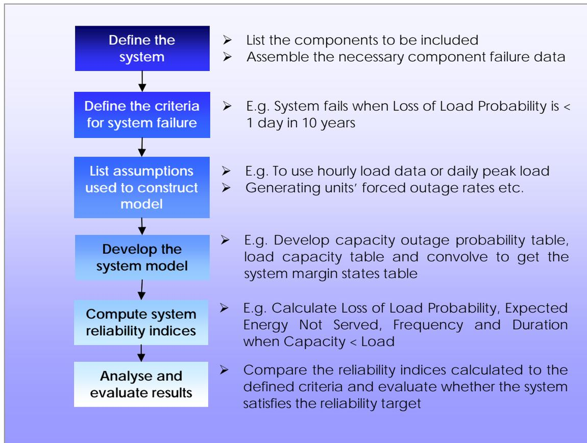
**Figure 2-2: Reliability models construction process**
