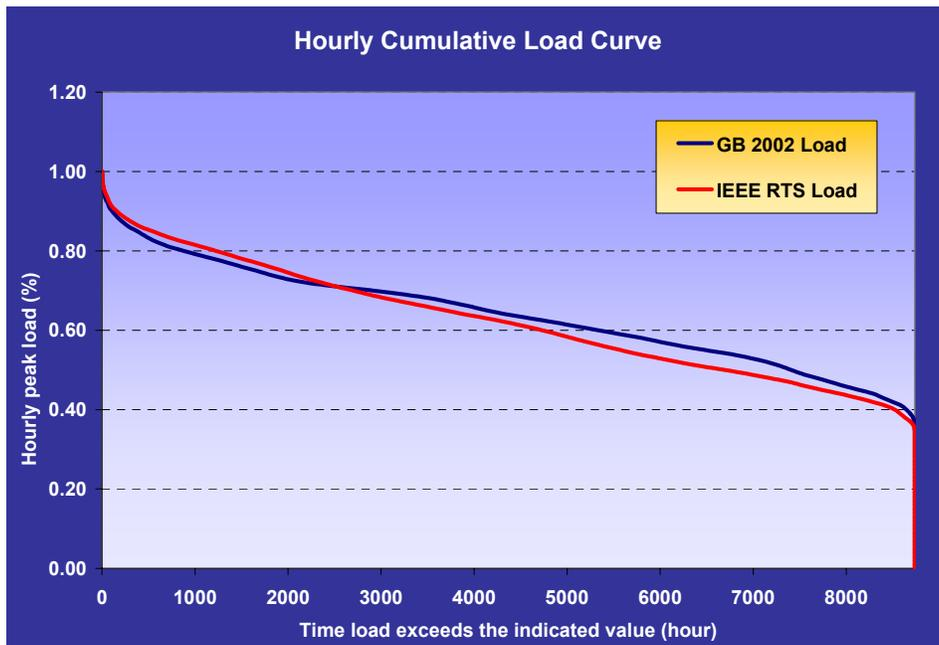
Figure 6-8: Hourly load duration curve comparison
