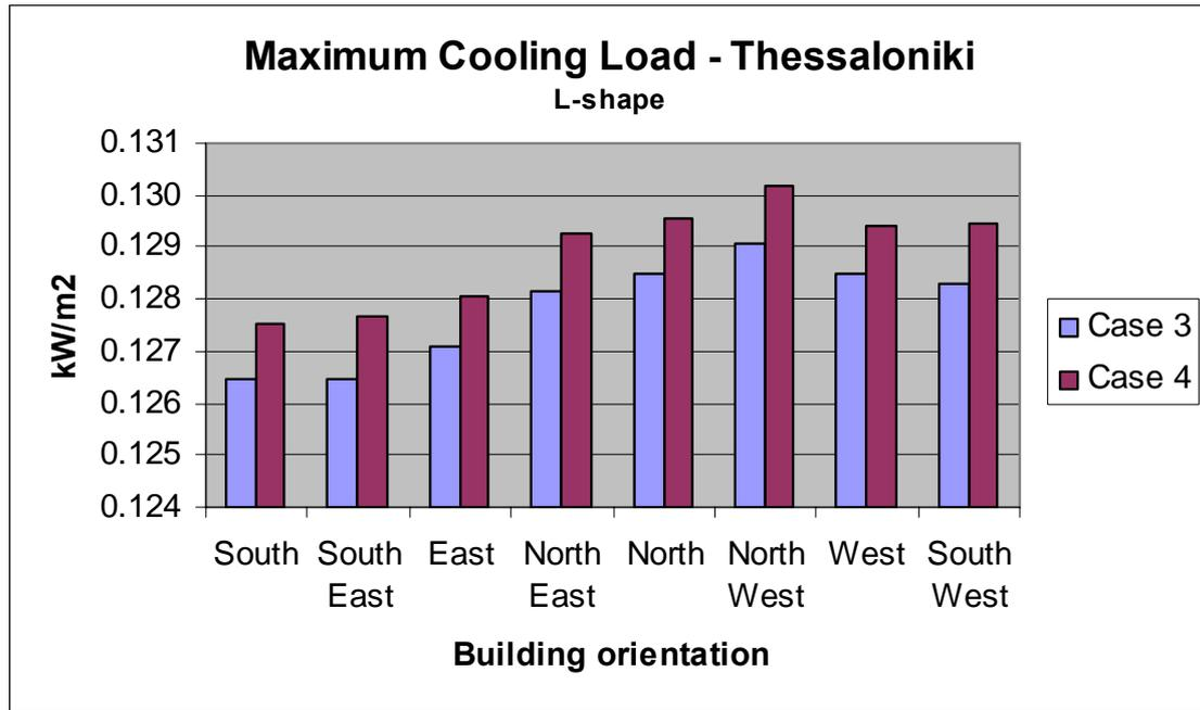
Figure 35: Maximum cooling load per m<sup>2</sup> - Thessaloniki
