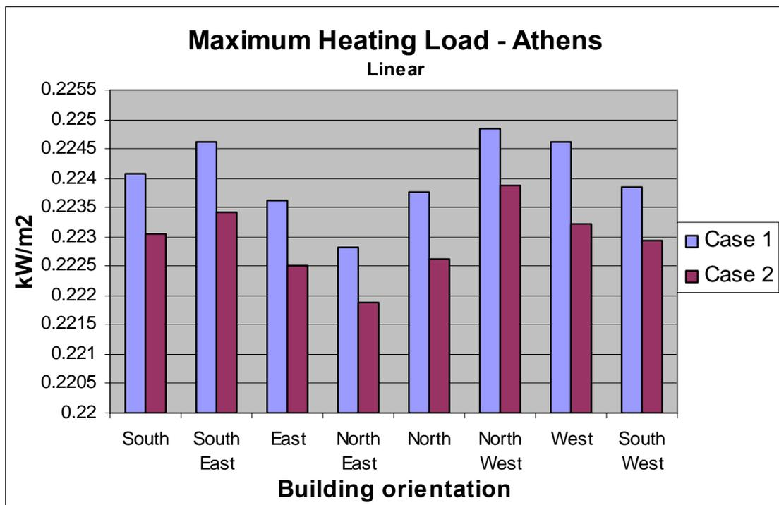
Figure 10: Maximum heating load per  $\text{m}^2$  - Athens
