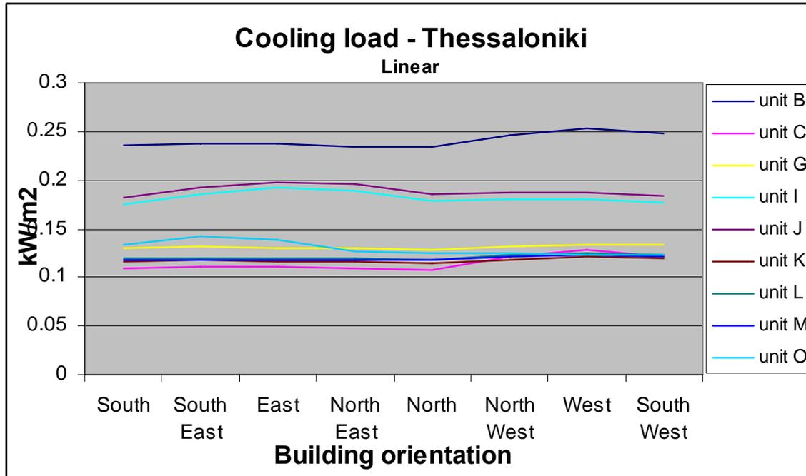
Figure 20: Maximum cooling load per zone per m<sup>2</sup> - Thessaloniki
