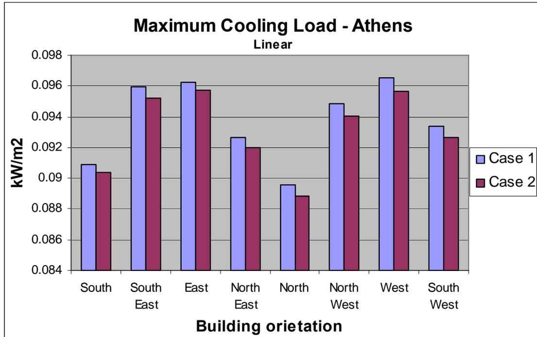
Figure 12: Maximum cooling load per m<sup>2</sup> - Athens
