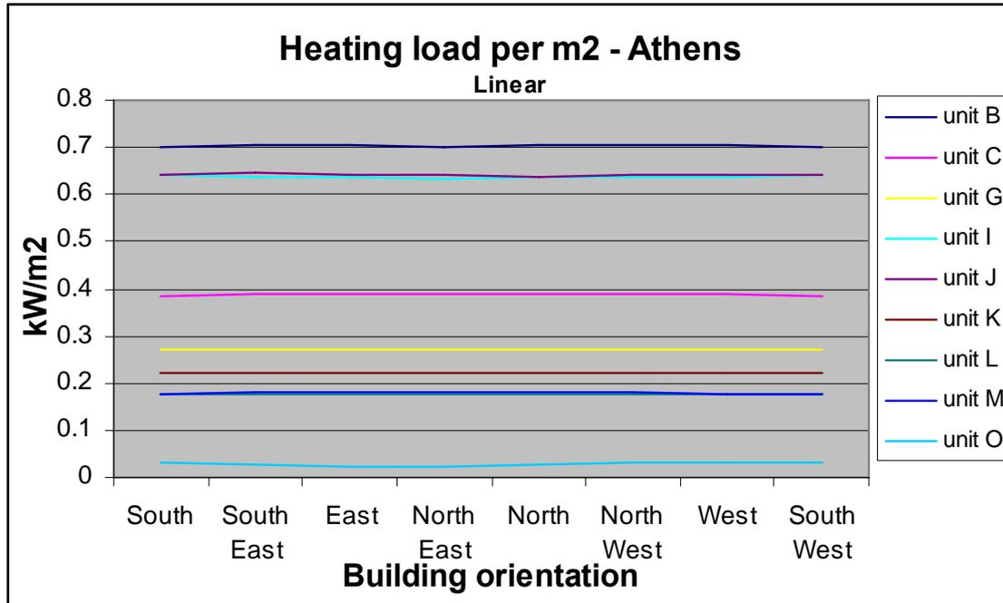
Figure 11: Maximum heating load per zone per m<sup>2</sup> – Athens
