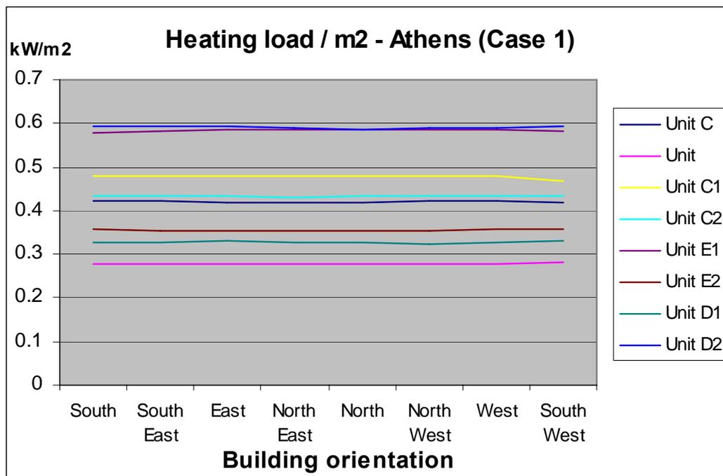
Figure 27: Maximum heating load per zone per  $\text{m}^2$  – Athens
