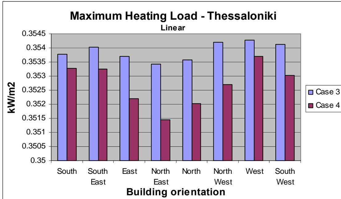
Figure 18: Maximum heating load per m<sup>2</sup> - Thessaloniki
