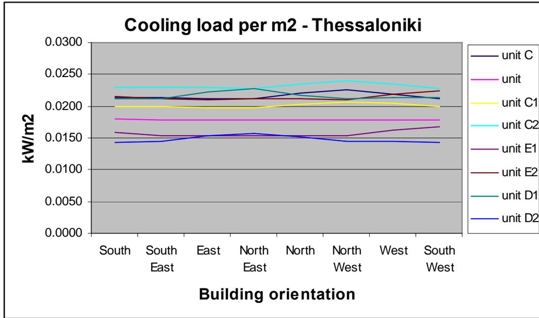
Figure 36: Maximum cooling load per zone per m<sup>2</sup> - Thessaloniki
