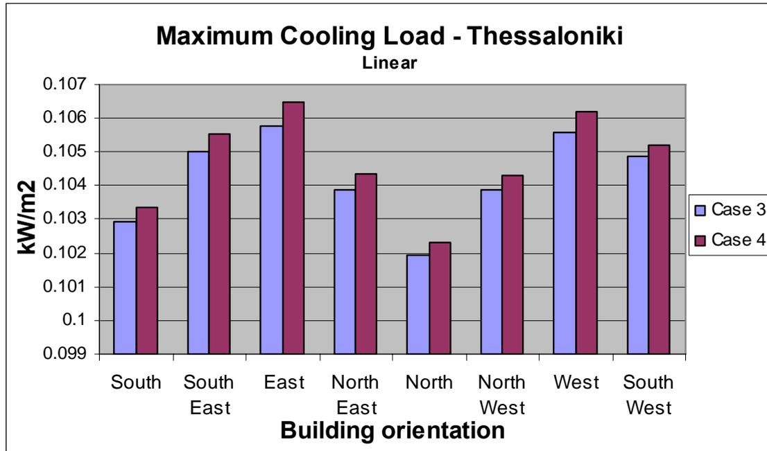
Figure 19: Maximum cooling load per m<sup>2</sup> - Thessaloniki
