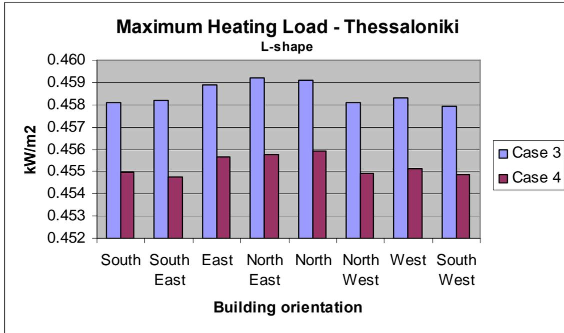
Figure 34: Maximum heating load per m<sup>2</sup> - Thessaloniki
