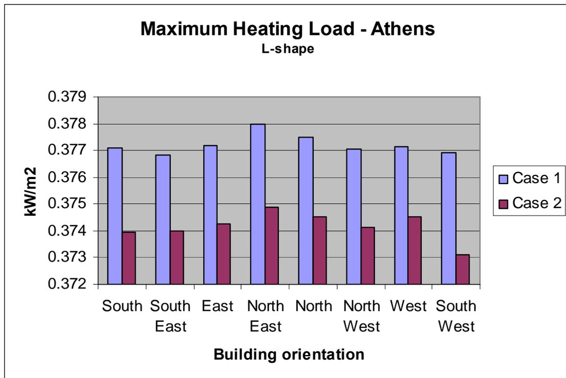
Figure 26: Maximum heating load per  $m^2$  - Athens
