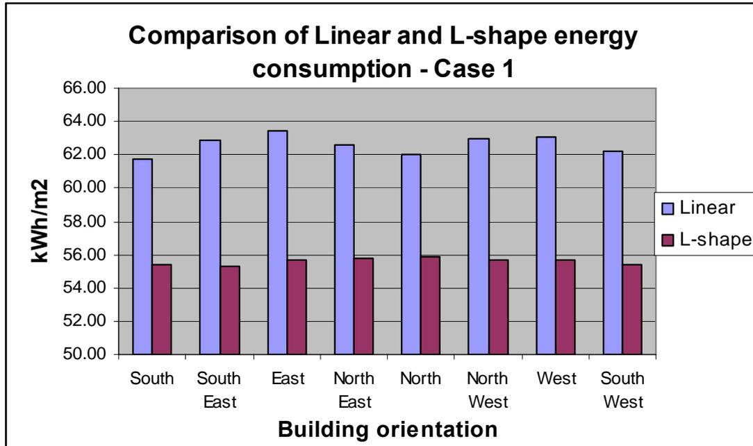
Figure 4: Energy consumption comparison – Athens – Case 1
