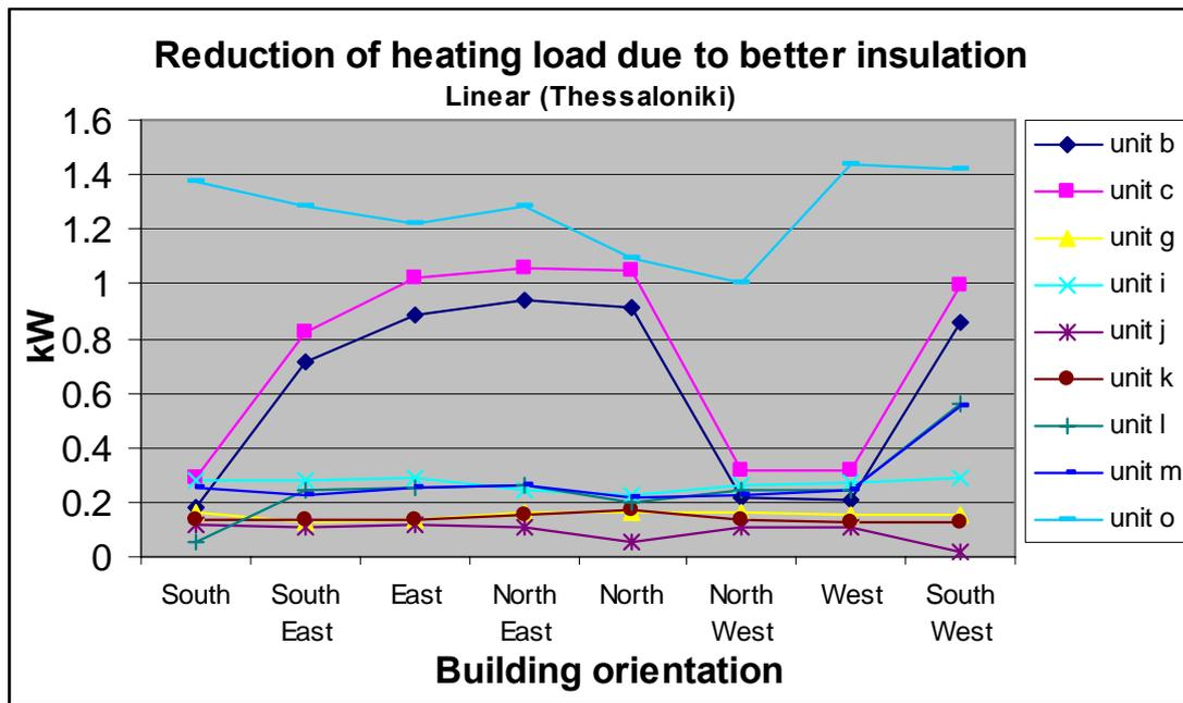
APPENDIX E4: Reduction of heating load due to better insulation
