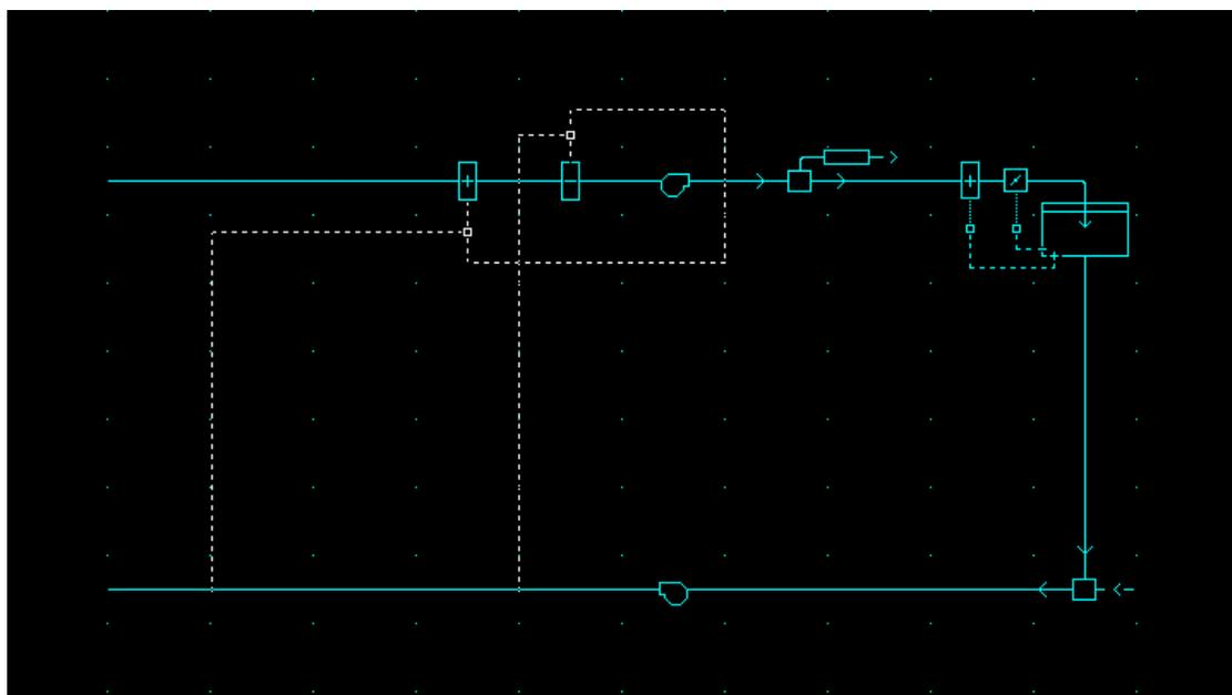
Figure 19: VAV TAS System Model Schematic
