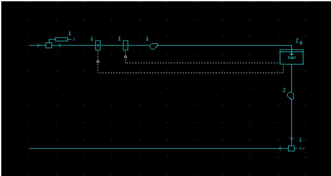
Figure 17: CAV TAS System Model Schematic
