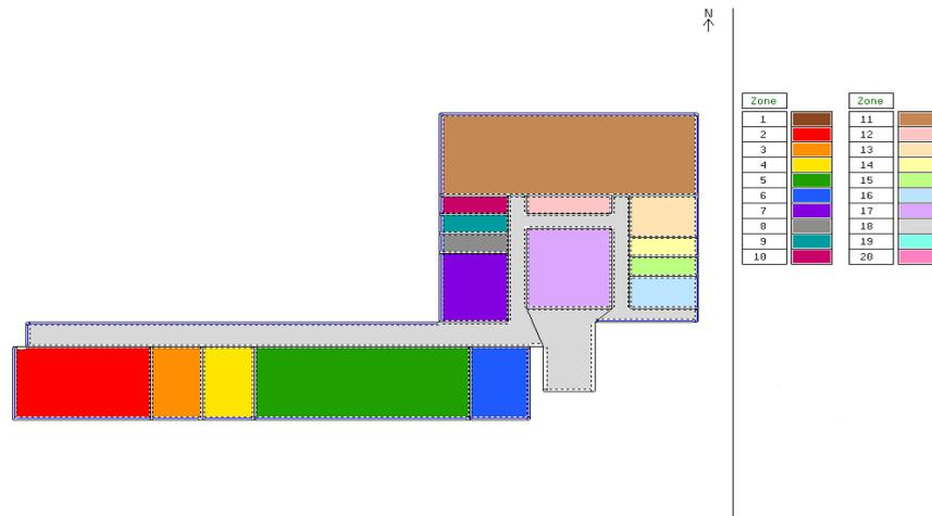
Figure 13 Thermal model zoning for a typical lower floor
