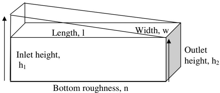
$n = 0.035$  (course sand), length = 10,000m, inlet height=53.5m, outlet height=51.5m, width = 1000m and the hydraulic radius is given by  $R = A/P$  where  $A$  = cross-sectional area of the flow and  $P$  is the wetted perimeter.
