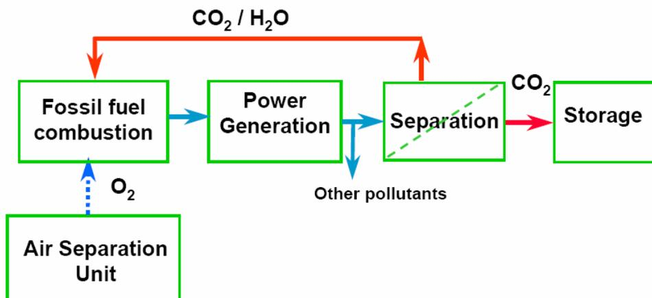
Figure 3.7: Oxy-fuel combustion
