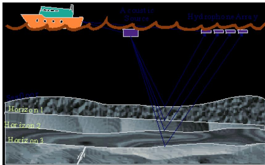
*Figure 1.6: Offshore seismic exploration*
