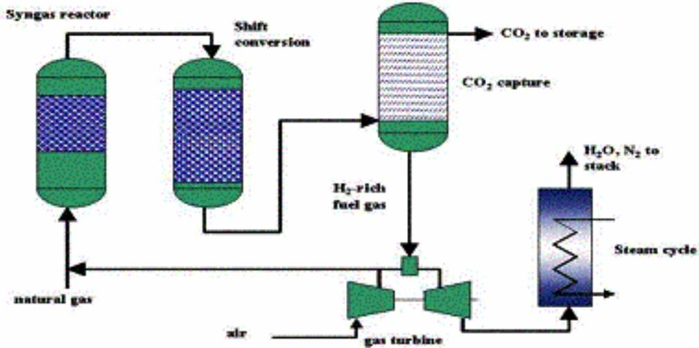
Figure 3.6: Pre-combustion capture for natural gas
