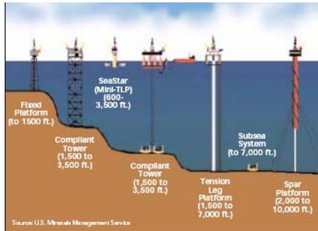
*Figure 1.9: Offshore drilling systems*
