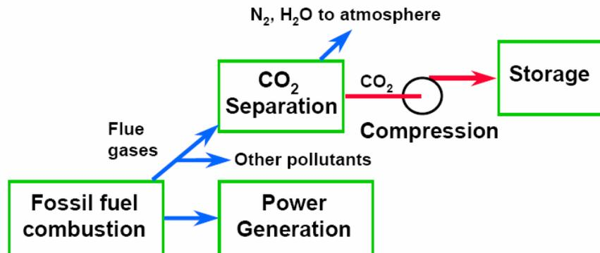
Figure 3.8: Post-combustion process
