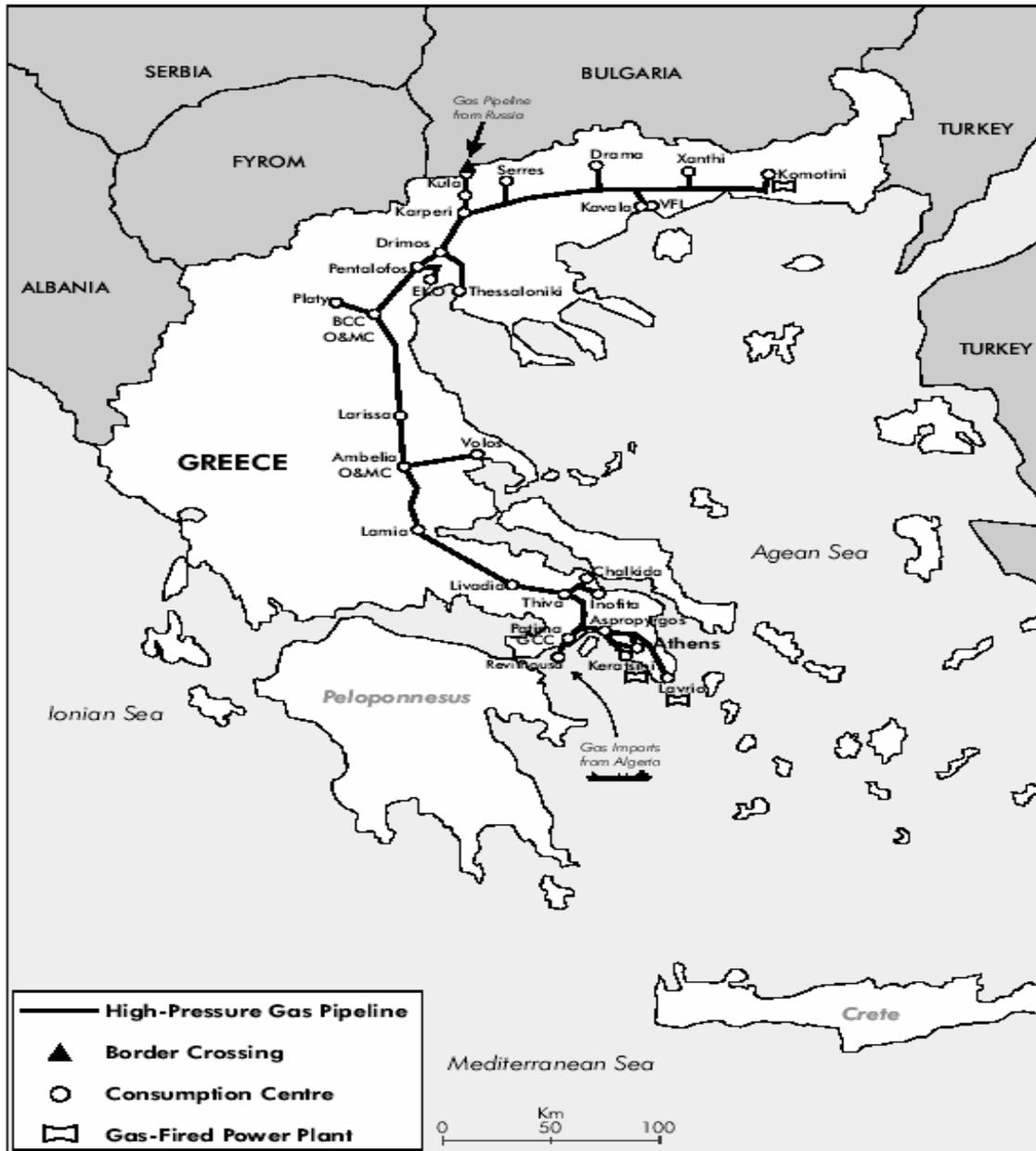
Figure 2.5: Greek transmission and distribution system
