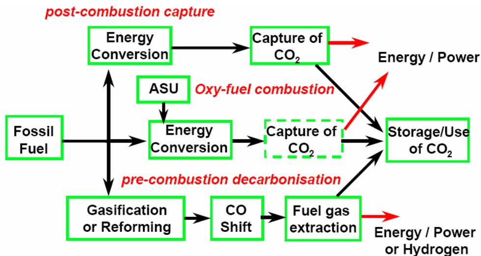
Figure 3.4: Carbon capture processes
