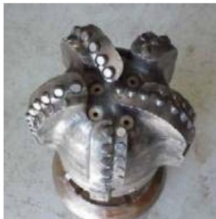
*Figure 1.8: Diamond studded drilling bit*
