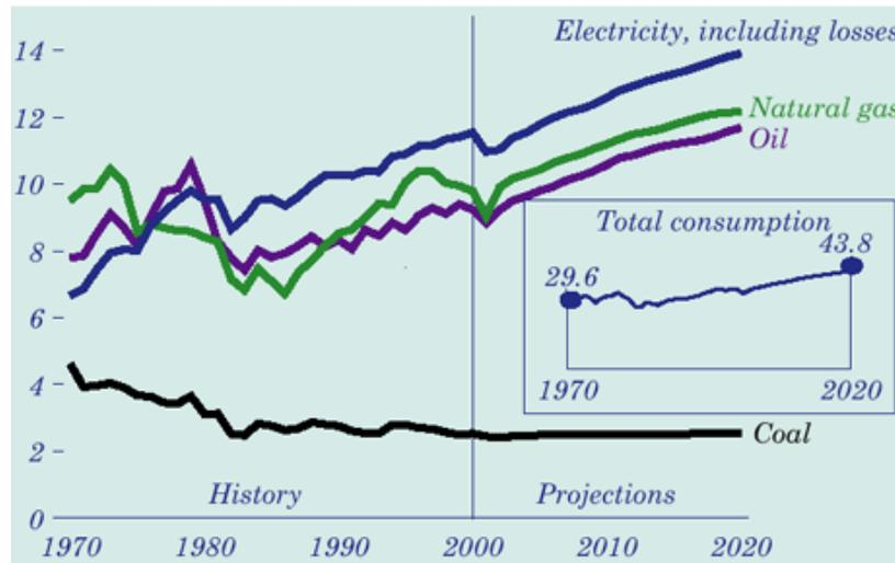
Figure 1.16: Industrial energy consumption by fuel in U.S.
