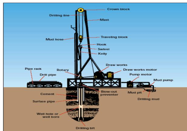
Figure 1.7: Onshore drilling technique
