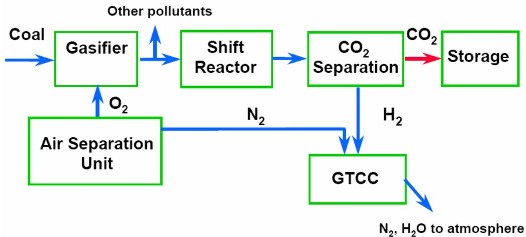
Figure 3.5: Pre-combustion capture
