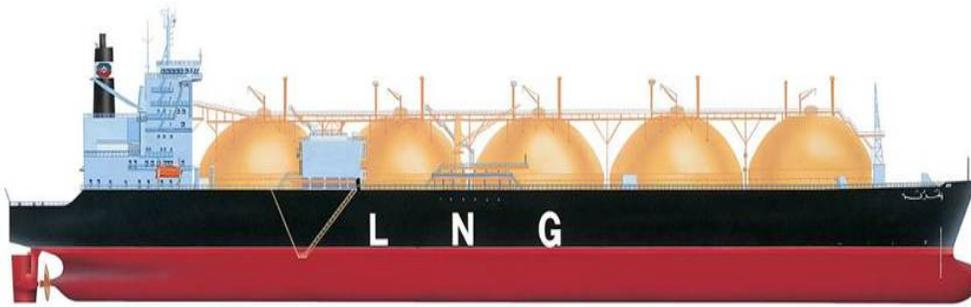
*Figure 1.11: Tanker carrying liquefied natural gas*
