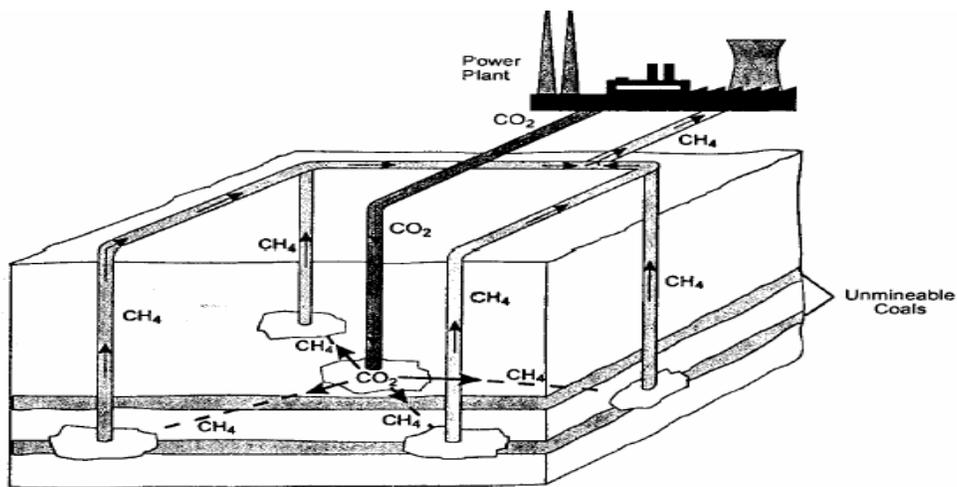
Figure 3.14: Methane recovery from CO<sub>2</sub> sequestration
