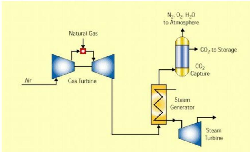
*Figure 3.9: Gas turbine combined cycle with post-combustion capture of CO<sub>2</sub>*
