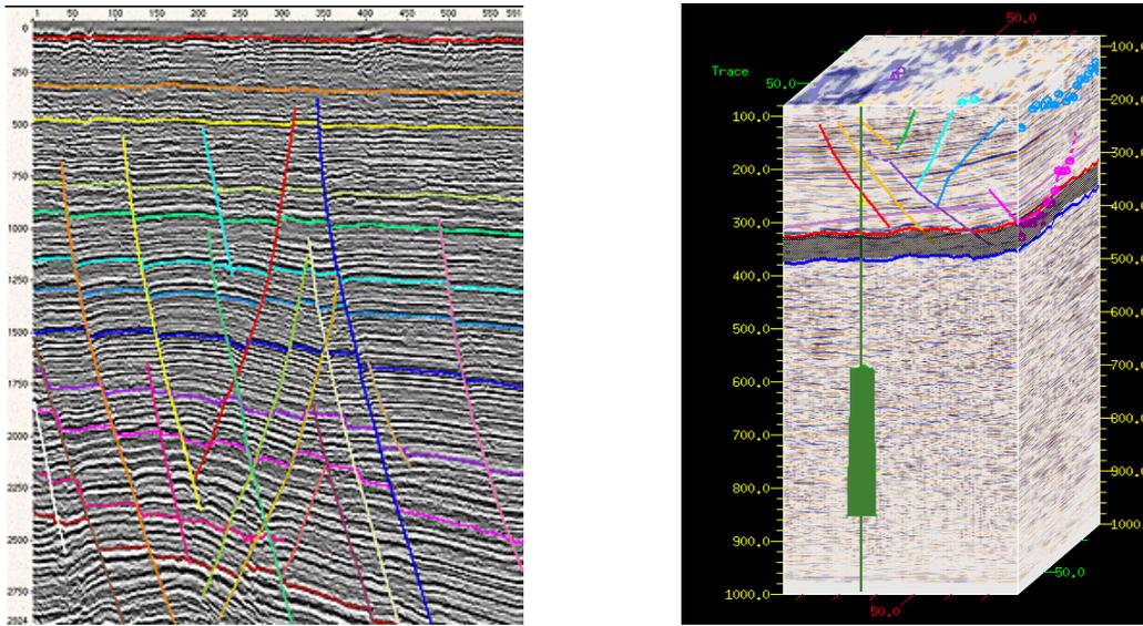
*Figure 1.4: Old 2-D provided data (left), Recent way of 3-D provided data (right)*
