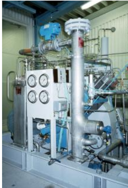
figure 10. A compact unit that scrubs and compresses biogas for use in alternative motor fuel
