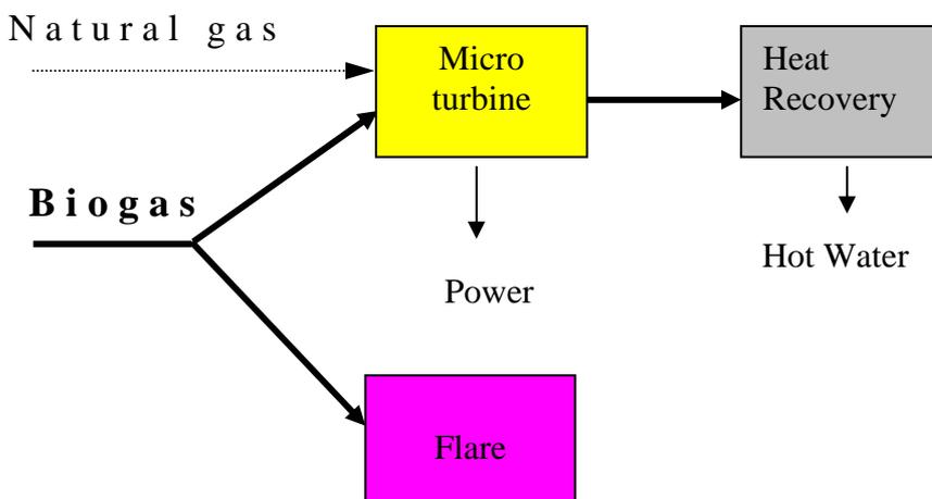
figure 18 . Case 2: Microturbine With heat Recovery
