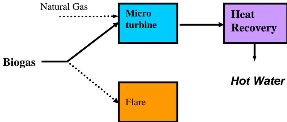
figure 22 . Case 2b:Microturbine with Heat Recovery
