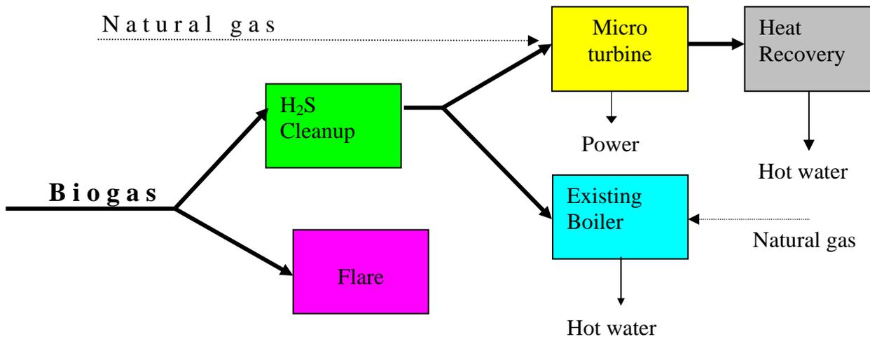
figure 19 . Case 3:H<sub>2</sub>S Removal and Microturbine with Heat Recovery
