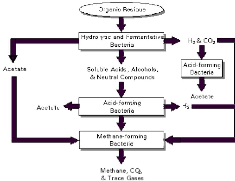
**figure 1.** Anaerobic digestion process
