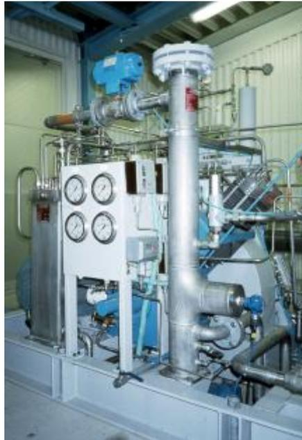
**figure 10.** A compact unit that scrubs and compresses biogas for use in alternative motor fuel
