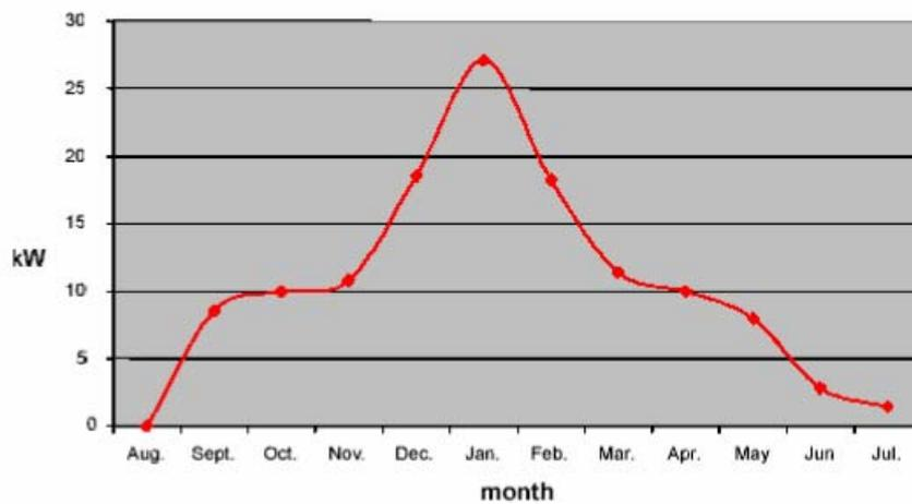
**figure 14.**Heat demand for the sewage treatment digester
