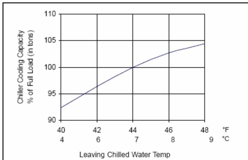
Figure II-5 example of variation on chiller capacity with chilled water temperature [8]
