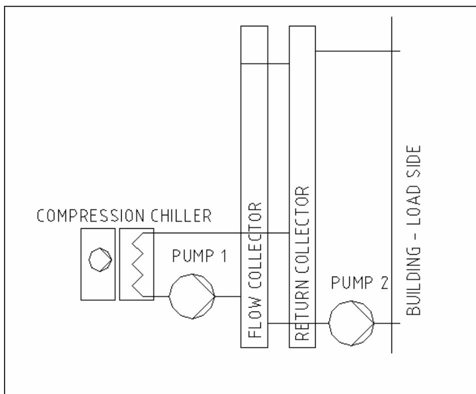
**Figure VI-1 option 1 schematic**
