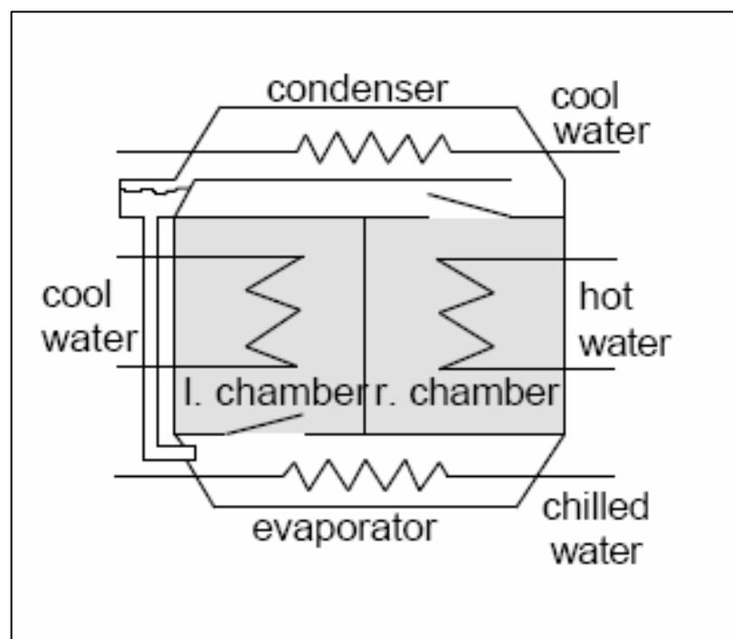
**Figure II-6 adsorption chiller schematic [10]**
