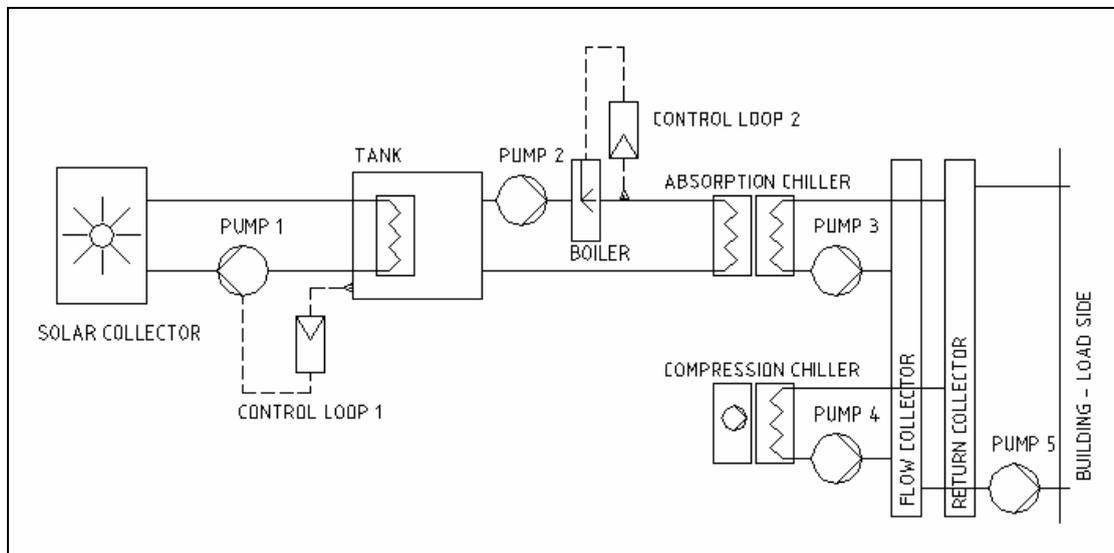
**Figure VI-4 schematic of absorption plant**
