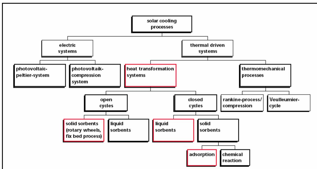
Figure II-1 overview of solar cooling methods [3]
