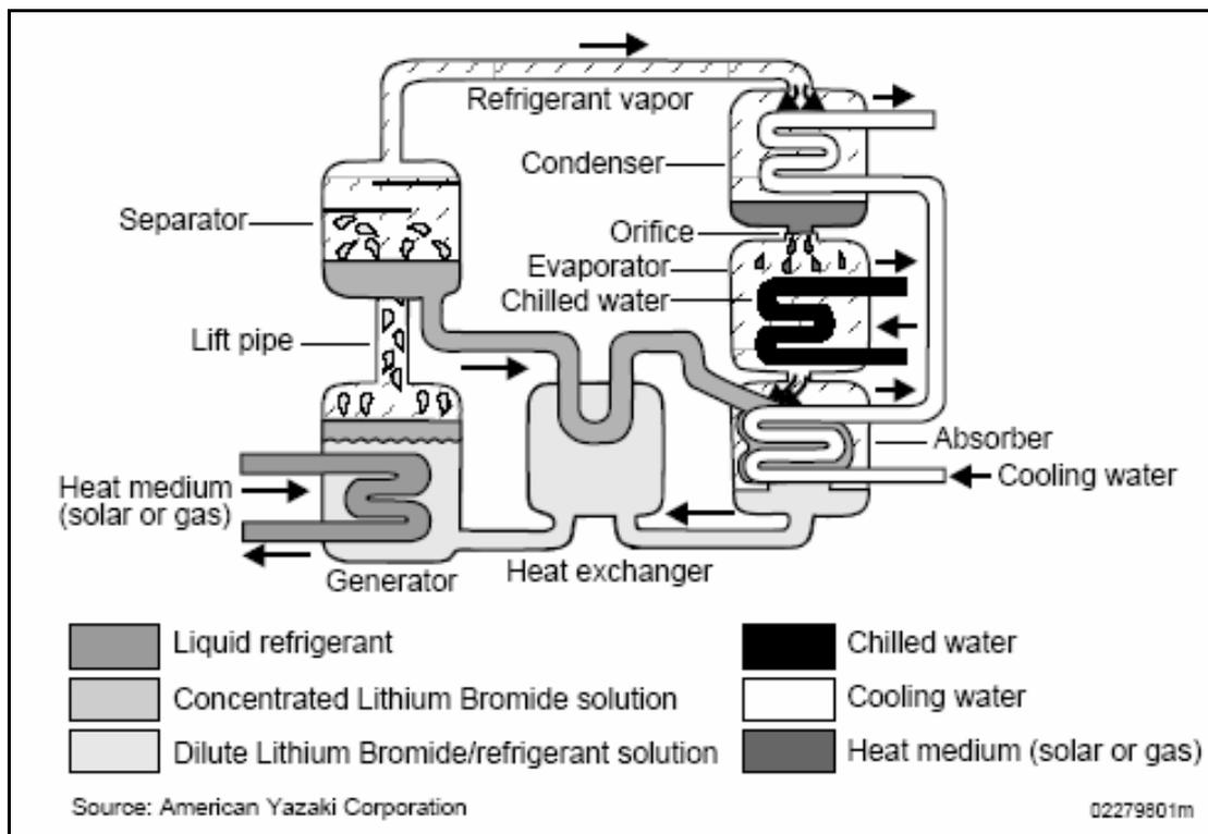
Figure II-4 absorption cycle [6]
