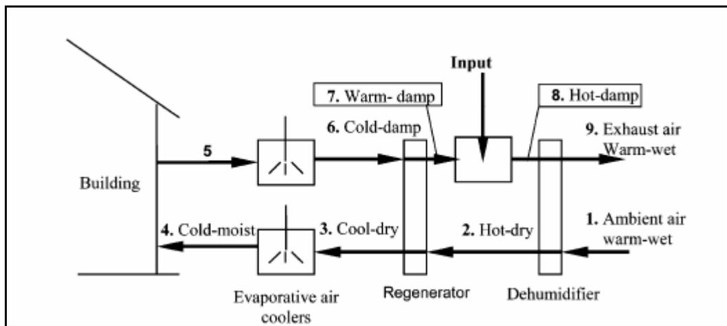
**Figure II-8 schematic of desiccant cooling [11]**
