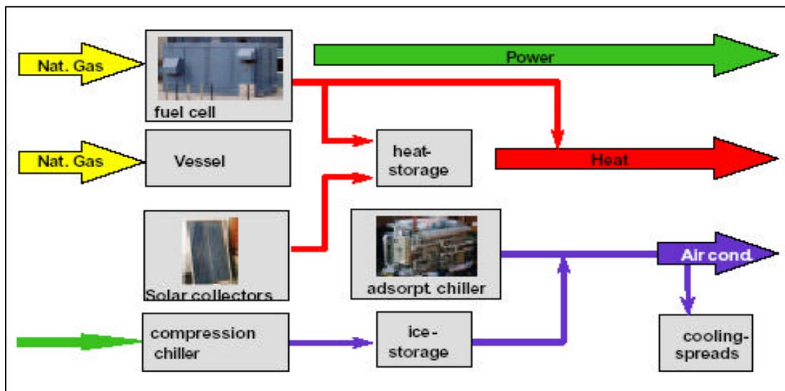
Figure III-2 schematic of Malteser's trigeneration scheme [10]
