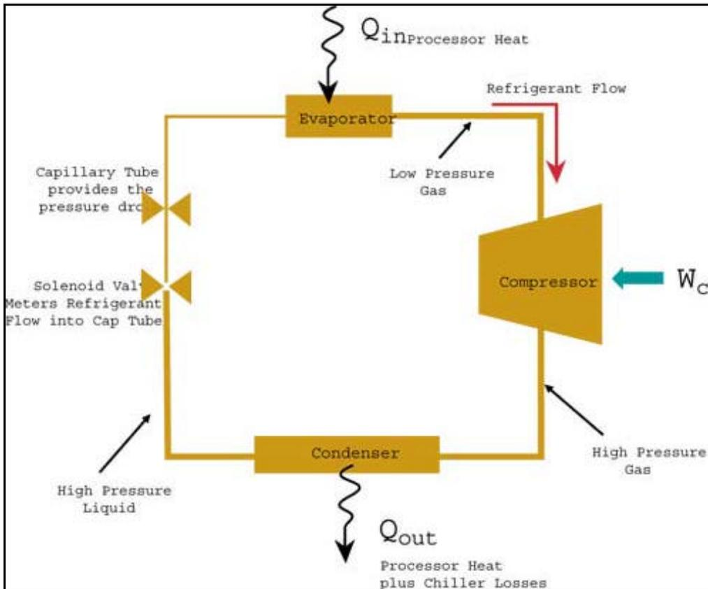
Figure II-3 compression refrigeration cycle [5]
