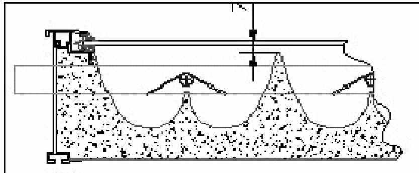
Figure III-5 schematic of CPC collector [11]
