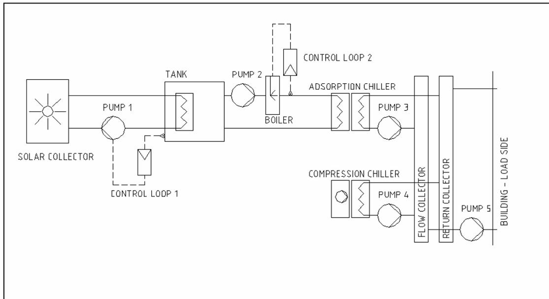
**Figure VI-5 adsorption plant schematic**
