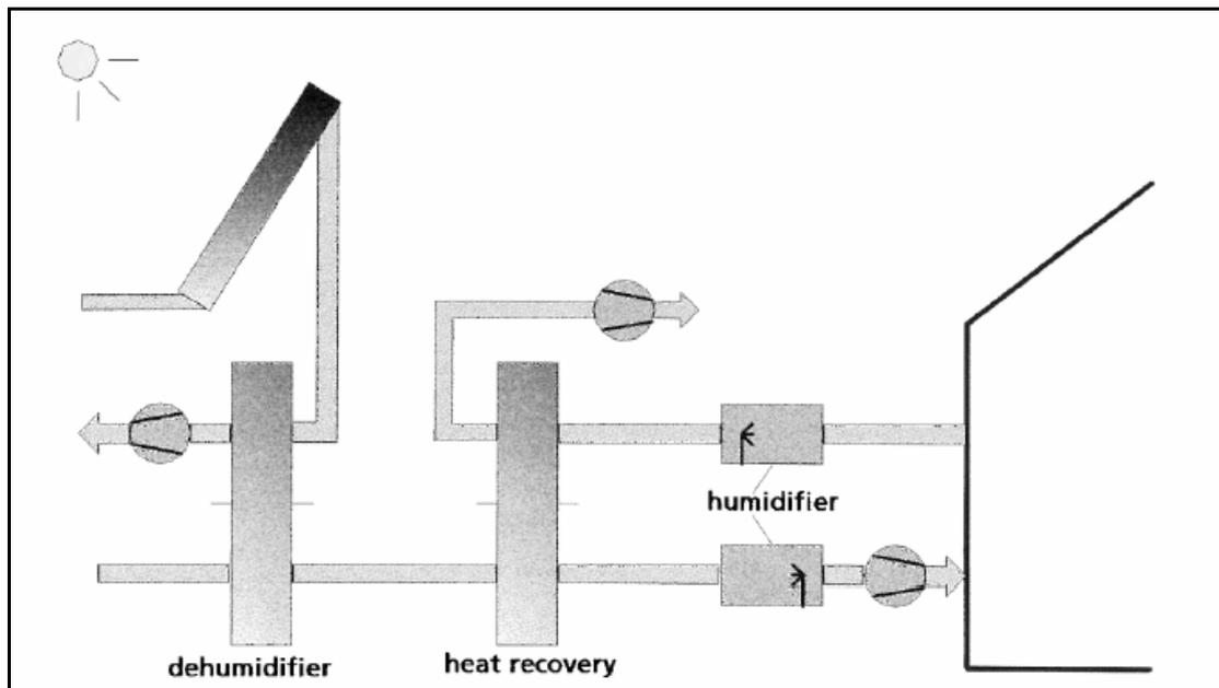
Figure II-10 schematic example of desiccant cooling system using outside air and air solar collectors [12]
