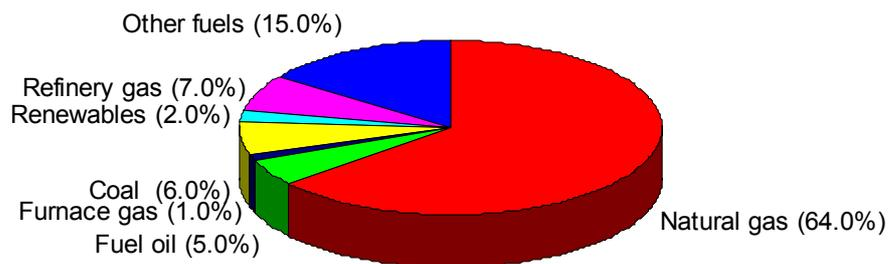
Figure 16 - Cogeneration plant fuel mix.
