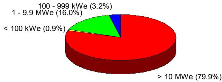
Figure 15 - Energy production depending on the cogeneration plant size.
