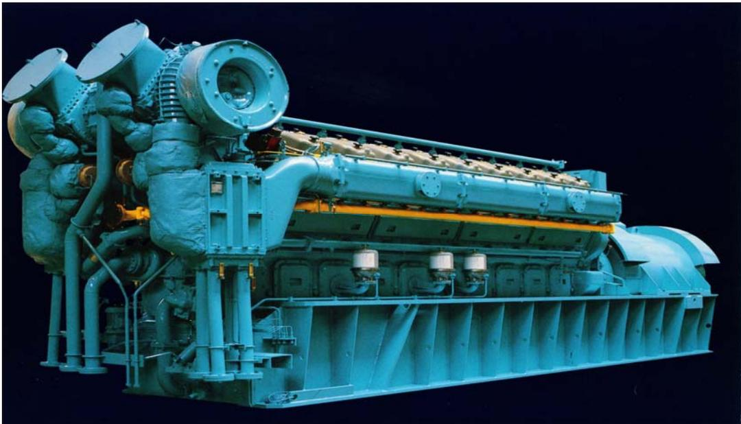
Figure 20 - Photograph of a 3MWe gas engine.
