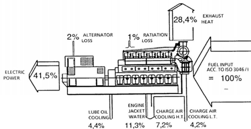
Figure 9 - Reciprocating gas engine sankey diagram.
