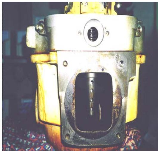
Figure 24 - Photograph of a gas engine cylinder head.
