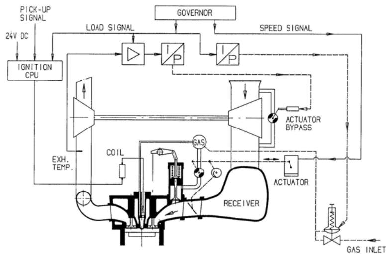
Figure 25 - Gas engine control system.
