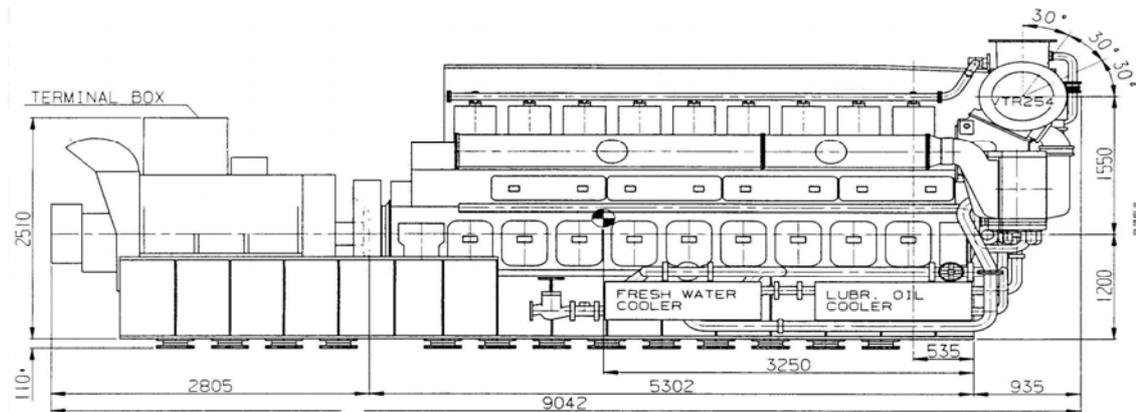
Figure 21 - Gas engine elevation drawing.
