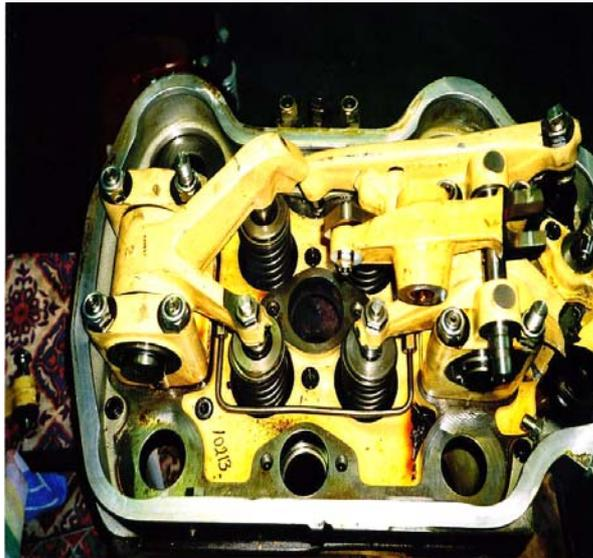
Figure 23 - Photograph of a gas engine cylinder head.
