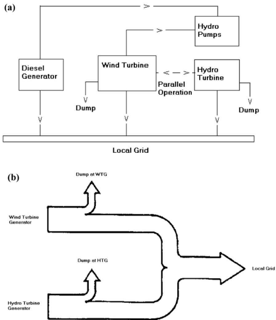
Figure 5.6: Schematic diagram of (a) the combined system and (b) energy flow
