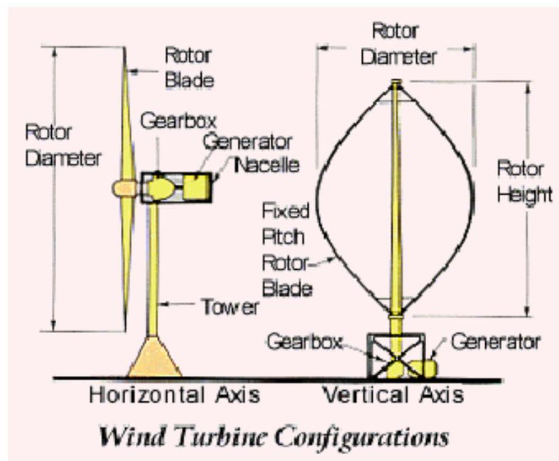
**Figure 3.1: Wind turbine configurations**
