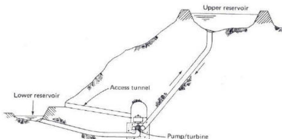
**Figure 4.1: A diagram of pumped hydro storage**
