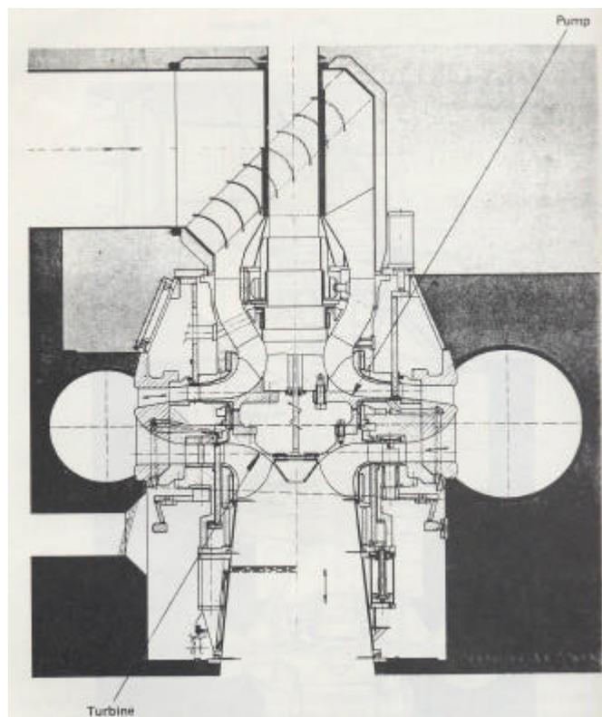
**Figure 4.8: Isogyre pump/turbine**
