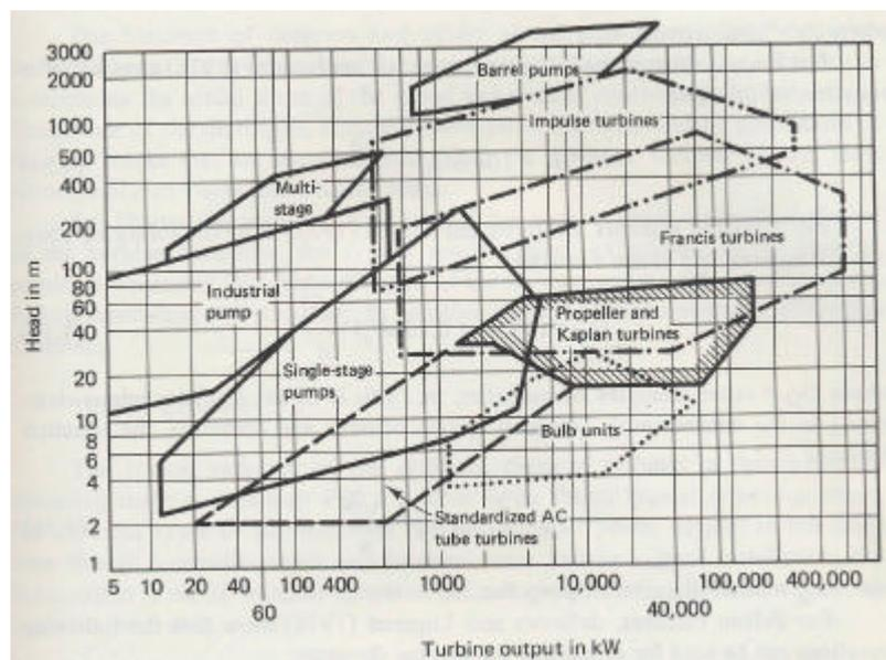
**Figure 4.9: Application ranges for various types of turbines**
