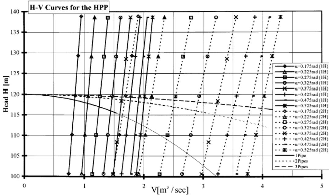
Figure 5.9: Operational (H-V) curves for the power hydro station
