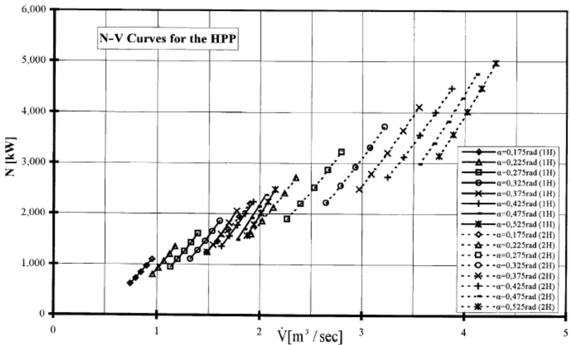
Figure 5.10: Operational (P-V) curves for the power hydro station
