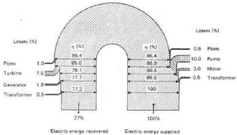
**Figure 4.2: Energy storage cycle for a large pumped plant**
