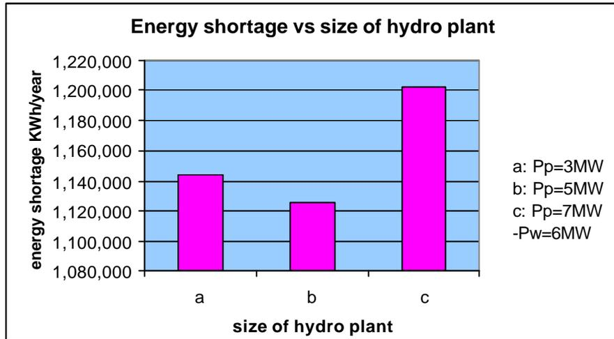
**Figure 6.9: The relationship between the energy shortage and the size of hydro plant**
