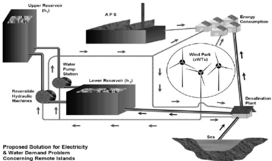
**Figure 5.7: A combined power system for remote islands**
