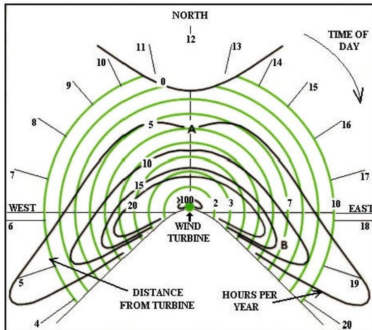
**Figure 3.3 An example of a shadow flicker calculation**
