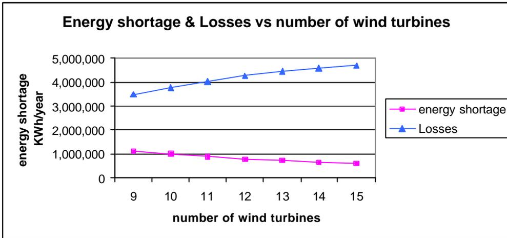
**Figure 6.7: Energy shortage and losses vs size of wind farm**
