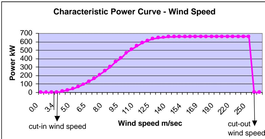
**Figure 3.2: Characteristic wind speed-power curve**
