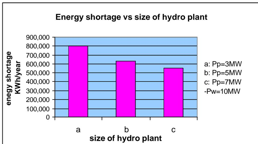
**Figure 6.10: The relationship between the energy shortage and the size of hydro plant**
