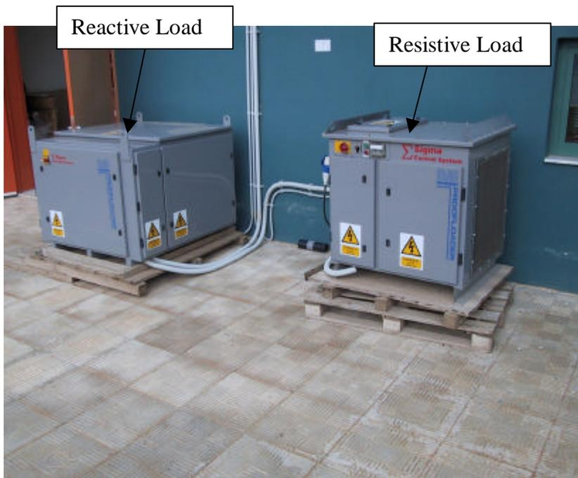
Figure 4- Resistive & Reactive Loads of the test circuits.
