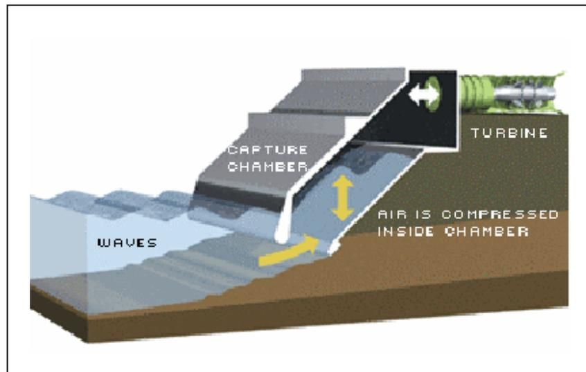
Figure 3: How the LIMPET 500 operates
