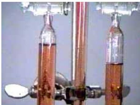
Figure 5: Resulting Gas collection, H<sub>2</sub> on right
