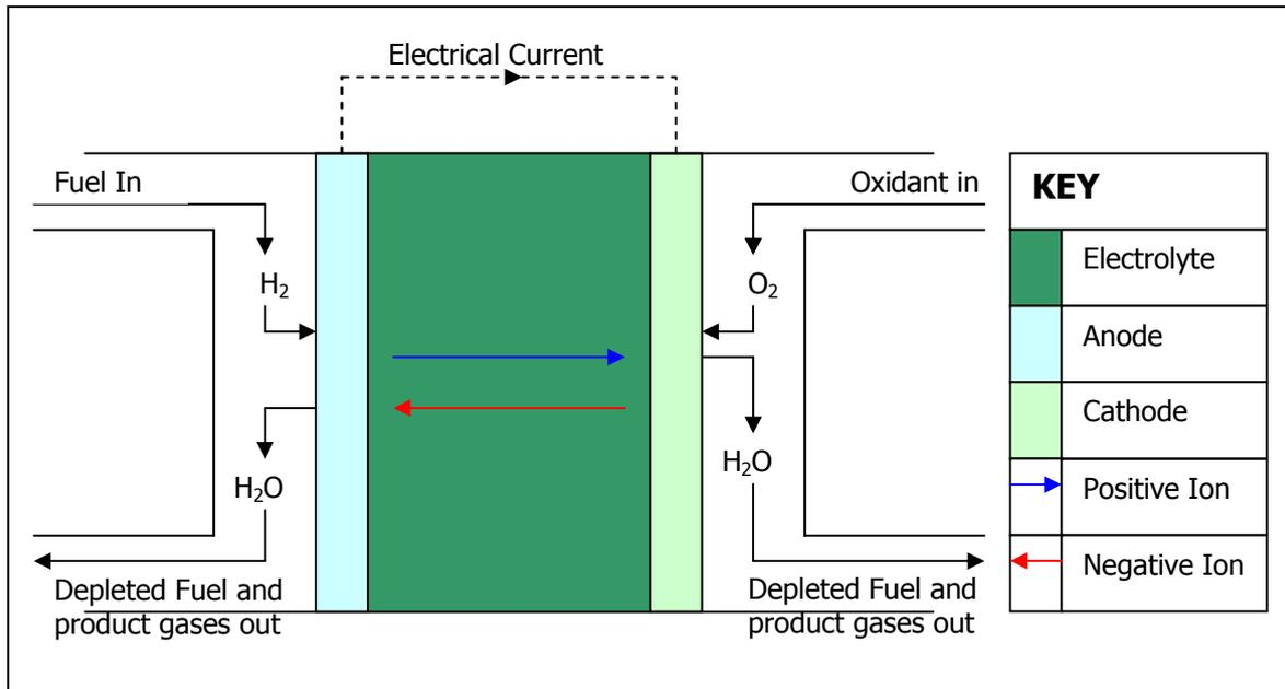
Figure 8: Fuel Cell Schematic Diagram
