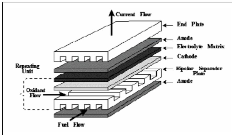
Figure 9: Components of a fuel cell stack<sup>11</sup>
