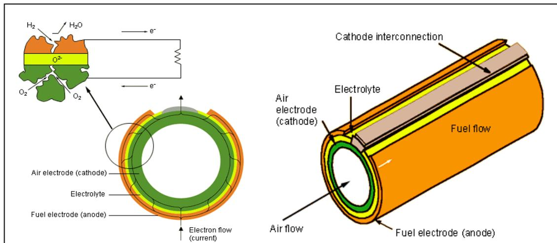
Figure 14: Siemens Tubular Solid Oxide Fuel Cell
