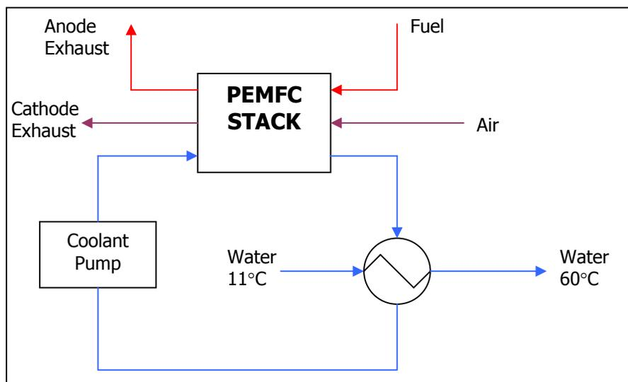
Figure 11: Example of a hot water cogeneration system
