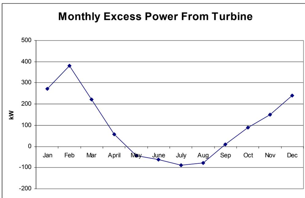
Figure 23: Average Monthly Excess power provided by the LIMPET 500
