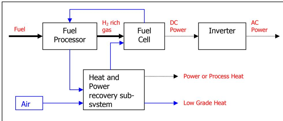
Figure 10: Components of a fuel cell cogeneration system with external reformer
