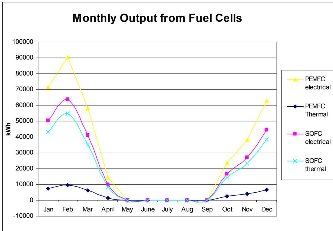
Figure 27: Potential monthly heat and electrical output from Fuel Cells
