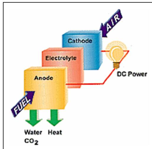
Figure 7: How fuel cells work
