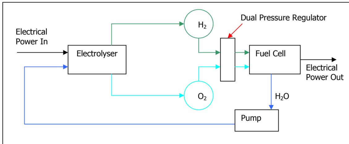
Figure 12: Regenerative fuel cell system
