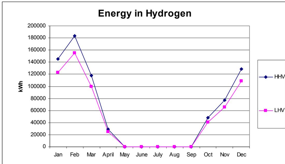
Figure 26: Energy available in hydrogen for higher and lower heating values
