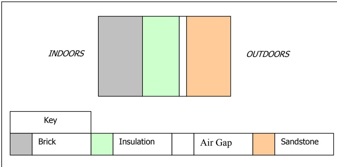
Figure 19: Components of typical external wall
