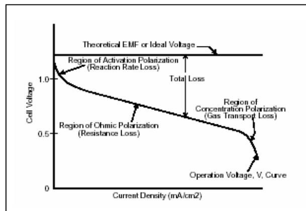
Figure 13: Ideal and Actual Fuel Cell Voltage/Current characteristic<sup>14</sup>
