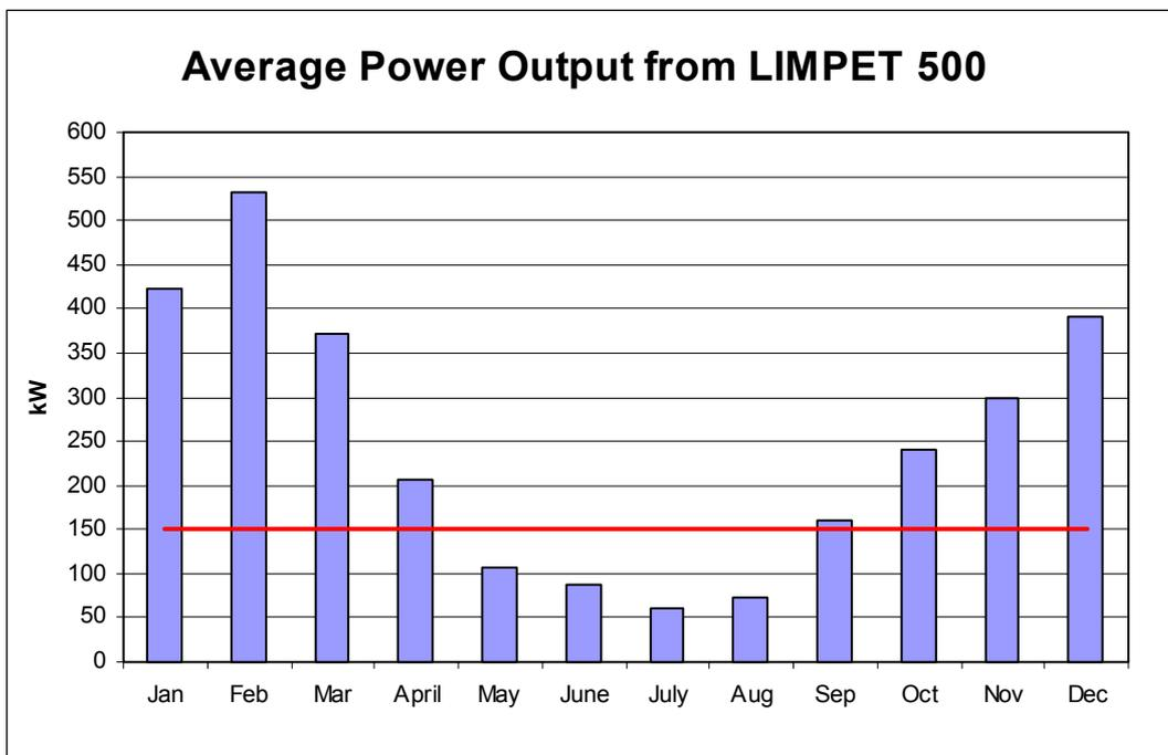
Figure 33: The average monthly output from the LIMPET 500 and the level of grid restriction
