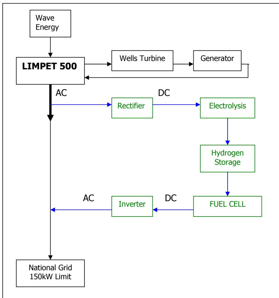
Figure 15: Simple Schematic of Entire System
