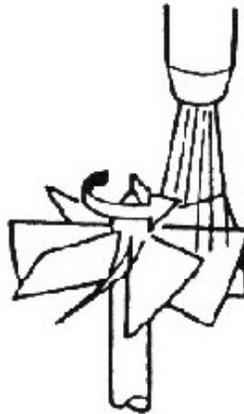
The momentum of a high-speed water jet turns impulse turbines.
