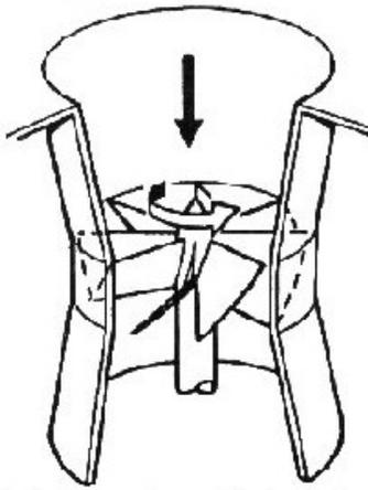
Hydrodynamic lift forces acting on the runner blades turn reaction turbines.
