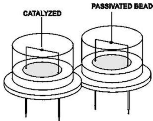
Figure 3.3.1.1, Catalytic Bead Sensor
