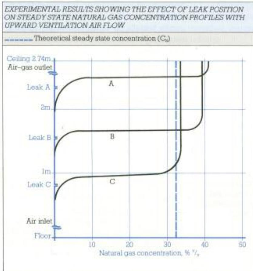
EXPERIMENTAL RESULTS SHOWING THE EFFECT OF LEAK VELOCITY AND LEAK POSITION ON STEADY STATE NATURAL GAS CONCENTRATION PROFILES FOR UPWARD VENTILATION AIR FLOW
