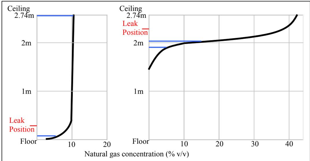
Figure 3.2.1, Possible height for detecting natural gas
