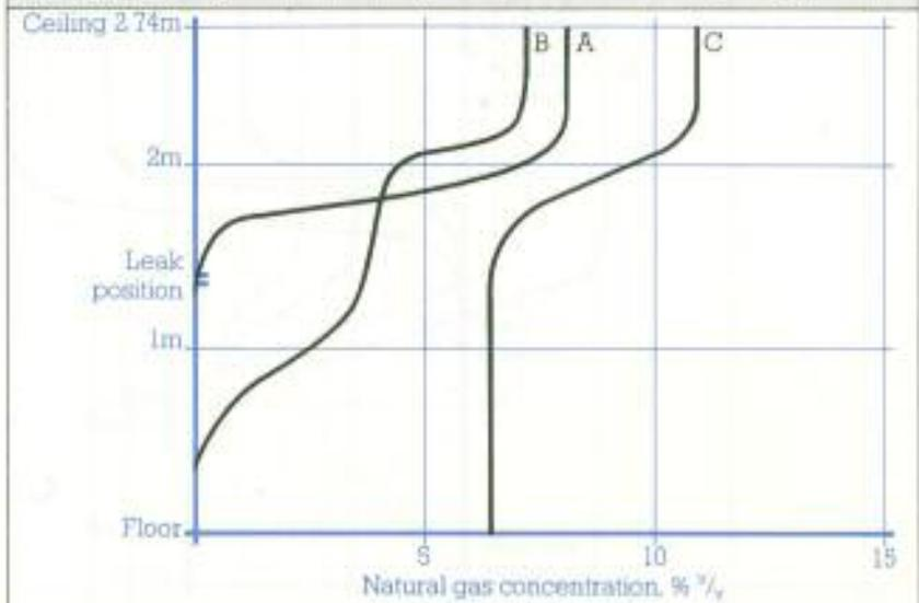
Gas flow rate  $1.42\text{m}^3/\text{h}$  - all cases · Room height  $2.74\text{m}$  · Air flow direction  $\rightarrow$
