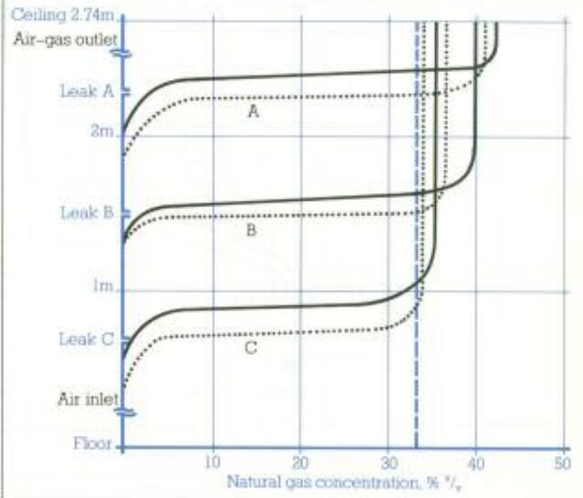
*EXPERIMENTAL RESULTS SHOWING THE EFFECT OF VENTILATION RATE ON STEADY STATE NATURAL GAS CONCENTRATION FOR UPWARD VENTILATION AIR FLOW*
