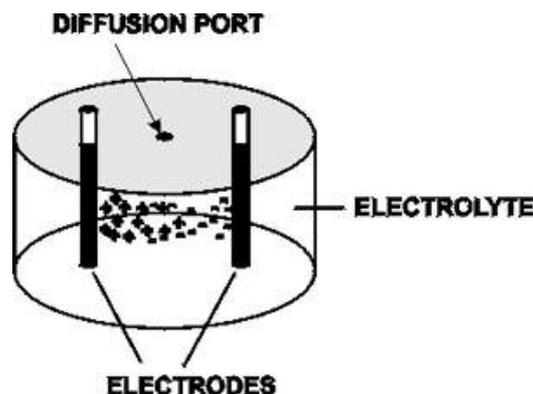
Figure 3.3.3.1, Electrochemical Sensor
