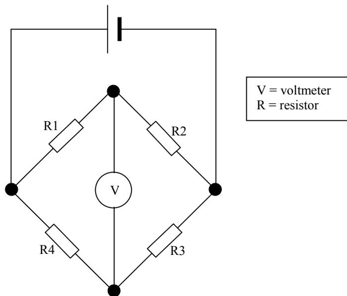
Figure 3.3.1.2, Typical Wheatstone Bridge Circuit
