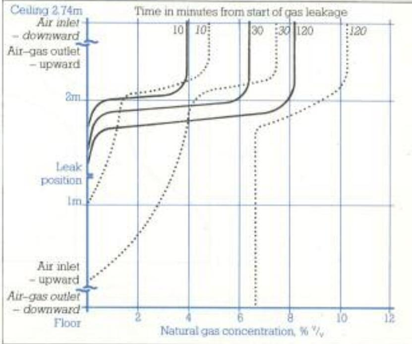
**EXPERIMENTAL RESULTS SHOWING STEADY STATE NATURAL GAS CONCENTRATION PROFILES FOR DIFFERENT VENTILATION PATTERNS**
