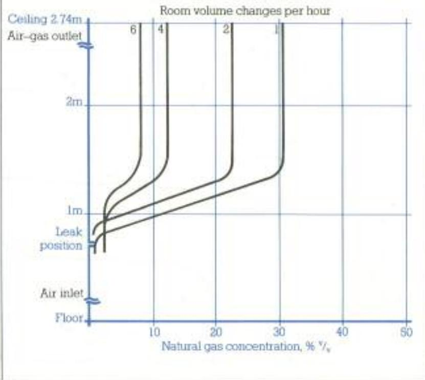
**EXPERIMENTAL RESULTS SHOWING THE BUILD-UP OF NATURAL GAS CONCENTRATION WITH TIME FOR UPWARD AND DOWNWARD VENTILATION AIR FLOW**
