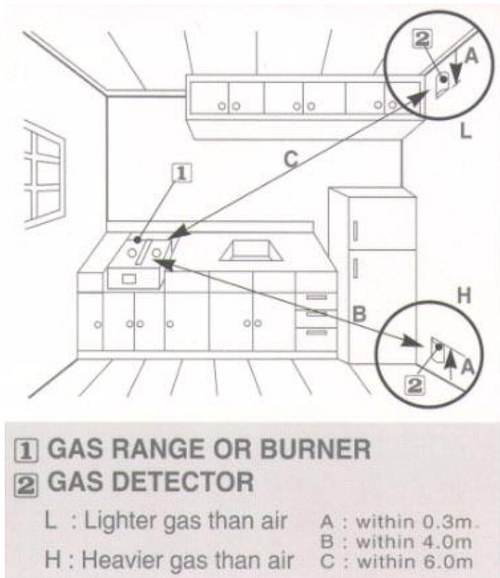
Figure 3.2.2, Typical positions for installing gas detection sensors (exact distance may vary dependant on the sensor design)
