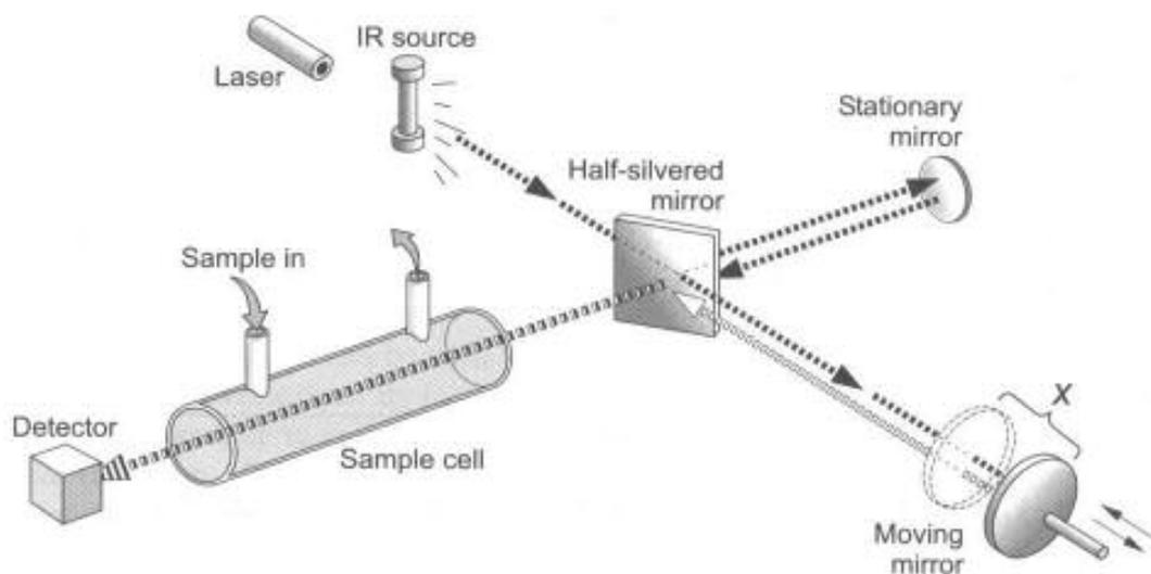
Figure 3.3.4.1, Basic Fourier Transform Infrared spectrometer
