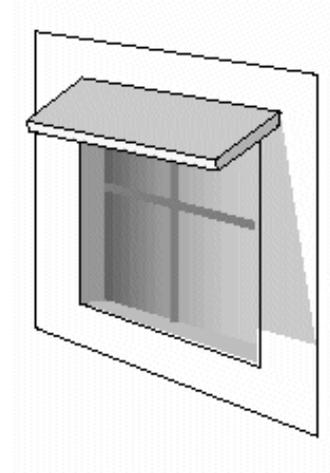
Figure 3.7: Solid sloping overhang <sup>[3]</sup>
