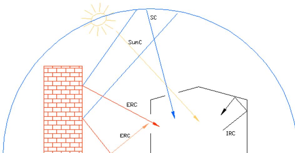
Figure 2.4: Components of Daylight
