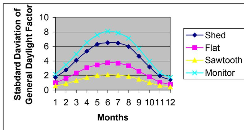
Figure 5.11 : Standard deviation of General Daylight Factor for different roof geometry
