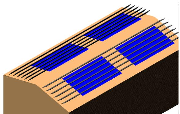
Figure 3.11: Perspective view of shed roof with slopping shading
