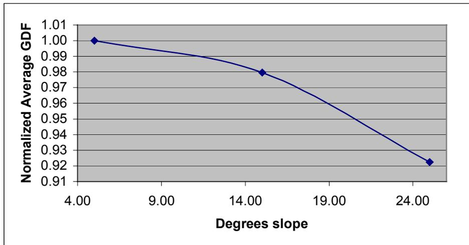
Figure 5.2 : Normalized average General Daylight Factor reduction with roof slope
