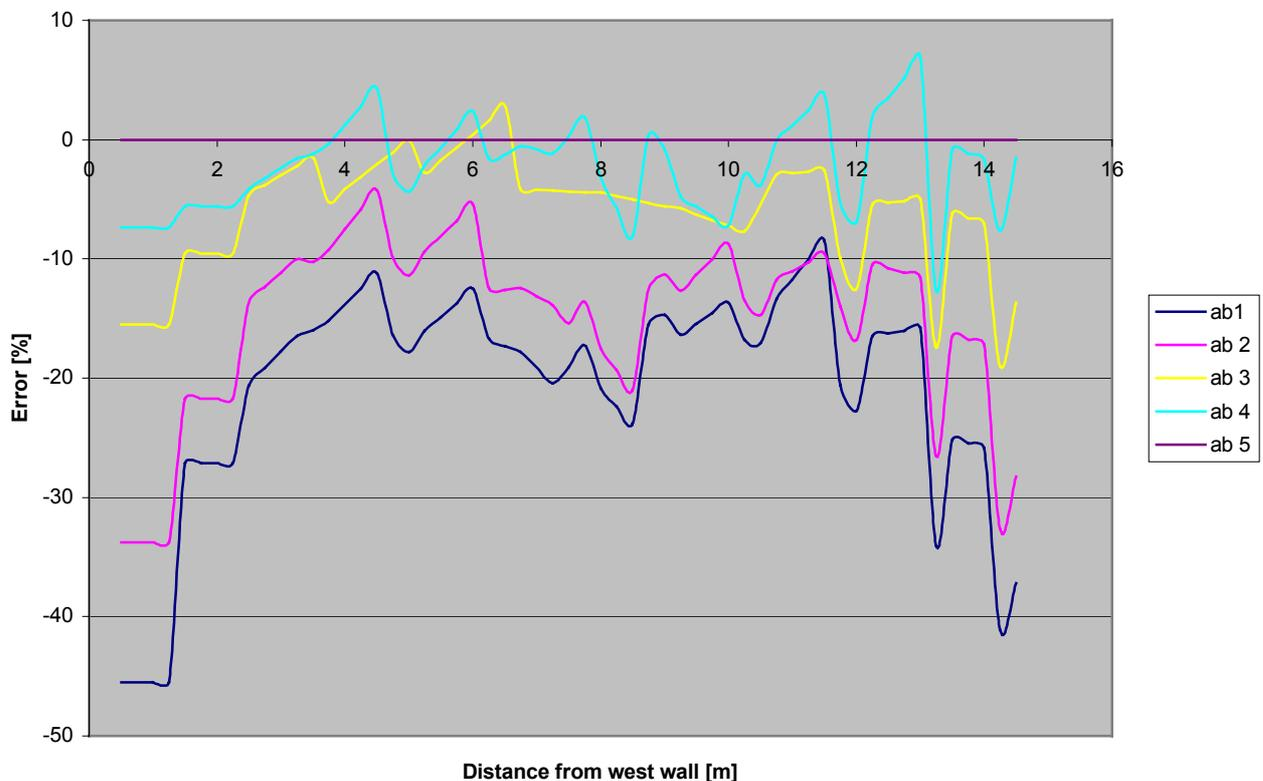
Figure 4.2 : General Daylight Factor error for different number of ambient bounces
