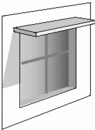
Figure 3.3: Solid horizontal overhang <sup>[3]</sup>
