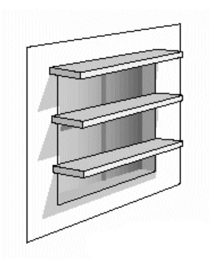
Figure 3.8: Parallel horizontal overhangs for better light distribution <sup>[3]</sup>
