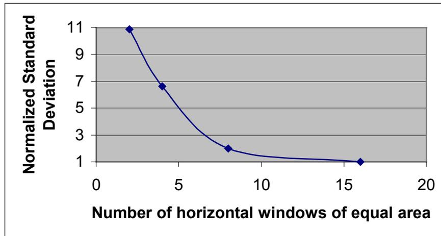
Figure 5.5: Normalized Standard deviation of General Daylight Factor with the number of horizontal windows of equal area
