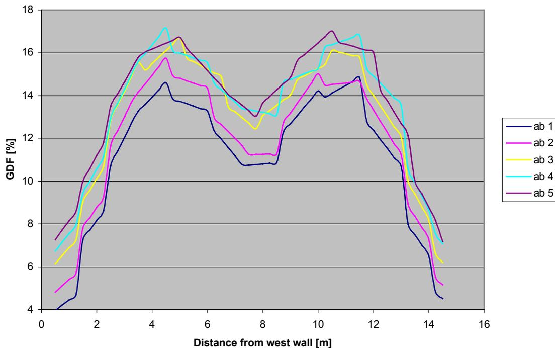
Figure 4.1: General Daylight Factor plots for different ambient bounces number
