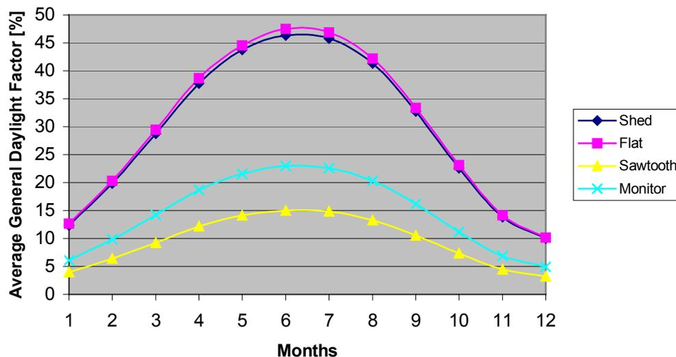
Figure 5.9 : Average General Daylight Factor through out the year
