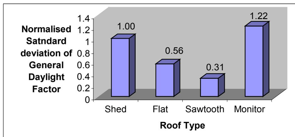
Figure 5.12 : Normalised standard deviation of General daylight factor for different type of roof geometry
