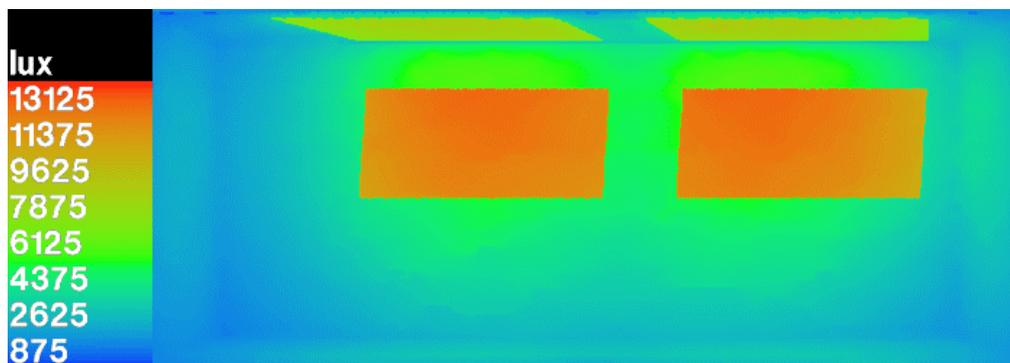
Picture 5.1 : Illuminance level in the interior of a space with shed roof on 15<sup>th</sup> of June at 13:00
