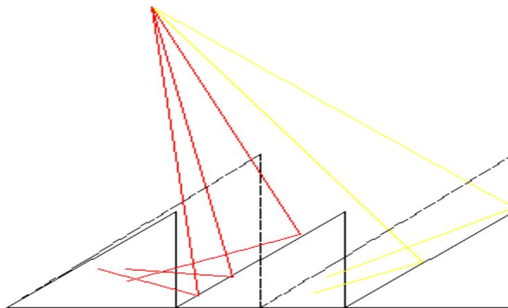
Figure 5.7 : Reflection of sun rays of high altitude of a sawtooth roof with two and three 'saws'
