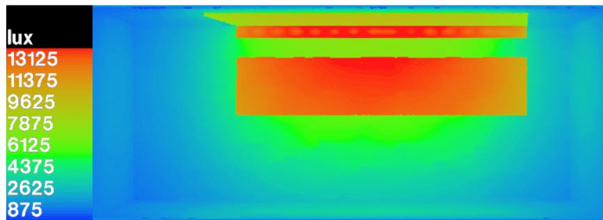
Picture 5.3 : Illuminance level with flat roof and two horizontal windows on 15<sup>th</sup> of June at 13:00
