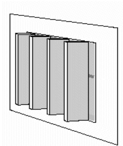
Figure 3.9: Vertical shading device (louvers) for east and west facades <sup>[3]</sup>
