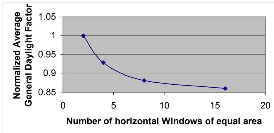
Figure 5.4 : Normalized average General Daylight Factor reduction with the number of horizontal windows of equal area
