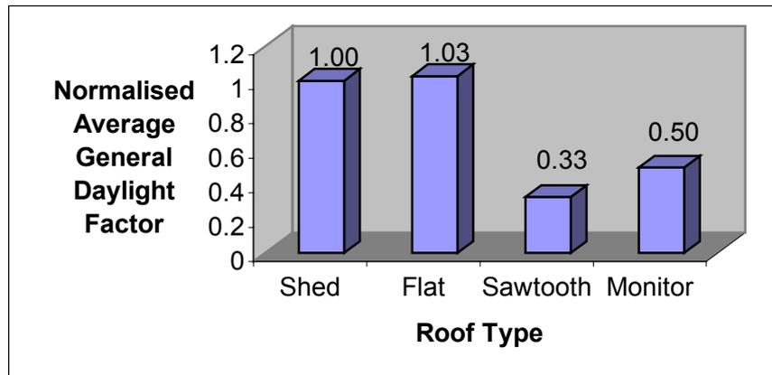
Figure 5.10: Normalised average General Daylight Factor for different type of roof geometry
