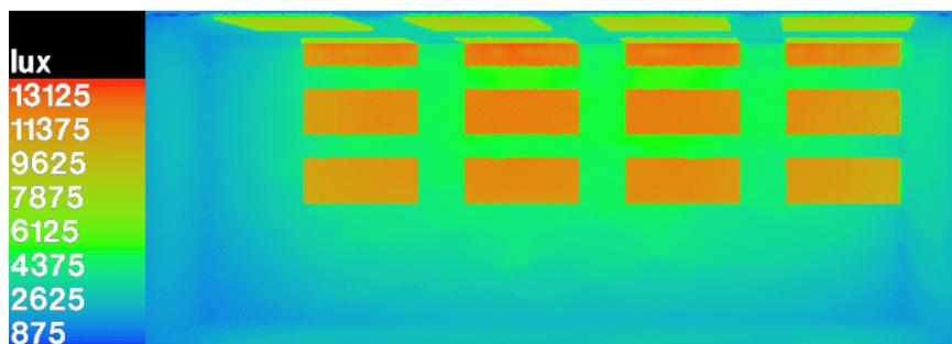
Picture 5.6: Illuminance level with flat roof and sixteen horizontal windows on 15<sup>th</sup> of June at 13:00
