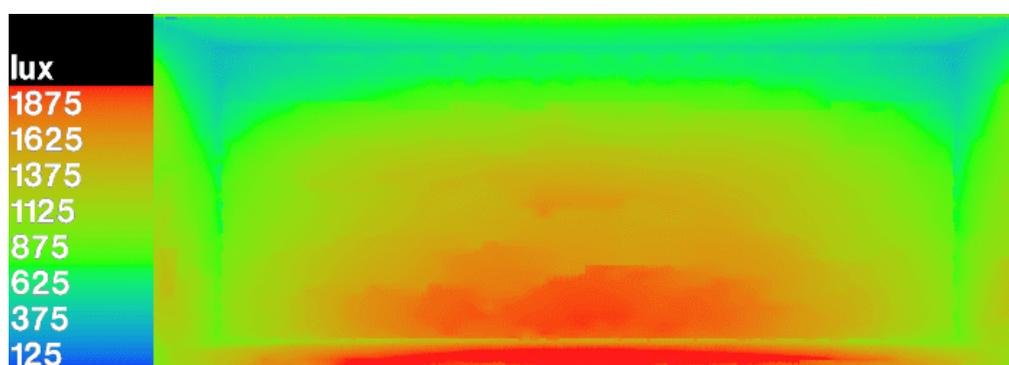
Picture 5.7 : Illuminance distribution with two 'saws' on 15<sup>th</sup> of June at 13:00
