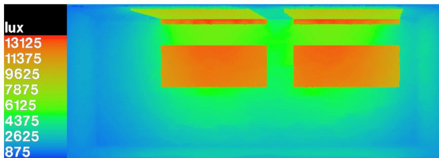
Picture 5.4: Illuminance level with flat roof and four horizontal windows on 15<sup>th</sup> of June at 13:00
