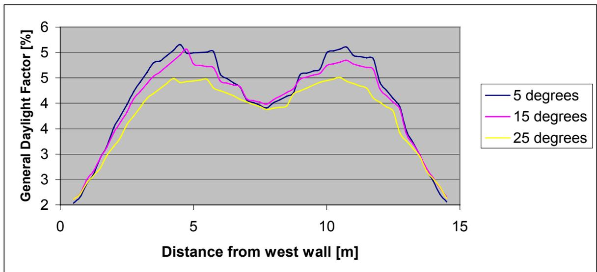
Figure 5.1 : Variation of GDF of shed models with 5, 15 and 25 degrees roof slope
