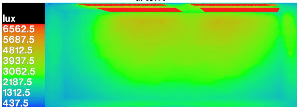
Picture 5.2 : Illuminance level in the interior of a space with shed roof on 15<sup>th</sup> of March at 13:00
