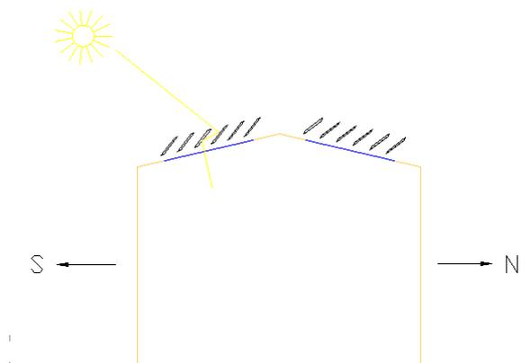
Figure 3.10: Shed roof with slopping shading
