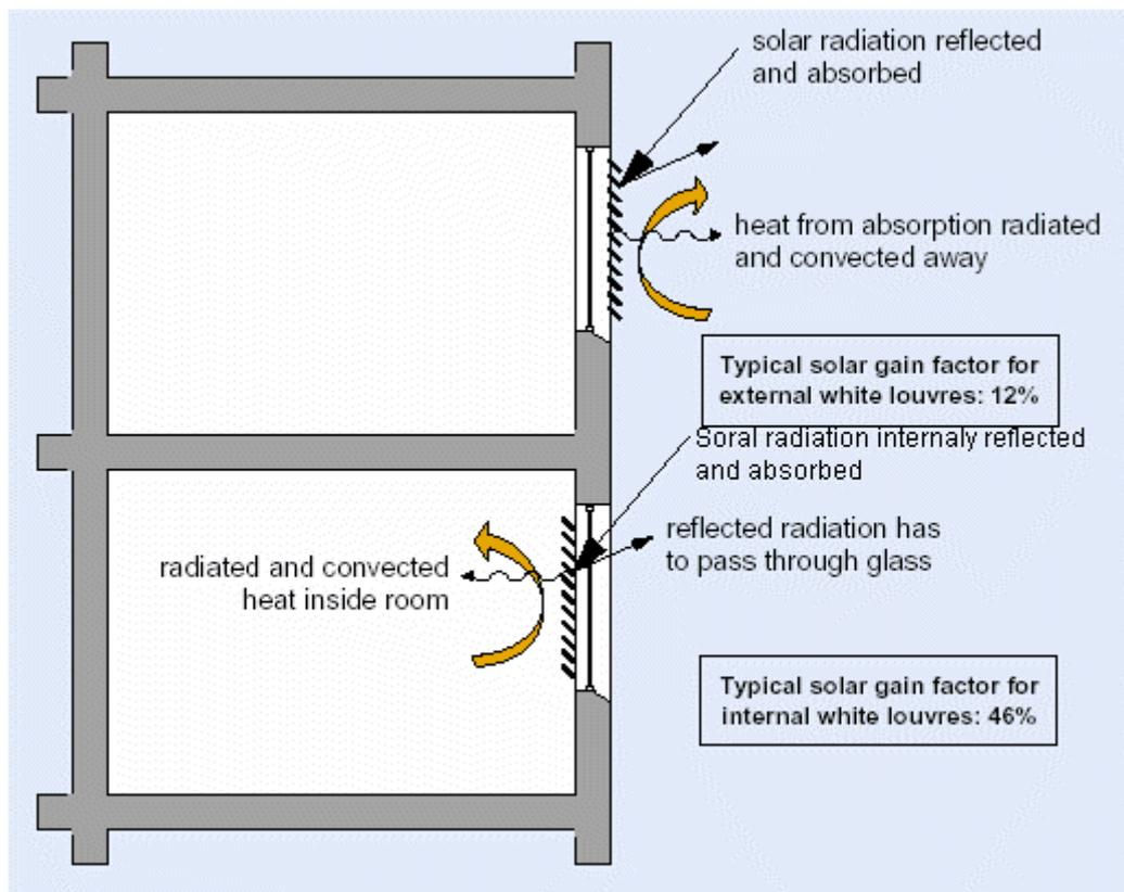
Figure 3.1 External versus Internal shading device <sup>[2]</sup>
