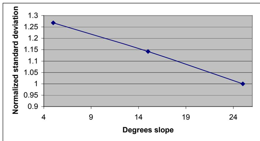
Figure 5.3 Normalized Standard deviation of General Daylight Factor with roof slope
