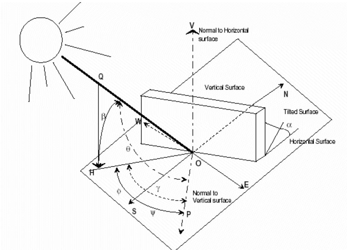
Figure 2.2: The solar altitude angle ( $\beta$ ), solar azimuth angle ( $\Phi$ ), surface azimuth ( $\Psi$ ), surface solar azimuth angle ( $\gamma$ ), the angle of incidence ( $\theta$ ), and the tilt angle ( $\alpha$ ) for an arbitrarily tilted surface [2].
