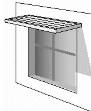
Figure 3.4: Louvers horizontal overhang
