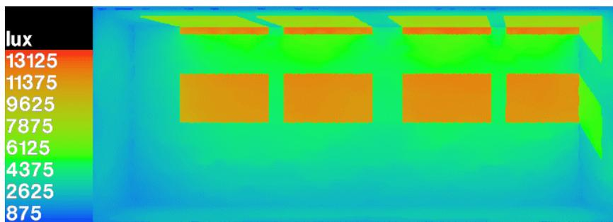
Picture 5.5: Illuminance level with flat roof and eight horizontal windows on 15<sup>th</sup> of June at 13:00
