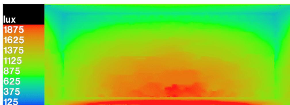
Picture 5.8 : Illuminance distribution with three 'saws' on 15<sup>th</sup> of June at 13:00
