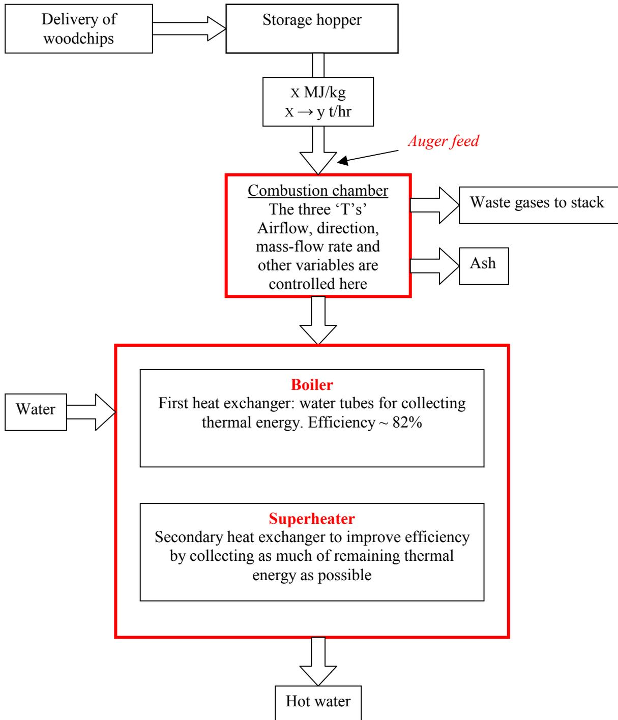
Fig. 30: Model for wood burning boiler [19]
