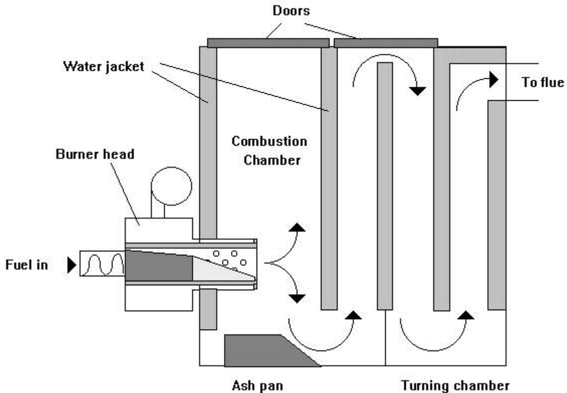
Fig. 36: The Stoker-burner attached to a purpose designed steel boiler [18]
