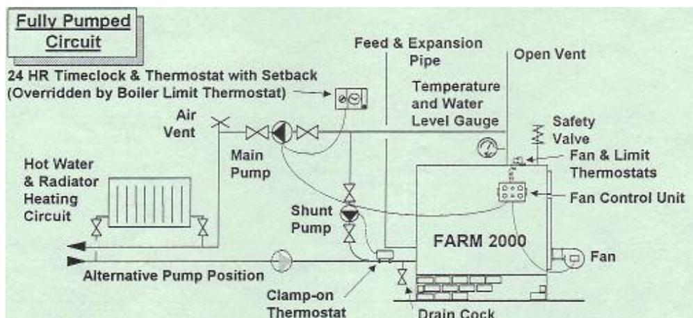
Fig.39: Woodchip boiler ('Farm 2000' model) connected into a Fully Pumped circuit [23]
