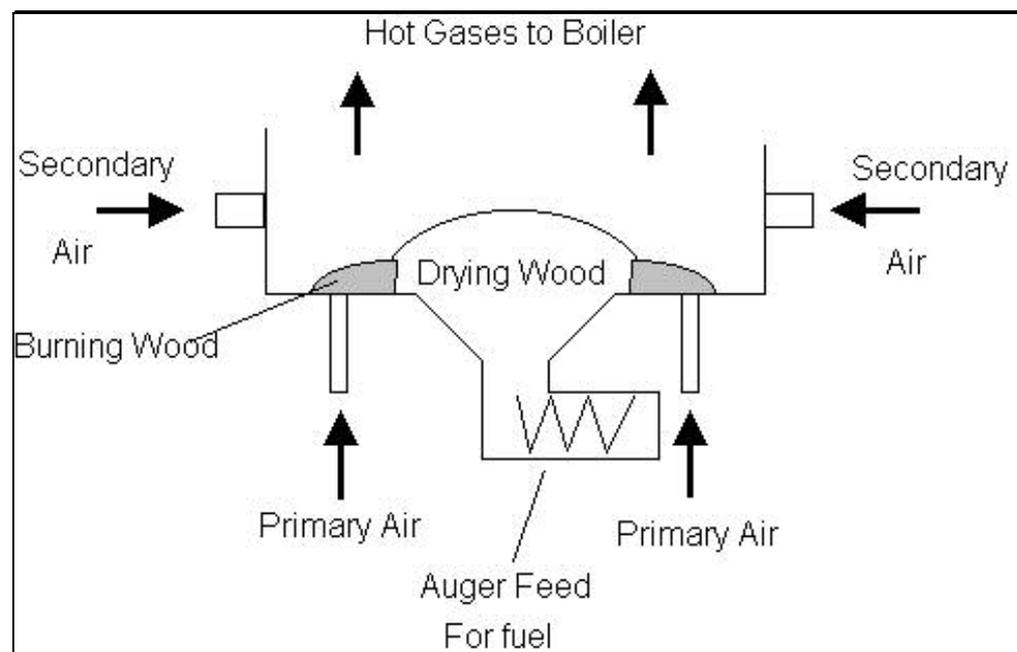
Fig. 33: The Underfeed Stoker arrangement [18]
