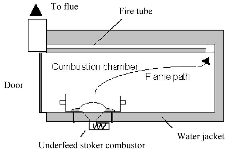
Fig. 34: Underfeed Stoker, shell and tube boiler [18]
