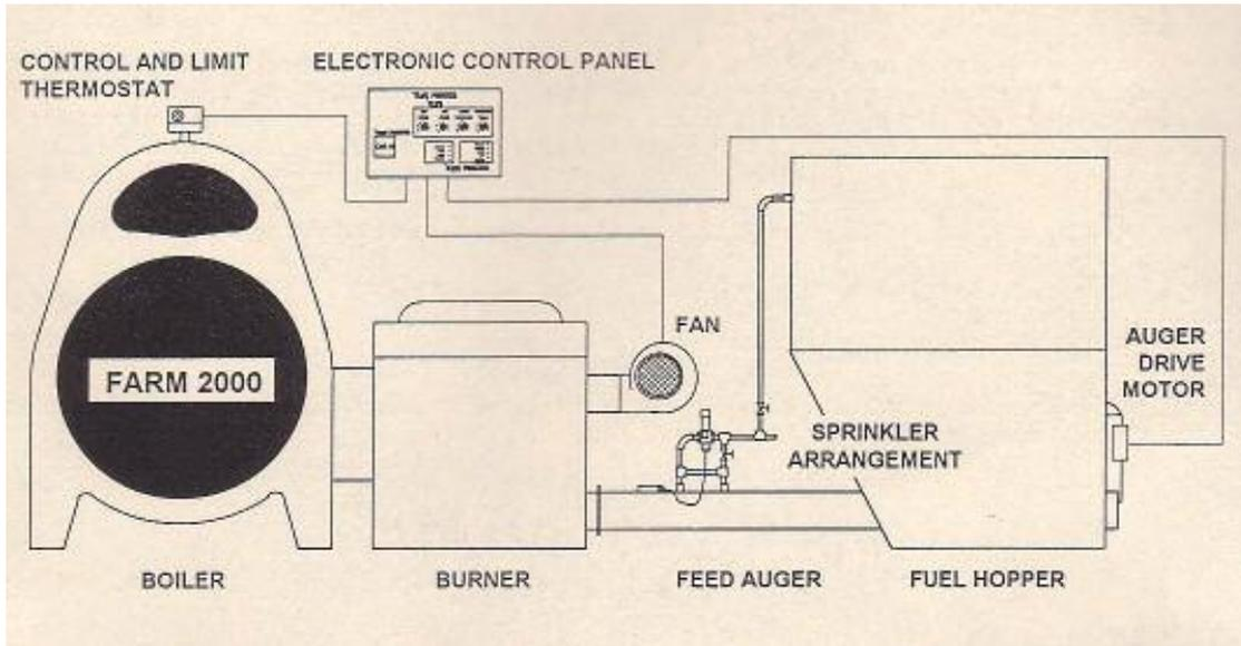
Fig.32 (b): The above woodchip system in schematic form, showing key components [23]
