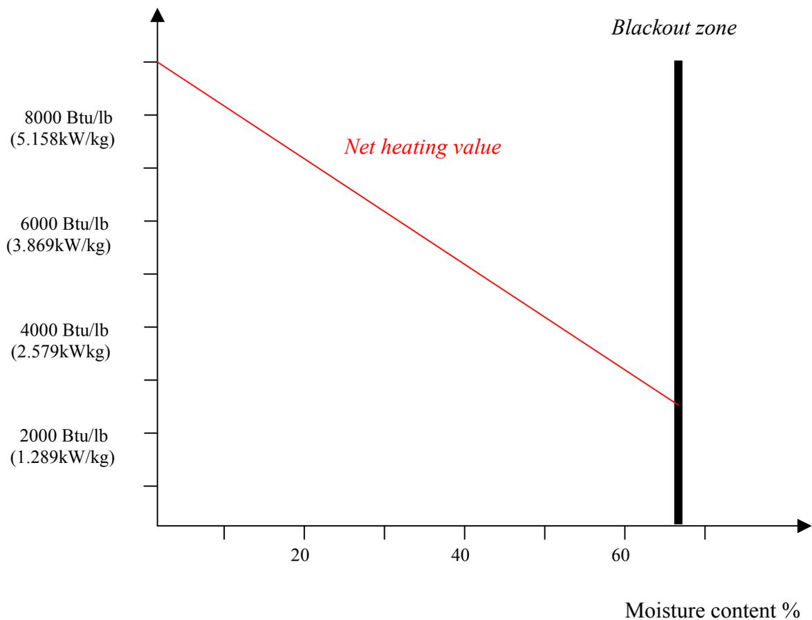
Fig. 21: The Effect of moisture on the heating value of wood [16]
