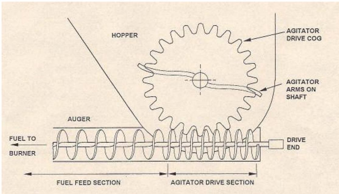
Fig. 32(c): The fuel feed system [23]
