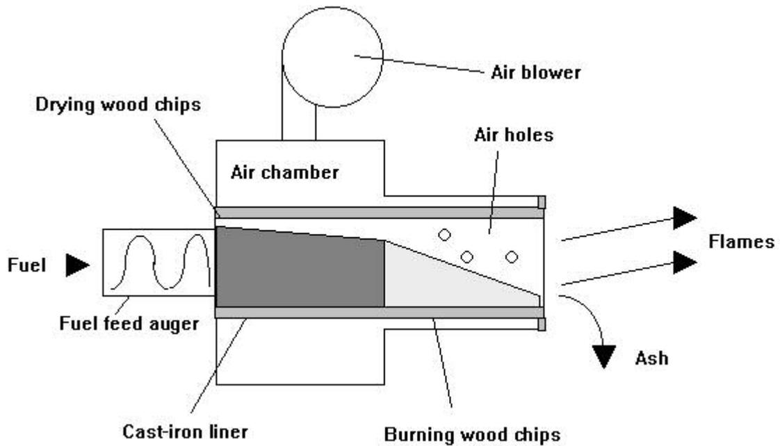
Fig. 35: The Stoker-burner layout [18]
