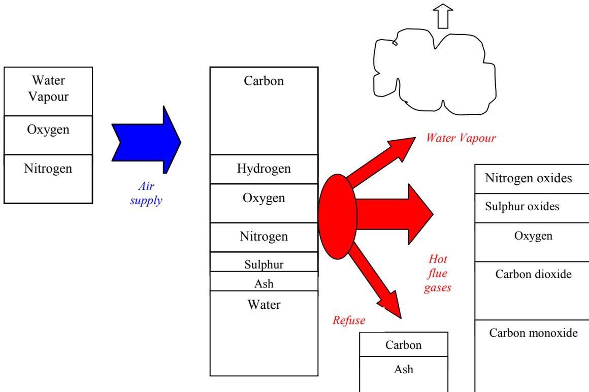
Fig.22: Simplified model of combustion balance [21]
