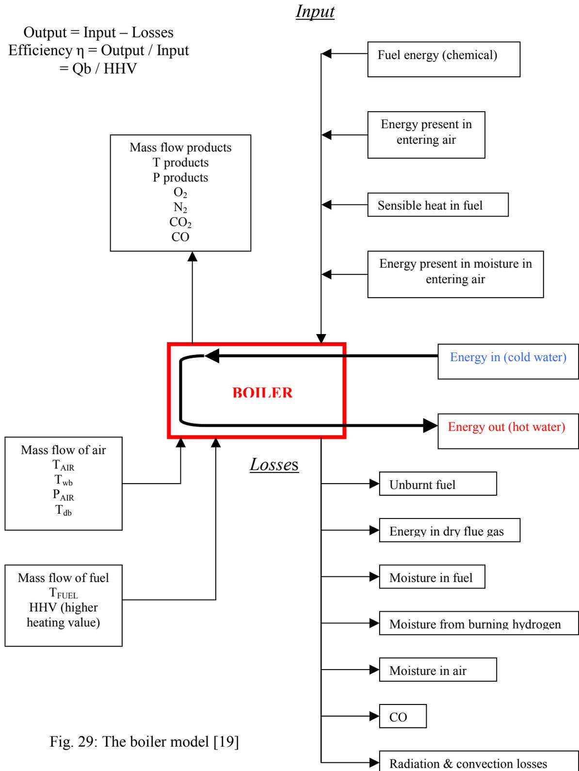
Fig. 29: The boiler model [19]
