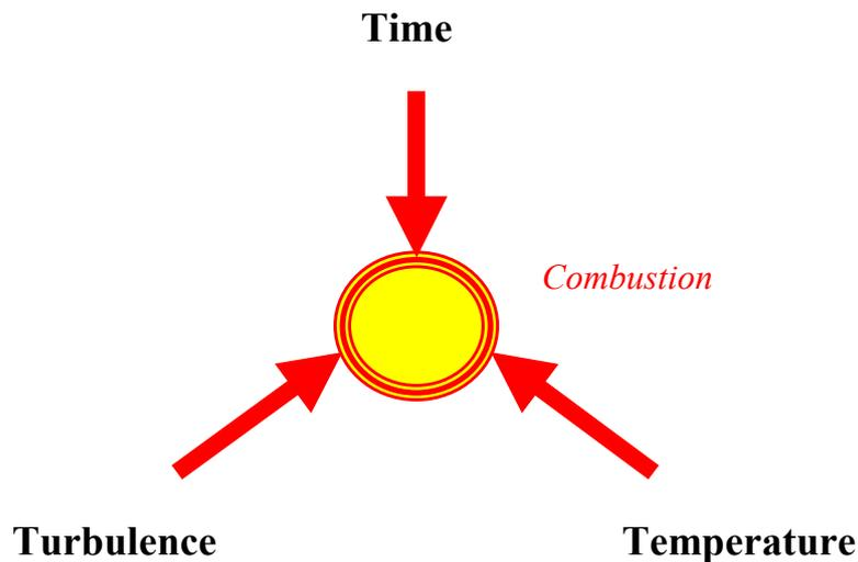
Fig. 19: The Three ‘T’s’ of Combustion [19]
