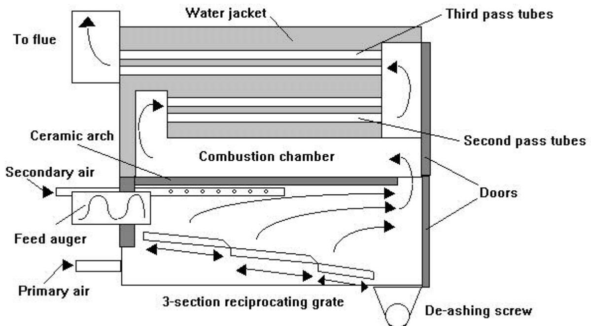
Fig. 37: The Inclined Grate design [18]
