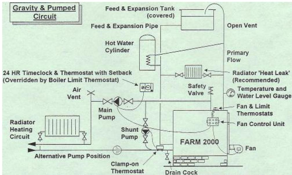
Fig. 38: Woodchip boiler ('Farm 2000' model) connected into a Gravity & Pumped Circuit [23]
