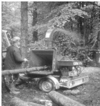
Fig. 27: A typical portable chipping machine [18]
