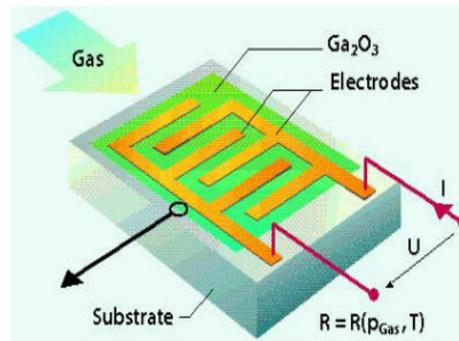
**Figure 4.3** *A typical gas sensor*
