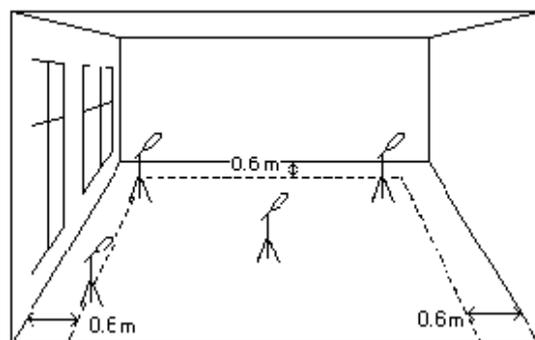
**Figure 4.2** *Example of Sensors arrangement*
