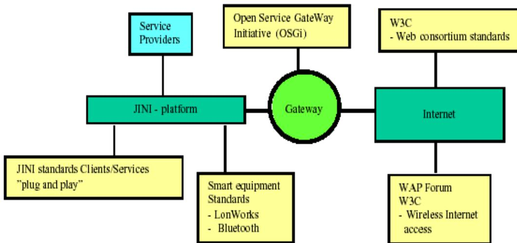
**Figure A1.1** *The most important standardization efforts and technologies supporting the networked smart house*
