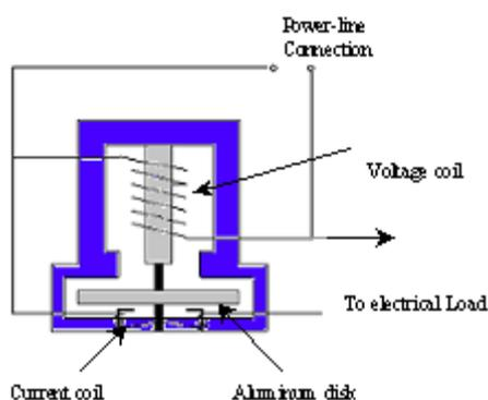
**Figure 4.1** KWh meter
