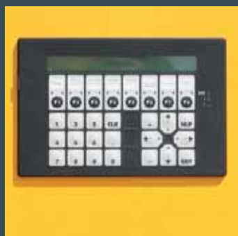
Control panel with plain language display (like PyroControl)
