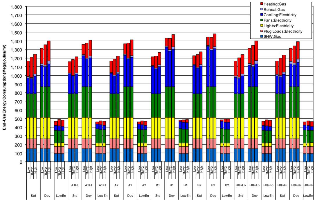
**Figure D.2-1. Annual Source Energy End-Use Consumption in Washington, D.C., USA, for Standard, Developing, and Low-Energy Buildings Using Typical Year, Climate Change Scenarios, and Heat Island Cases**
