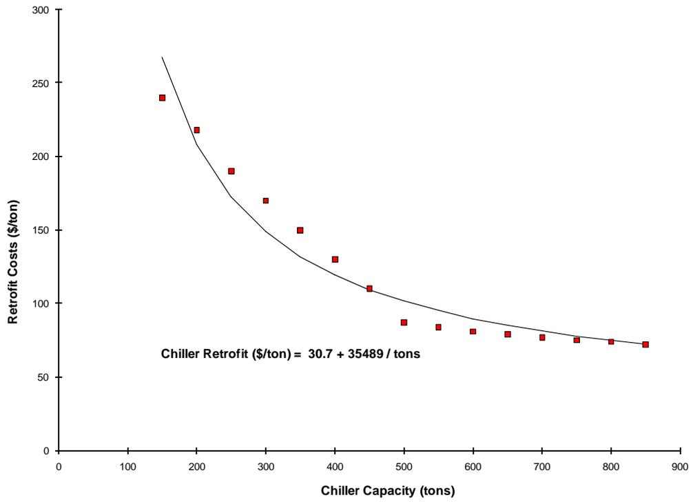
Figure C-3. Non-CFC Retrofit of Existing Chiller<sup>4,5</sup>
