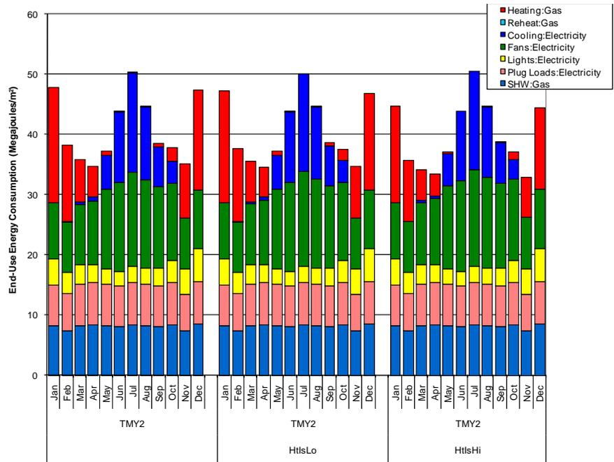
**Figure D.2-13. Monthly Source Energy End-Use Consumption in Washington, D.C., USA, for Low-Energy Building and Heat Island Cases**
