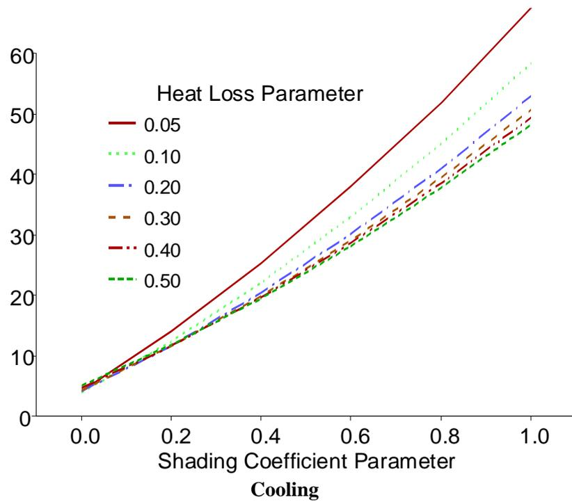
**Figure 3-3. Coil Loads for the South Orientation<sup>4</sup>**
