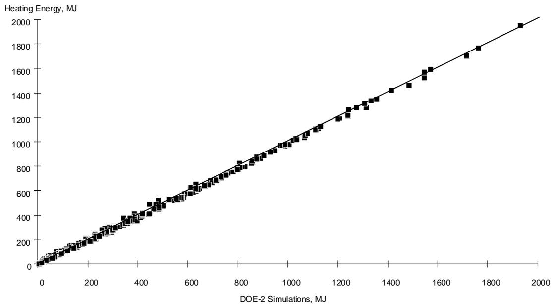
**Figure 4-3. Predicted Heating Energy for Correlation v. DOE-2.1E Simulations for East Orientation in Ottawa**
