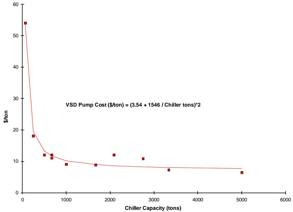
Figure C-5. Variable Speed Pump Drives<sup>7,8</sup>
