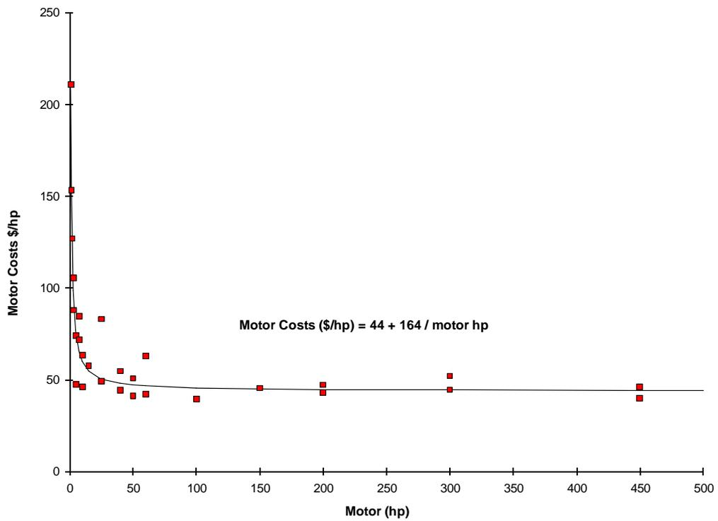
**Figure C-2. High-Efficiency Fan Motors<sup>3</sup>**
