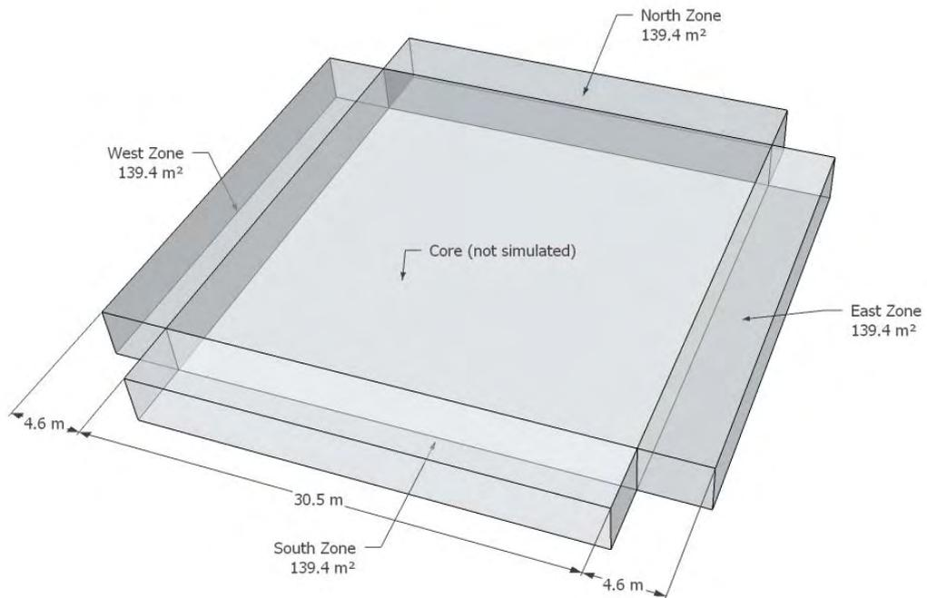
**Figure 3-5. Diagram of Four-Zone DOE-2 Building Model**
