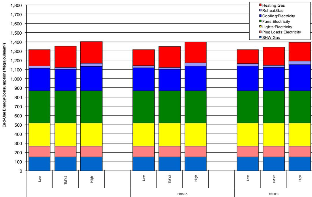
**Figure D.2-6. Annual Source Energy End-Use Consumption in Washington, D.C., USA, for Developing Building and Heat Island Cases**
