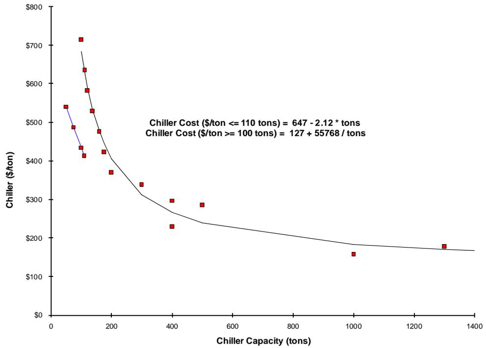
Figure C-4. New High-Efficiency Non-CFC Centrifugal Chiller<sup>6</sup>
