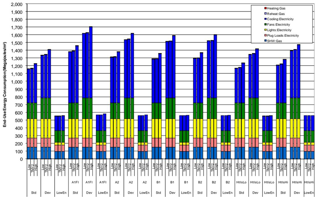
**Figure D.1-1. Annual Source Energy End-Use Consumption in San Juan, Puerto Rico, for Standard, Developing, and Low-Energy Buildings Using Typical Year, Climate Change Scenarios, and Heat Island Cases**
