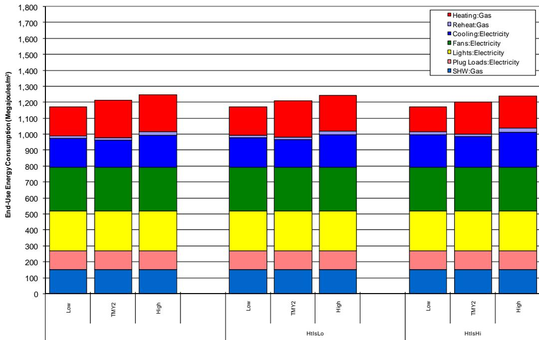
**Figure D.2-5. Annual Source Energy End-Use Consumption in Washington, D.C., USA, for Standard Building and Heat Island Cases**
