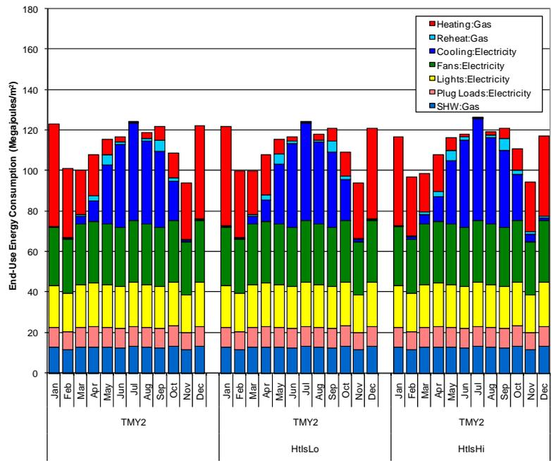
**Figure D.2-12. Monthly Source Energy End-Use Consumption in Washington, D.C., USA, for Developing Building and Heat Island Cases**
