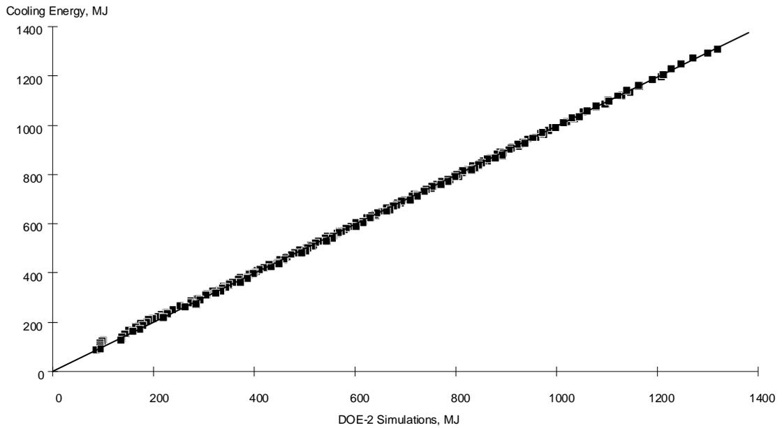
**Figure 4-2. Predicted Cooling Energy for Correlation v. DOE-2.1E Simulations for East Orientation in Ottawa**
