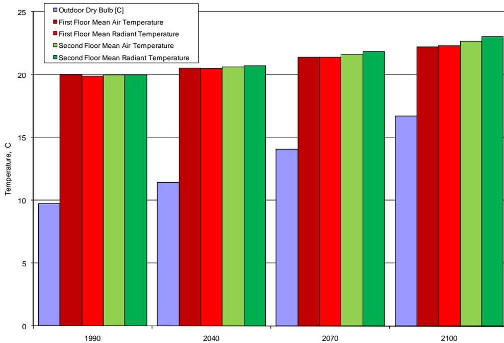
**Figure 2-1. Annual Average Outdoor Temperature and Predicted Indoor Mean Air and Radiant Temperature, °C, by Zone in Chicago, Illinois, USA (Crawley 2003)**
