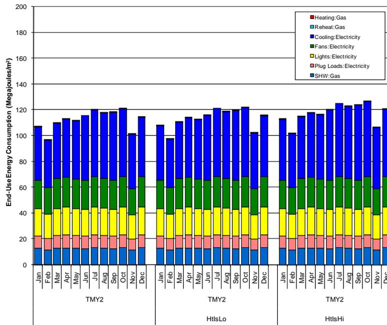
**Figure D.1-12. Monthly Source Energy End-Use Consumption in San Juan, Puerto Rico, for Developing Building and Heat Island Cases**
