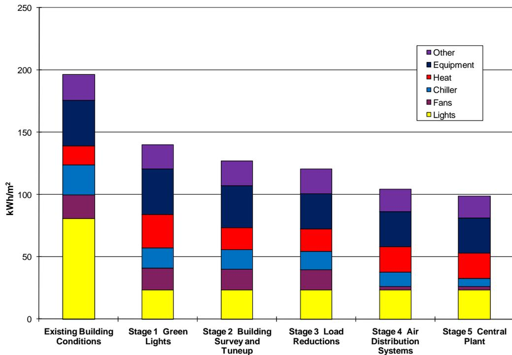
**Figure C-12. Energy End-Use by Stage for High-Rise Office Building with Electric Heat in Washington, D.C.**
