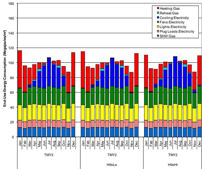
**Figure D.2-11. Monthly Source Energy End-Use Consumption in Washington, D.C., USA, for Standard Building and Heat Island Cases**
