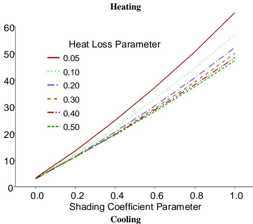
**Figure 3-4. Coil Loads for the West Orientation<sup>5</sup>**
