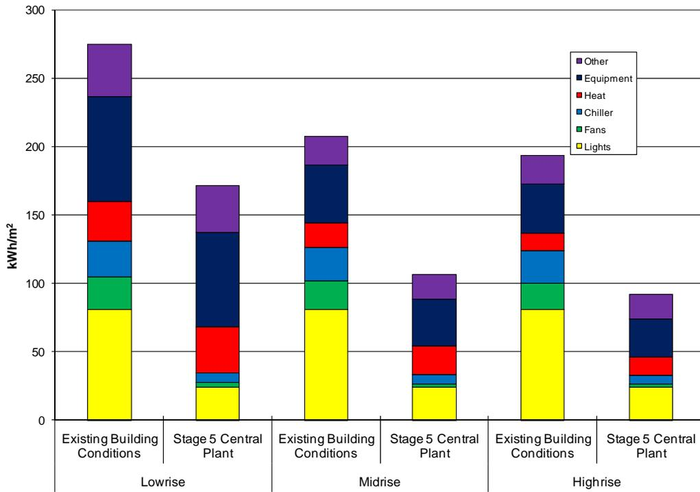
**Figure C-13. Comparison of Energy End-Uses for Existing Buildings and ENERGY STAR Buildings Upgrade for the Three Office Building Sizes in Washington, D.C.**
