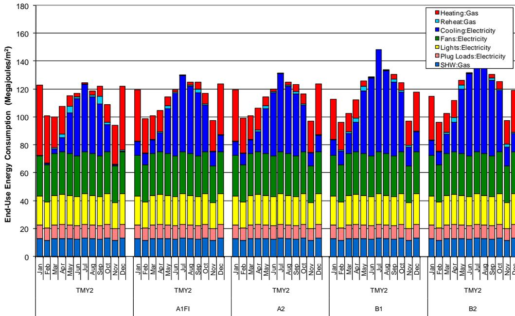
**Figure D.2-9. Monthly Source Energy End-Use Consumption in Washington, D.C., USA, for Developing Building and Climate Change Scenarios**
