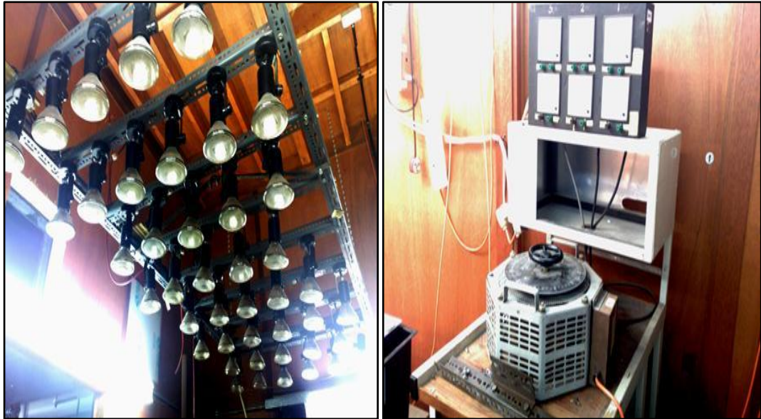
Figure 5-3: Solar simulator chamber parts: mercury vapour bulbs and potentiometer.
