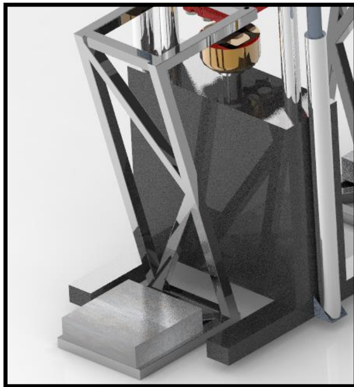
Figure 59: Mounting Frame Showing Supporting and Concrete Counter Weight Blocks
