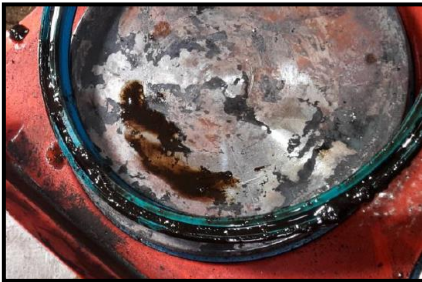
Figure 9: Oil Contamination Seen During Component Strip Down
