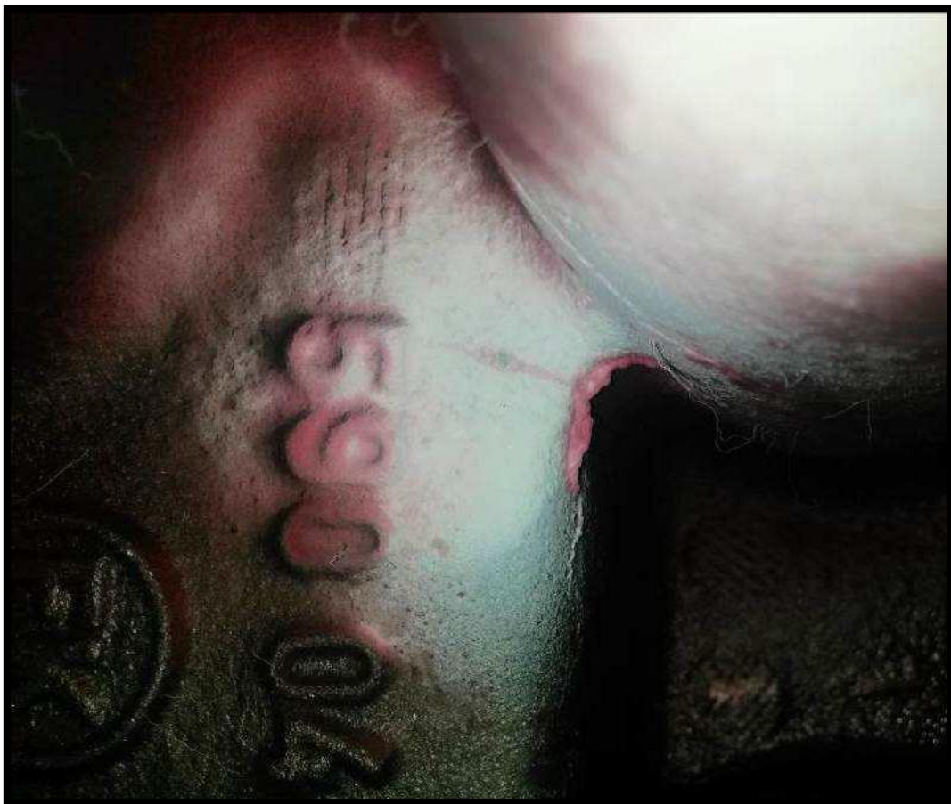
Figure 4: Dye Penetration On Shallowest Section Within The Hollow Section Between Clearance Holes
