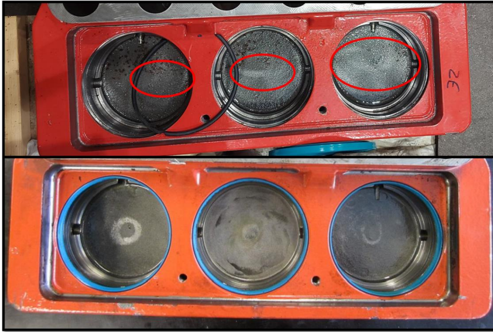
Figure 8: Top - New Caliper with Cast Skin, Cast Defects in Red; Bottom - Used Caliper with Cast Skin Damage
