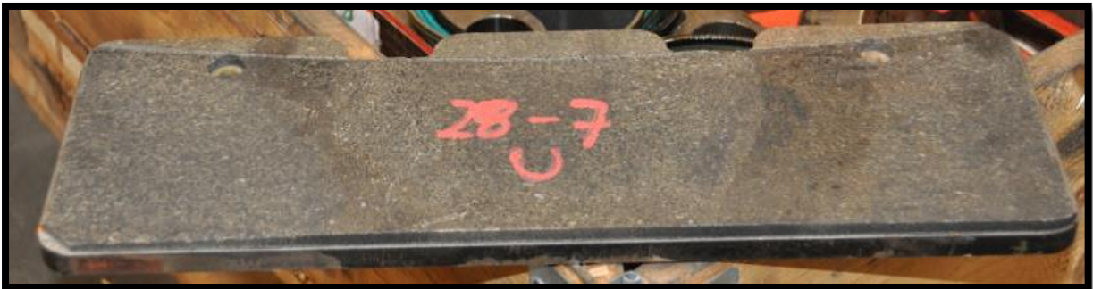
Figure 10: Brake Pad Showing Uneven Wear
