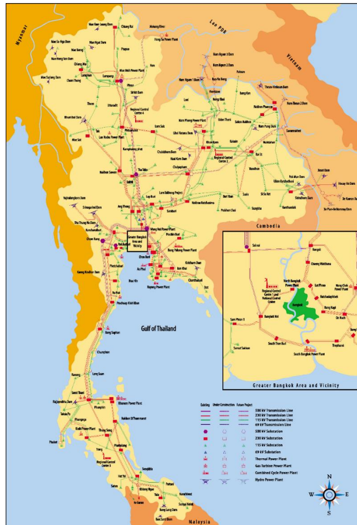
Figure 5 National Grid Network in Thailand (GENI, 2016)
