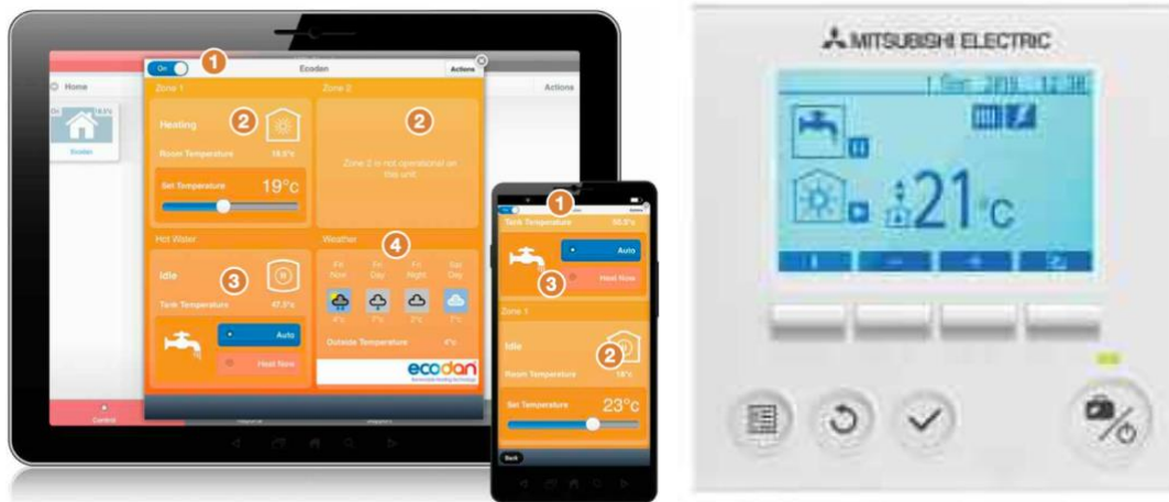
Figure 2: MELCloud User Interface & Wall controller Unit for Ecodan- FTC-5 (8)
