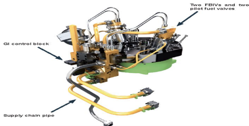
Figure 27: Fuel injectors and control block are installed in the cylinder lid Man 2019 [68].
