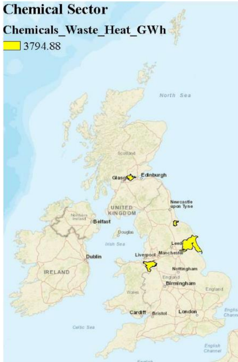
Figure 46 Distribution of estimated waste heat from the chemical industry [28].
