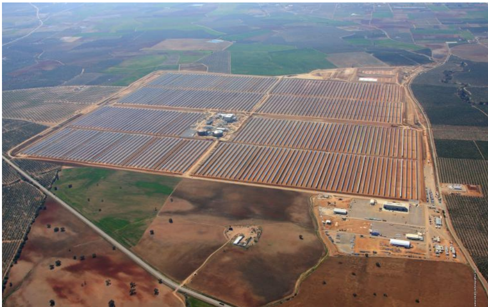
Figure 7 La Africana parabolic trough CSP plant in Spain (source: https://www.energy.sener/projects/la-africana-parabolic-trough-plant-50mwe )
