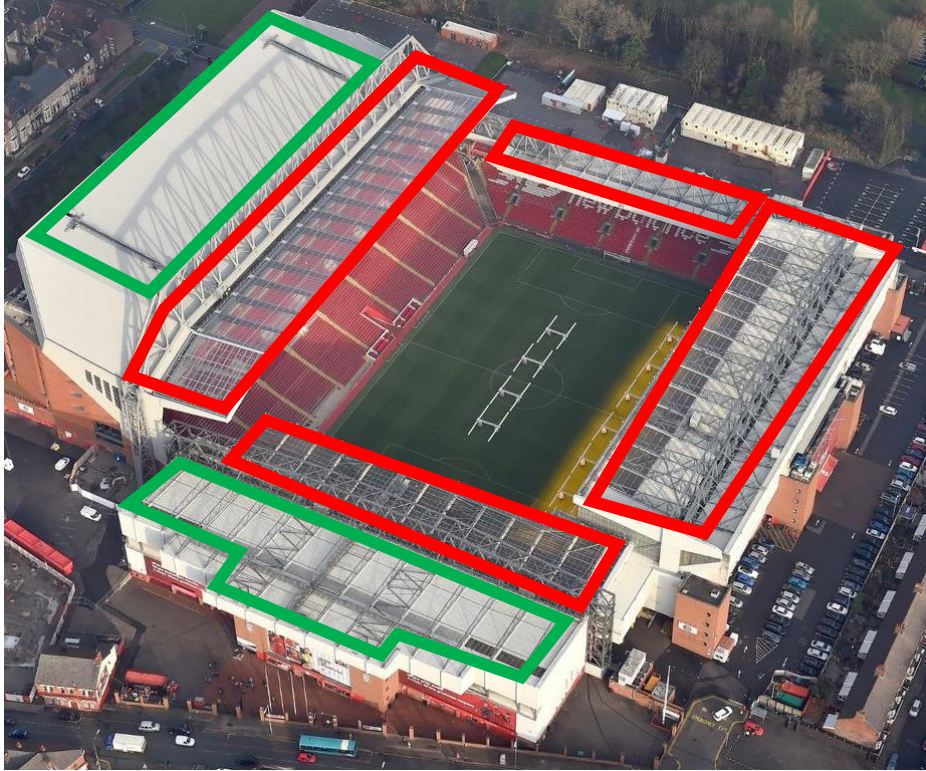
Figure 28: Aerial view of Anfield, home ground of Liverpool FC, with areas of the stadium roof suitable to hold PV panels shown in green and unsuitable areas shown in red.
