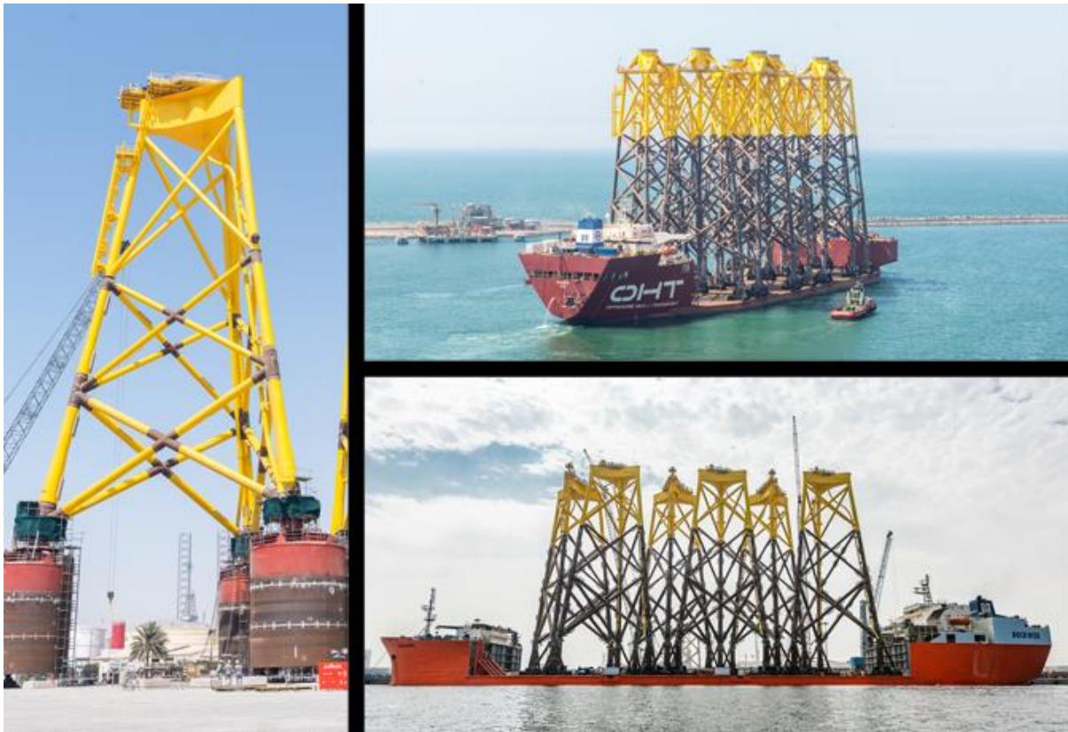
Figure 1: Wind Farm Jacket Foundations being transported by the Heavy Lift Vessel OHT Hawk (top right) from the Lamprell port based in the UAE heading to the North Sea. Image sourced from (Lamprell, 2021).
