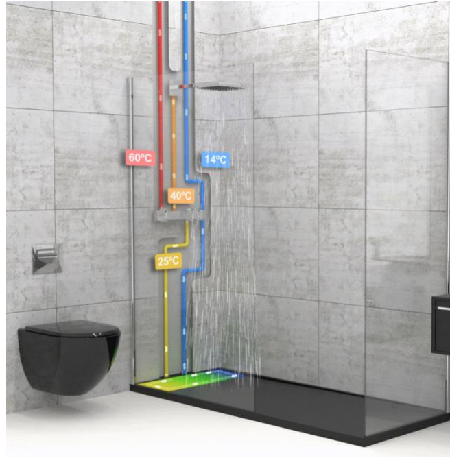
Figure 14: Diagram of the Cerian Passive Shower
