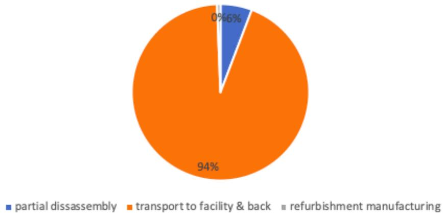
Figure 32- Breakdown of Carbon emission contributions by process within refurbishment process.
