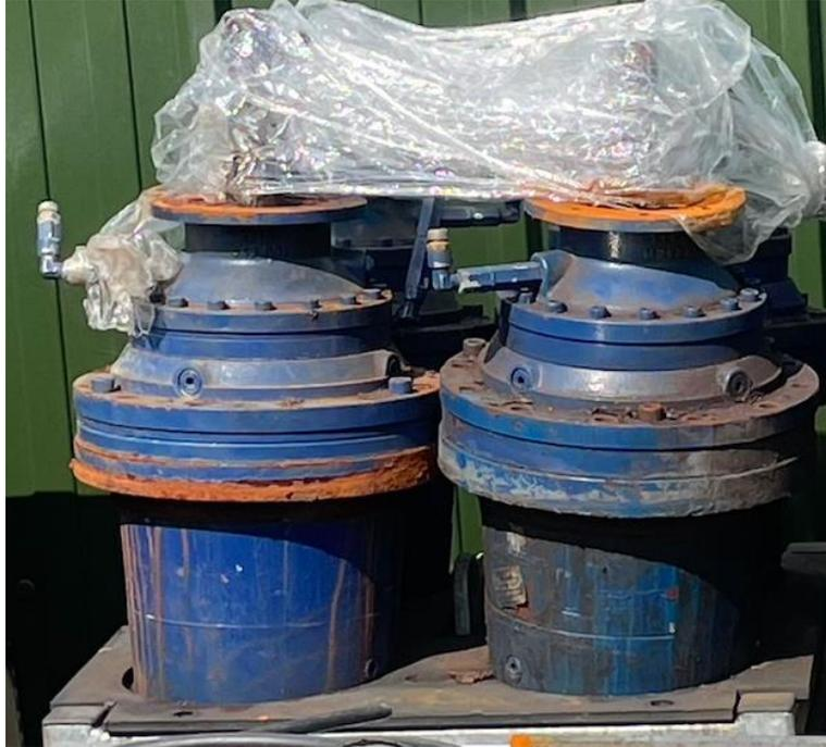
Figure 18- Two Yaw Gears upon delivery to RPL Refurbishment factory, prior to any work. Photographed by the author at the refurbishment factory in Lochgilphead on 04/08/2021.
