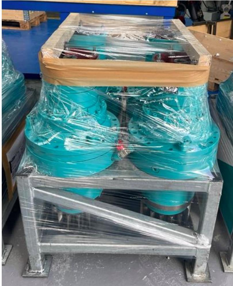
*Figure 20- Four fully refurbished and painted Yaw Gears, packaged to return to turbine customer site. Photographed by the author at the refurbishment factory in Lochgilphead on 04/08/2021.*
