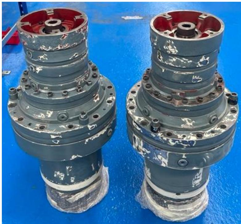
Figure 19- Two Yaw Gears after refurbishment and sanding.. Photographed by the author at the refurbishment factory in Lochgilphead on 04/08/2021.
