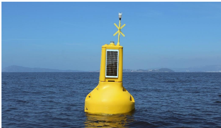
Figure 15: Metocean buoy installed in Saint-Nazaire [58]
