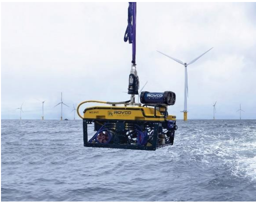
Figure 9: ROV used to take subsea pictures of offshore wind foundation [53]
