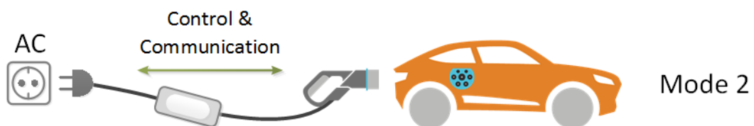
Figure 2.5 : EV charging Mode 2 (Source: Deltrix Chargers Company)
