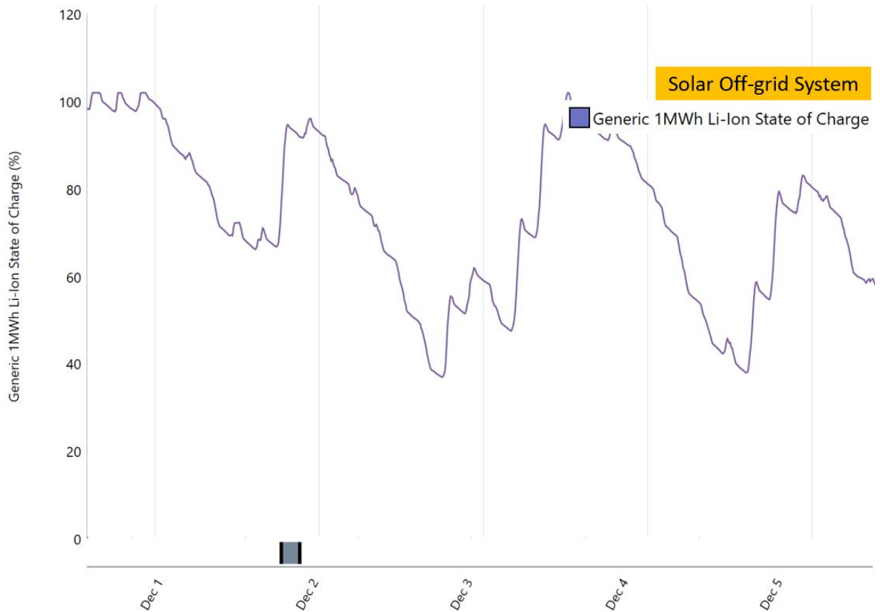
Figure 6.23 : The state of charge (SOC) of a solar off-grid system (Case 1 - on a cloudy day)
