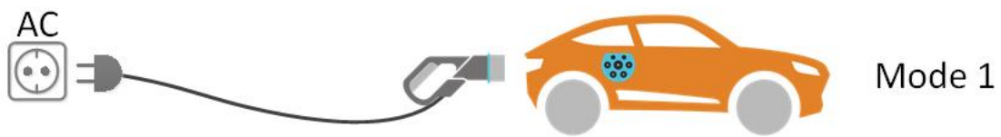
Figure 2.4 : EV charging Mode 1 (Source: Deltrix Chargers Company)
