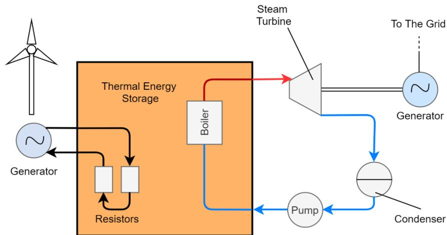
Figure 6 - Simplified WTES system using electric resistors to heat the storage medium
