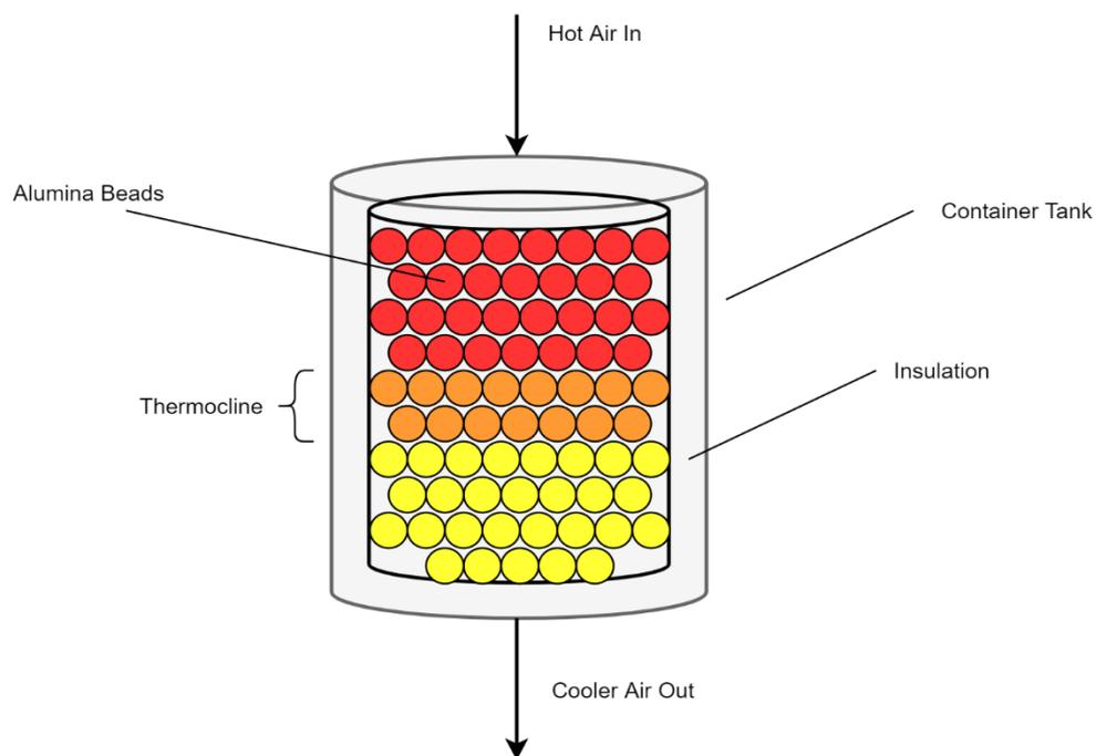
*Figure 9 – General schematic of an alumina beads packed bed SHS system*
