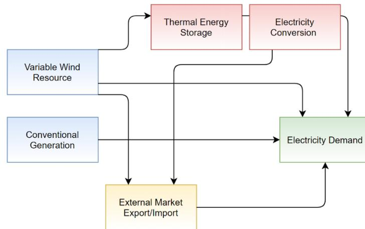
*Figure 11 - Schematic of desired simplified EnergyPLAN model*
