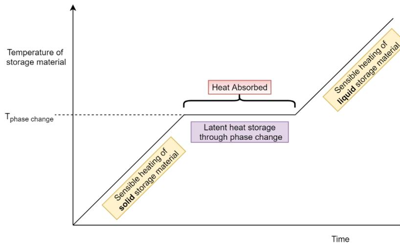
*Figure 4 - Simple graph to show how energy is stored as both sensible and latent heat in a PCM*
