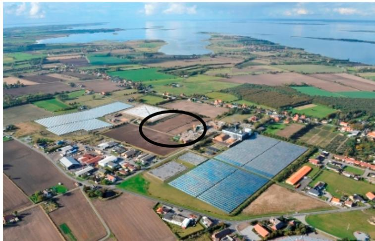
*Figure 3 - Marstal Solar Thermal District Heating Scheme, water container basin circled*
