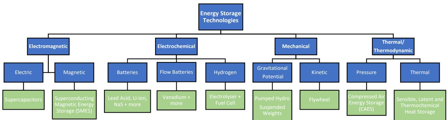
Figure 1 – Tree diagram showing the different categories of energy storage methods
