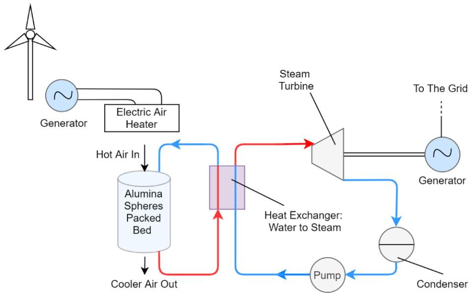
Figure 10 - Schematic of alumina beads packed bed SHS system within a WTES system
