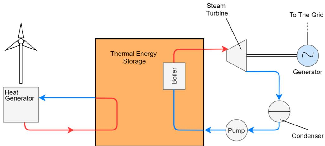
*Figure 7 - Simplified WTES system using a heat generator to heat the TES medium*
