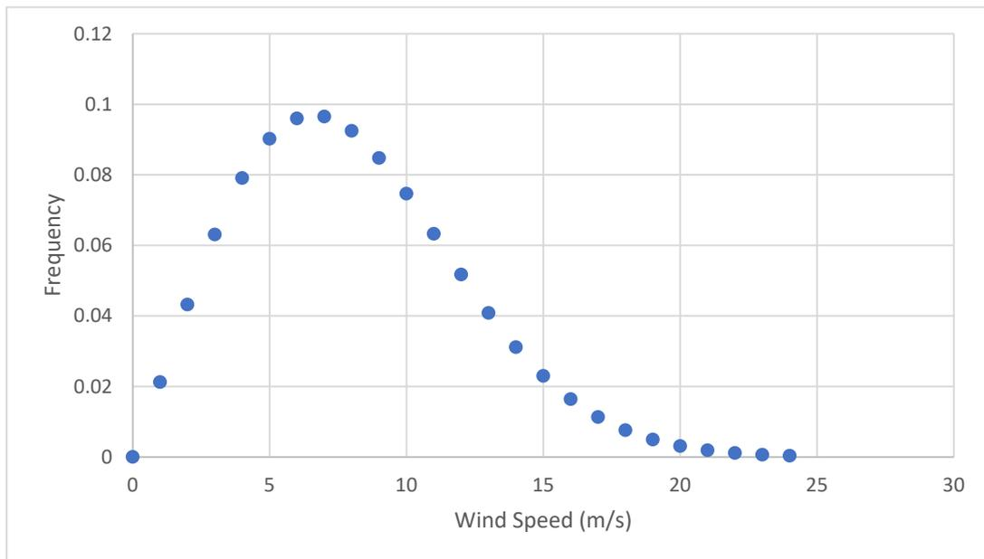
Figure 15 - Weibull distribution of wind speed at chosen area at height of 65m
