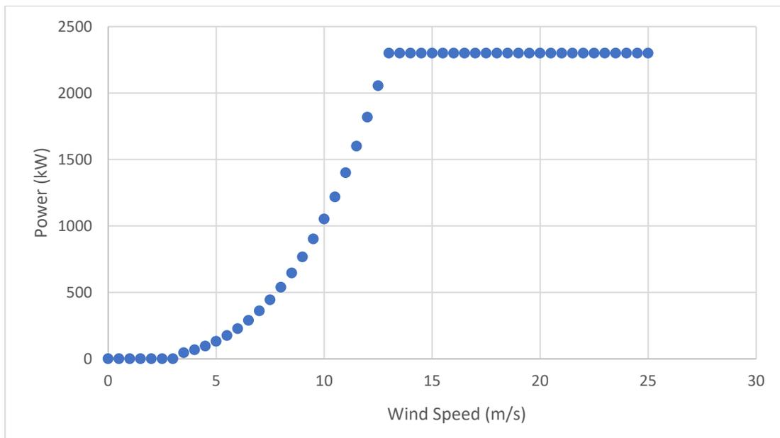
Figure 14 - Power curve of the Siemens SWT-2.3 turbine
