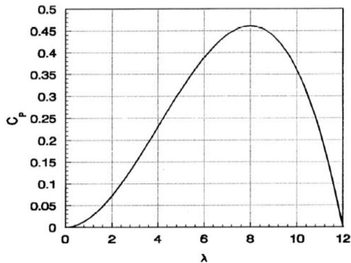
*Figure 8 - Generic  $C_p$ - $\lambda$  used to estimate the power coefficient at different wind speeds*
