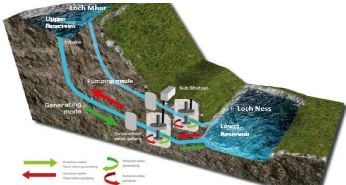
Figure 7 - Schematic representation of Foyers Pumped Hydro Scheme
