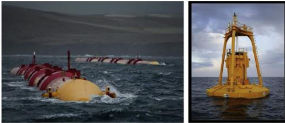
Figure VI: Illustrations of Pelamis II and PowerBuoy Oscillating Bodies, (Pérez-Collazo, Greaves and Iglesias, 2014).
