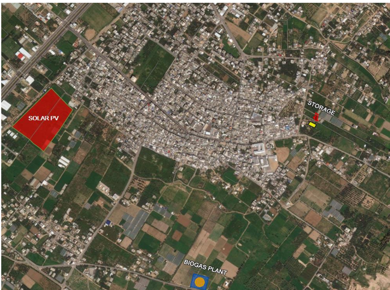
Figure 13- Potential layout of RES components for 70-75% RES penetration, in relation to Maghazi. ArcMap software.
