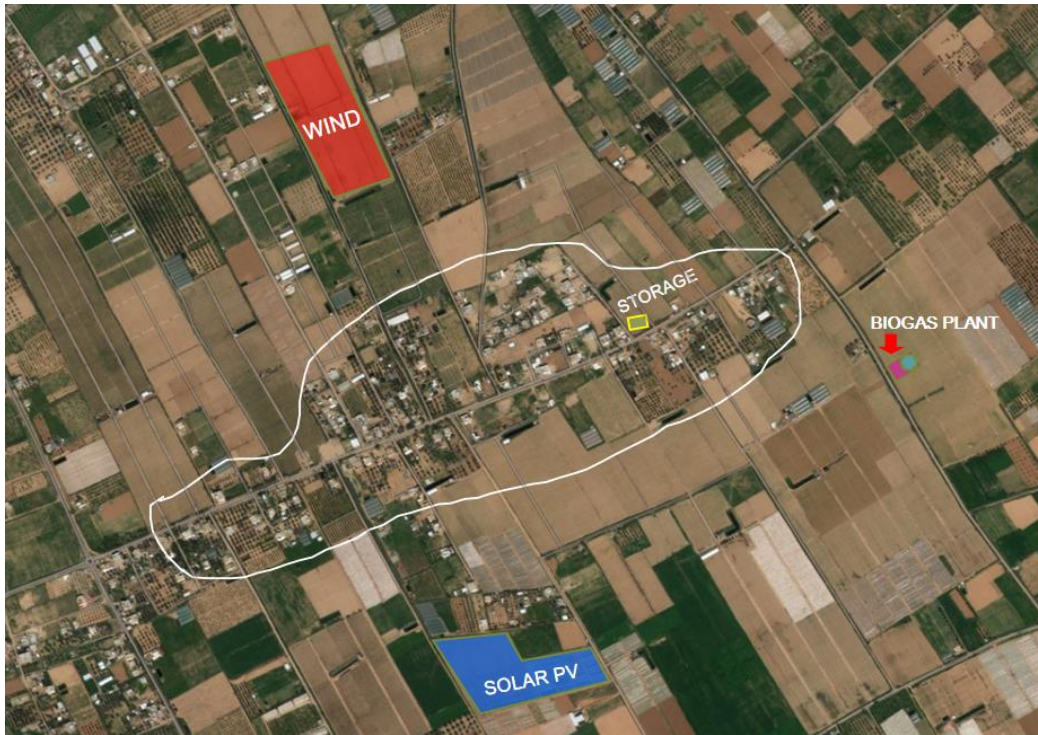
Figure 12- Potential layout of RES off-grid microgrid components in relation to Al-Fukkhari (circled in white). ArcMap software.
