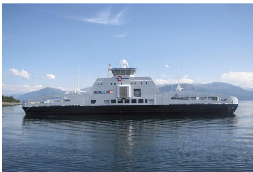
Figure 8: MS Ampere, world's first all-electric ship (NCE Maritime CleanTech, 2015)
