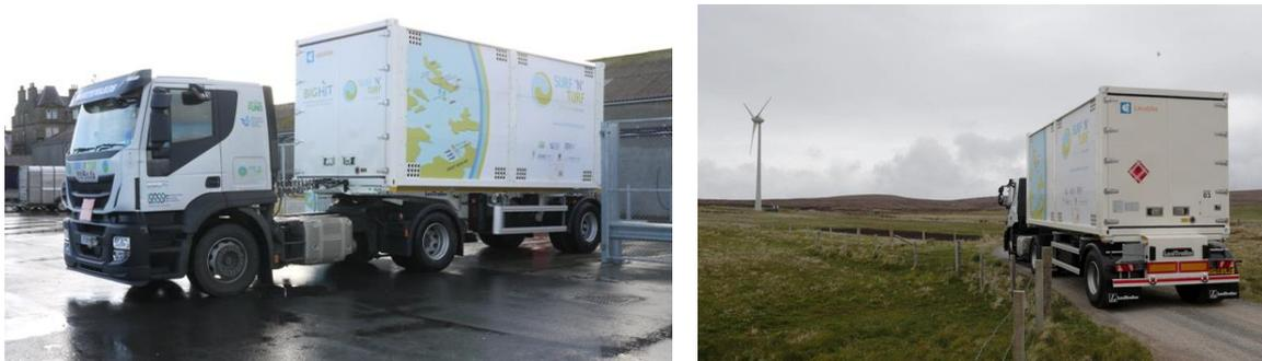
*Figure 35 Specialised Lightweight Trailer for Transportation of Hydrogen*
