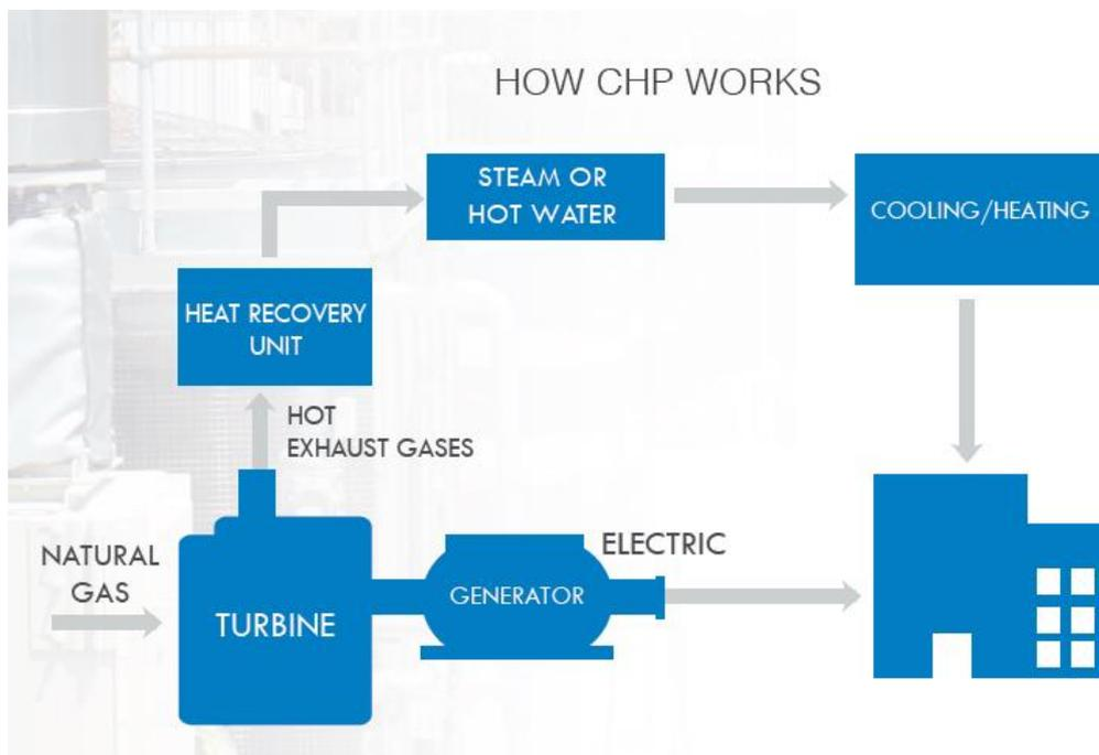
*Figure 5 Main Components of a Combined Heat & Power system (PGW, 2019)*
