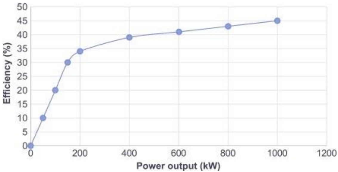
Figure 9 Efficiency of a Diesel Generator against Power Output (Adefarati et al, 2019)
