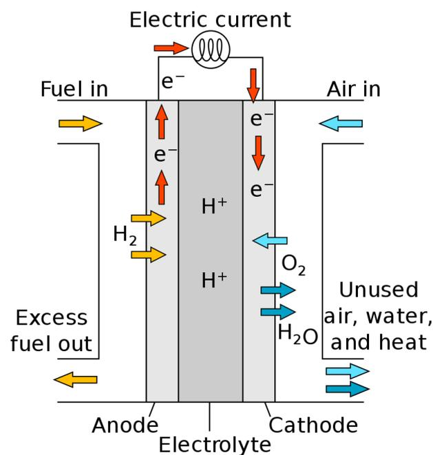
Figure 4 Diagram of a Hydrogen Fuel Cell
