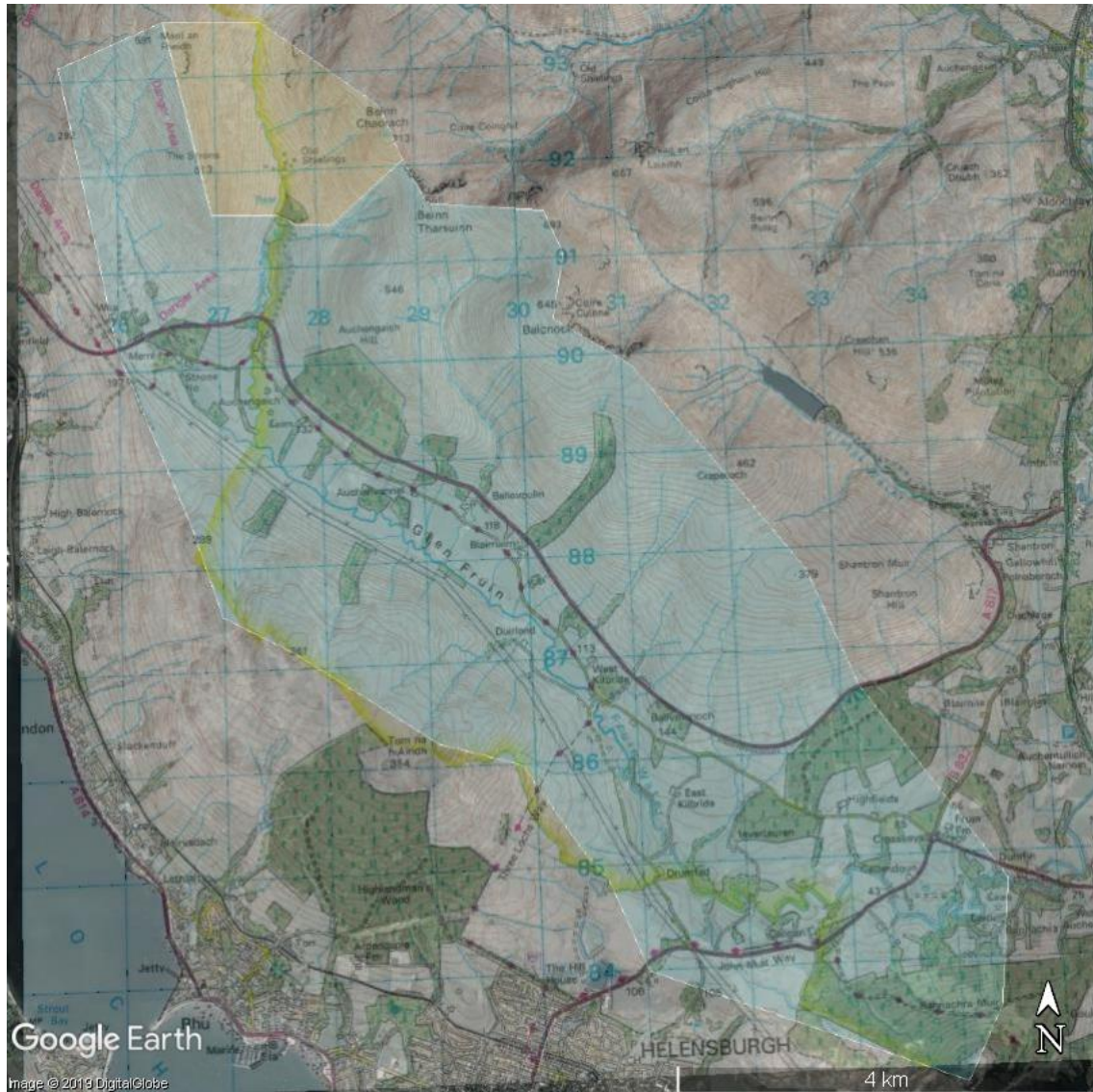
Figure 9: Case study catchment area plotted in Google Earth with OS mapping overlay. (The yellow shaded area represents the catchment area of the reservoir, the blue shaded area represents the catchment area of Fruin Water utilised at Dumfin Sawmill.)
