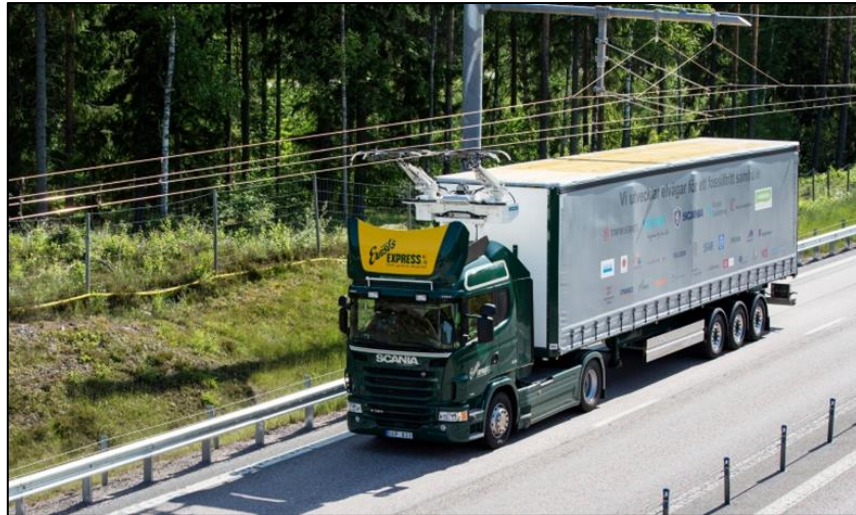
Figure 5: Electrified eHighway for trucks developed by Siemens in Germany
