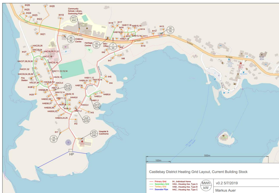
Figure 29 Proposed District Heating Grid with Labels Showing Current Energy Demand and Peak Loads.
