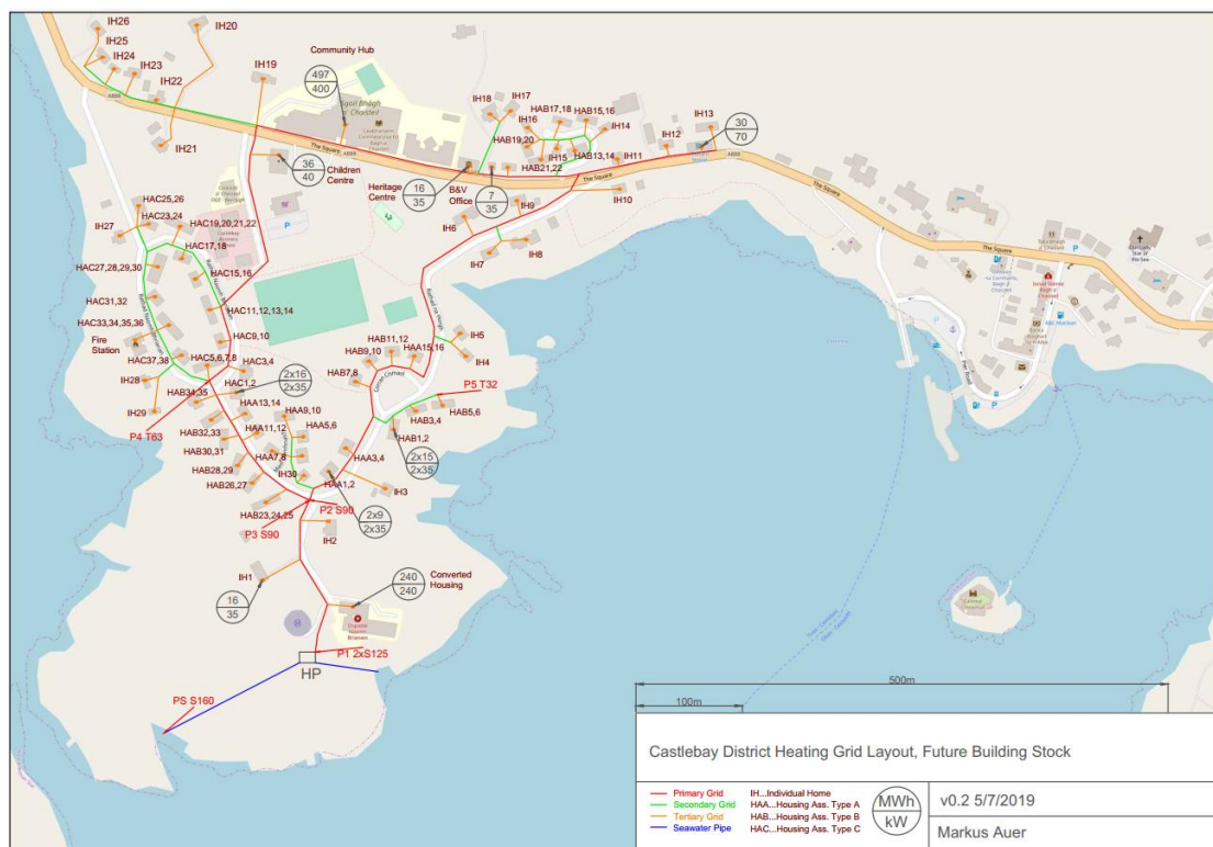
Figure 32 Proposed District Heating Grid with Future Energy Demands, Peak Loads and Pipe Dimensioning.
