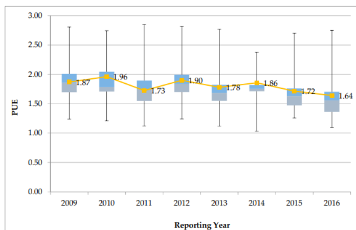
Figure 10 Average PUE per Reporting year, Source: Trends in European Data Centre Energy Consumption (Averingou et al 2017)
