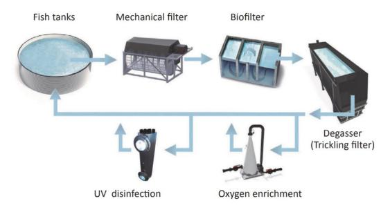
Figure 46: RAS recirculation key components (FAO, 2015)
