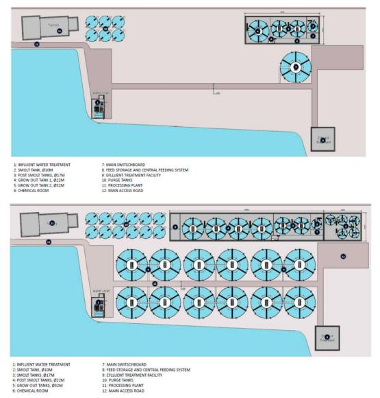
*Figure 49: Example of modular design for a recirculating aquaculture system plant* (*Niri.com, 2018*)
