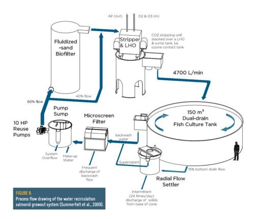
Figure 2: Diagram of a recirculating aquaculture system (RAS) (Summerfelt et al., 2013)
