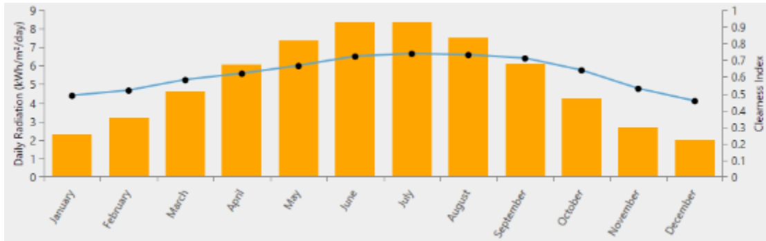
Figure 38: Global Horizontal Irradiance in kWh/m 2 /day and Clearness Index in %, for Koufonisi.
