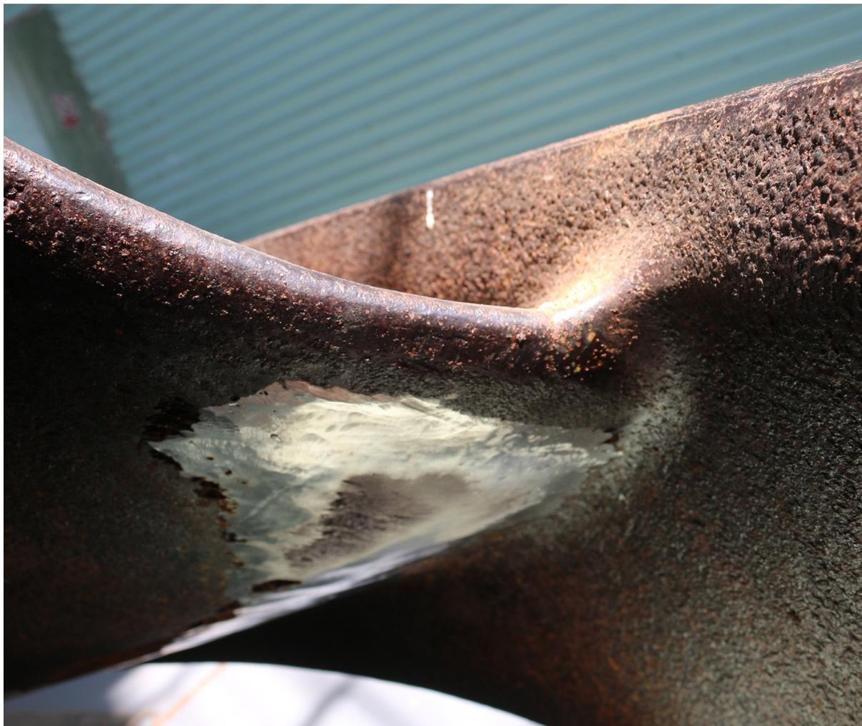
*Figure 15: Francis Turbine Cavitation Repair at Tongland*
