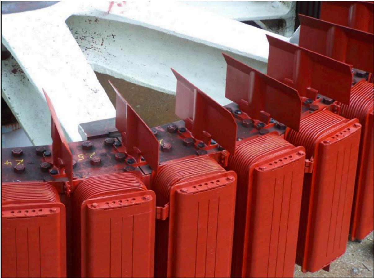
*Figure 8: Typical Field Pole (Mesa Associates Inc. and Oak Ridge National Laboratory, 2011a)*
